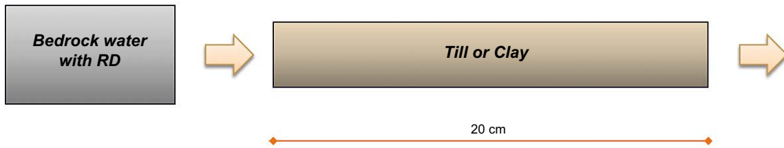
Figure C-1. Conceptual model. The domain is composed by till or clay with waters initially in equilibrium with those materials.
