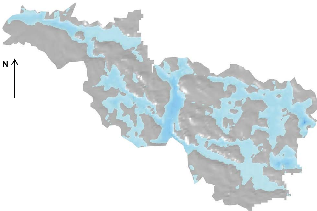
Figure 4-3. Areas with modelled groundwater discharge at the ground surface of the regolith (light blue).
