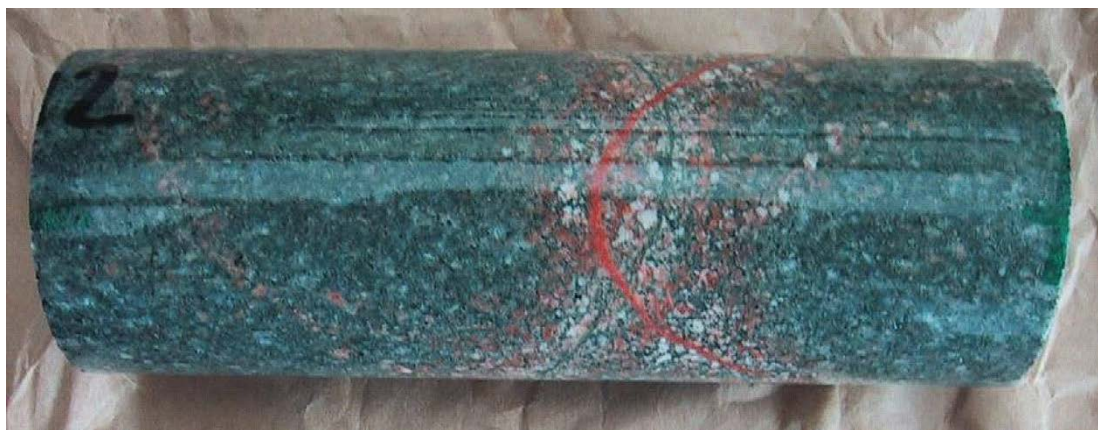
Figure 1-12. Epidote sealed fracture cut by a sealed fracture filled with hematite stained adularia. KFM05A 692.00–692.15 m. The diameter of the drill core is c 5 cm.
