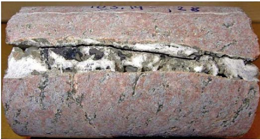
Figure 1-14. Partly open fracture with a mixture of euhedral calcite, small euhedral quartz crystals, asphaltite and small pyrite crystals. The diameter of the drill core is c 5 cm.
