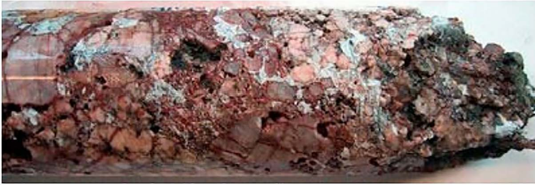
Figure 6-29. Episyenite where the quartz has been dissolved. The voids have later been filled with calcite (white in figure). The diameter of the drill core is c 5 cm. KFM08A 410.60–411.04 m.
