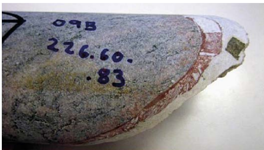
Figure 9-15. Open fractures of borehole KFM09B at Forsmark, at borehole lengths 226 m, with coating of laumontite, calcite, pyrite, and quartz (figure modified from Löfgren and Sidborn (2016)).
