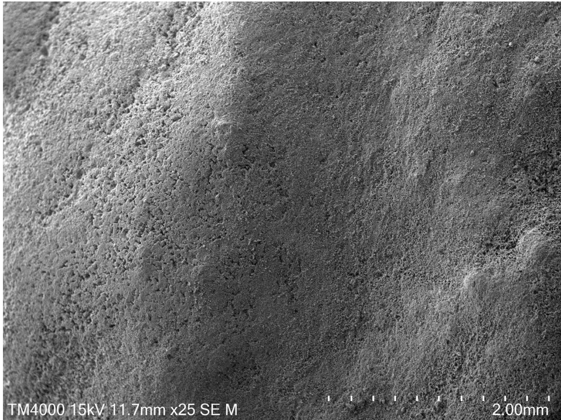
Figure 3-2. Surface of black mineralization visualized by SEM.
