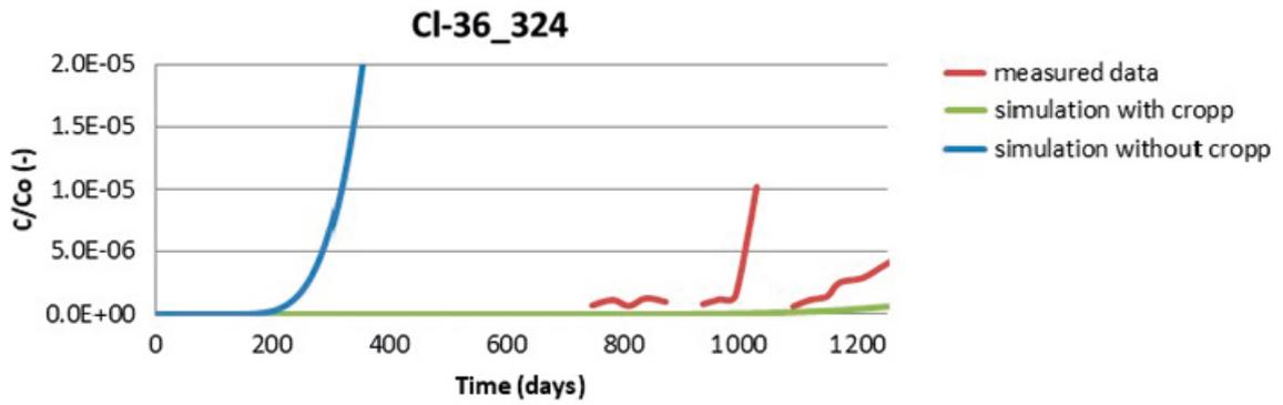
Figure 6-40. Agreement between the measured and model results in the monitoring borehole.
