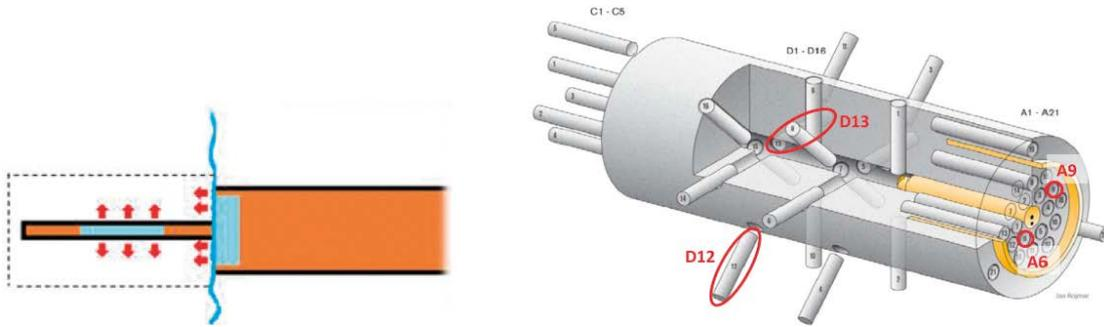
**Figure 4-1.** Configuration of the LTDE-SD experiment: Left: boreholes intersecting the fracture, placement of the radionuclide solution, direction of migration and position of the drill block. Right: configuration of core drilling sampling and selection of the profile for Task 9B-1 (below). In yellow, the insulation separating the 177 mm core area that was in contact with the radionuclides while the exterior should theoretically be unaffected. (Löfgren and Nilsson 2020).
