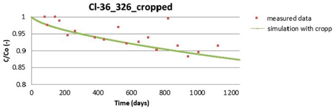
**Figure 6-39.** Agreement between the measured and model results for the cropped data, development of activity in the injection borehole.
