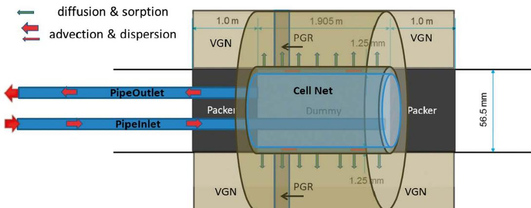
**Figure 3-4.** Schematic representation of the conceptual model of the WPDE1-2 experiments in GoldSim – using a cell network for the rock and slot and two Pipe pathway elements (PipeInlet and PipeOutlet) for the inlet and outlet pipes.
