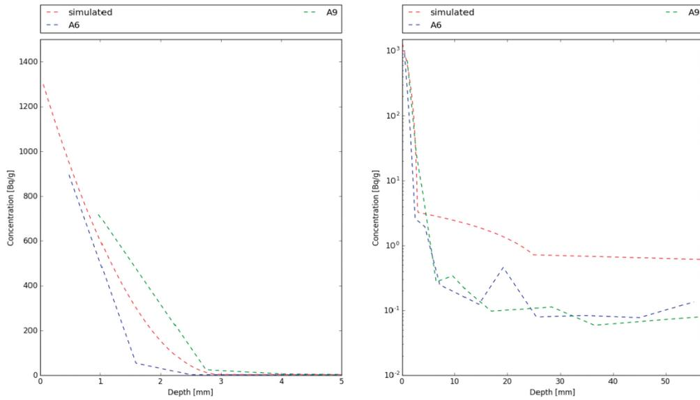
**Figure 4-17.** LTDE-SD – concentration profiles in the rock in a linear (left) and logarithmic (right) scale – Ba-133.
