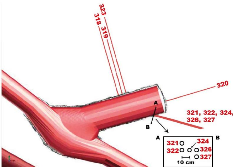
**Figure 6-1.** Borehole assembly at and around the TDE experiment – the injection borehole is number 326 and the monitoring boreholes are 324 and 327 (taken from Andersson et al. 2020).
