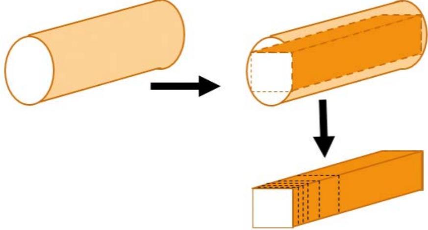
**Figure 4-3.** Diagram of the preparation of the analysed samples from the drill core (taken from Löfgren and Nilsson 2020).
