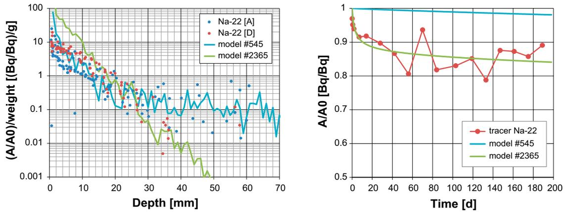
Figure 5-10. Na-22 – comparison of measured data and model results – cross-sections of the sample and model domain on the left, course of the activity in the source reservoir on the right.
