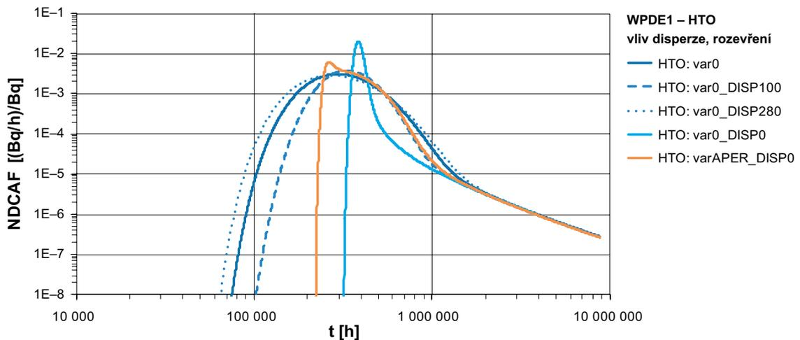
Figure 3-26. Effect of dispersion and aperture of the fracture on the course of the breakthrough curve of HTO.
