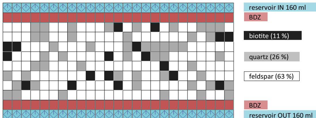
**Figure 5-7.** Laboratory diffusion experiment LTDIII – concept of rock matrix without significant micro-fractures with division of the domain according to the percentage of minerals (Aare granite).
