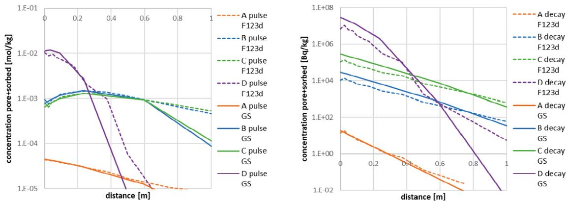
Figure 7-12. Comparison of solution 9D-1 cross-sectional profiles of two models (Flow123d and GoldSim – GS) for all of the tracer., Pulse inflow without decay (variant a); continuous inflow with decay (variant b).
