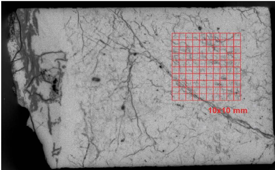
*Figure 5-1. Microstructure image obtained by the C-14-PMMA method – sample LTDE-SD1 (DD18, 2017).*
