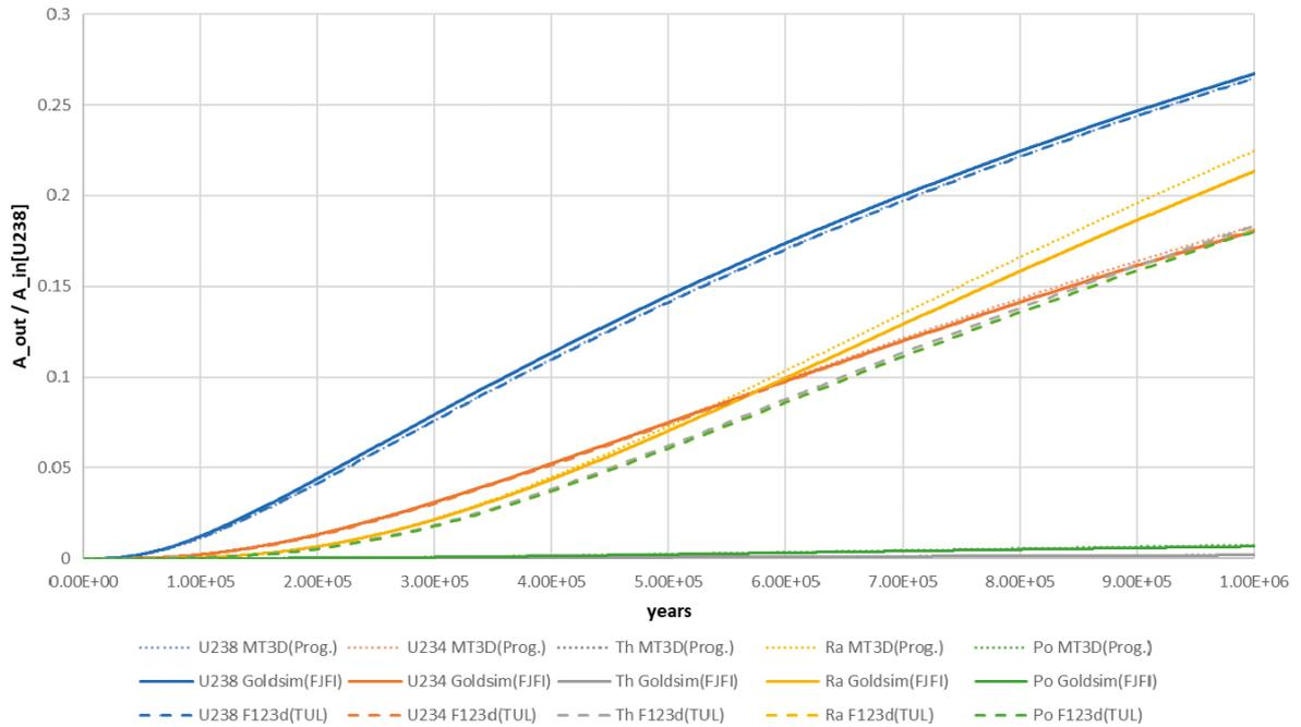
**Figure 7-14.** Comparison of solution 9D-2 breakthrough curves for five radionuclides in the decay series (*Pb* is not plotted, it is graphically indistinguishable from *Po*) – calculations by three different software programs.
