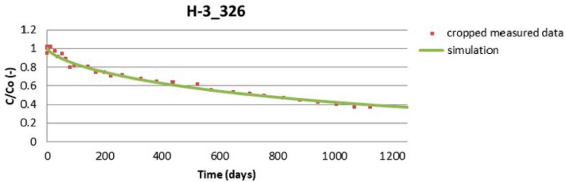
Figure 6-33. Development of activity in the injection borehole.
