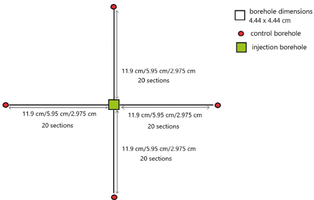
**Figure 6-5.** Representation of uniform discretisation for sorbing radionuclides, size and discretisation of the model area was made in three variants.
