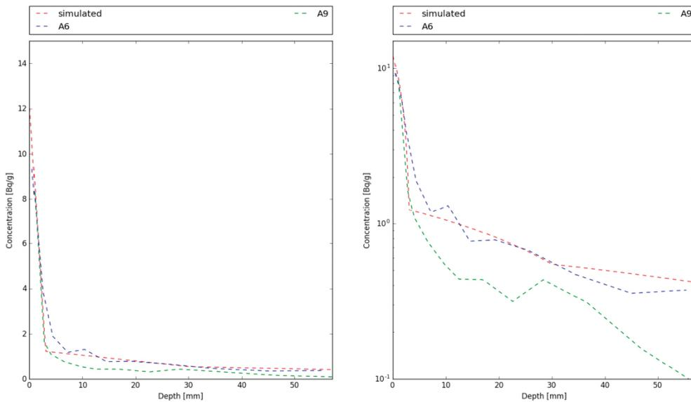
**Figure 4-14. LTDE-SD – concentration profiles in the rock in a linear (left) and logarithmic (right) scale – Cl-36.**
