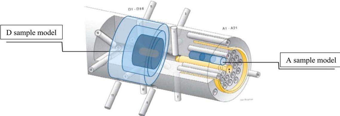
**Figure 4-2.** Configuration of the LTDE-SD experiment showing the geometric significance of the models for two sample types (axisymmetric for D and one-dimensional for A).
