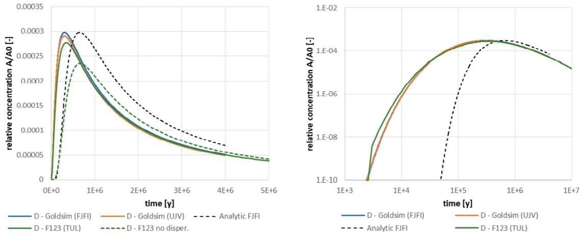
Figure 7-10. Comparison of solution 9D-1-a breakthrough curves in two types of axis scales for tracer D (three models and variants without dispersion corresponding to the analytical solution).
