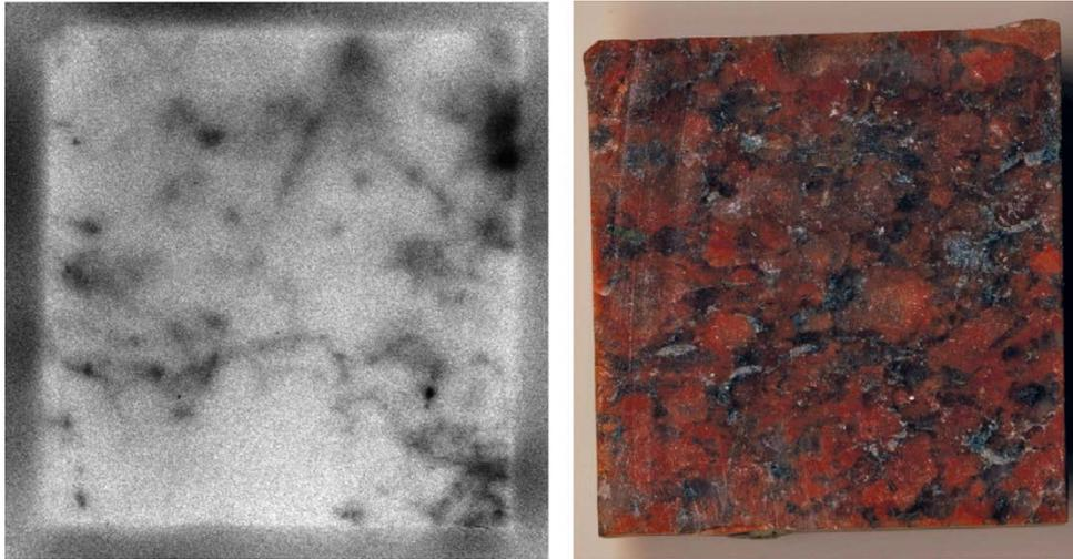
**Figure 4-28.** Autoradiograph (left) and photograph (right) of the cutting of sample A.9. The black-coloured parts in the autoradiograph may be interpreted as a network of micro-fractures, which represent preferential transport pathways. Taken from Löfgren and Nilsson (2020).
