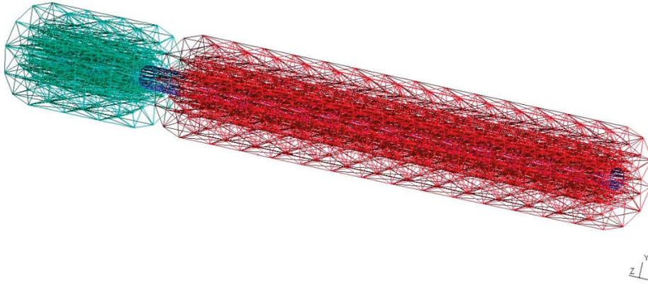
**Figure 3-6.** Computational mesh of WPDE for the blind prediction (the PGR part is hidden in order to show the discretisation of the fracture).
