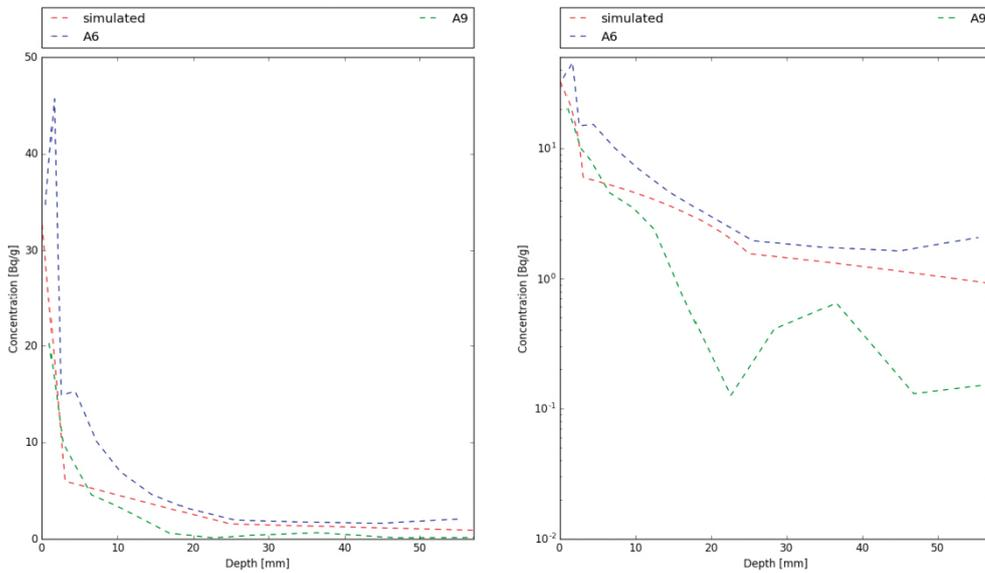
**Figure 4-13. LTDE-SD – concentration profiles in the rock in a linear (left) and logarithmic (right) scale – Na-22.**
