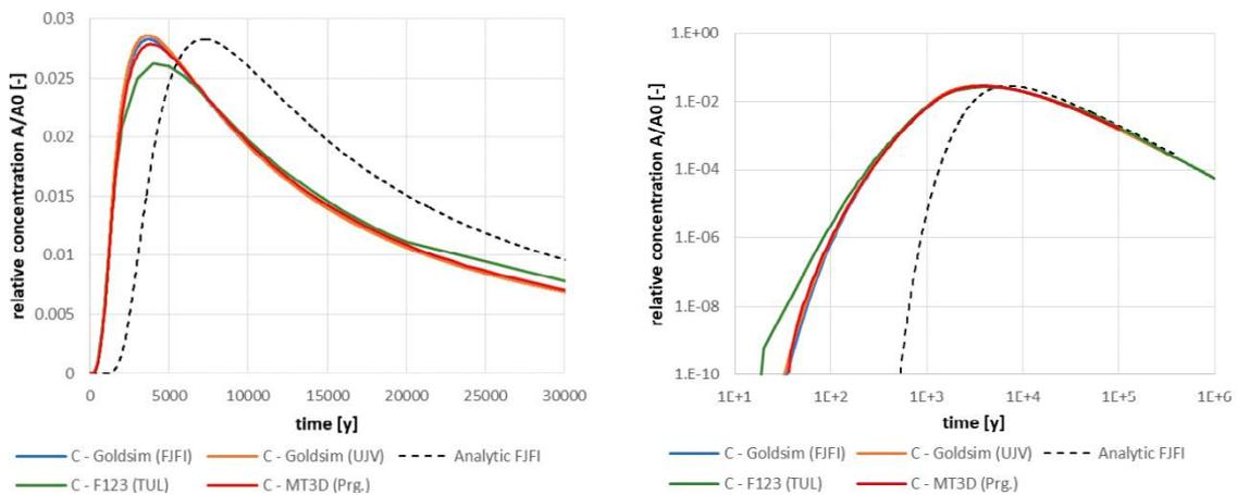
**Figure 7-9.** Comparison of solution 9D-1-a breakthrough curves in two types of axis scales for tracer C (four models).
