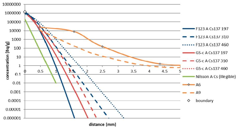
**Figure 4-9.** Comparison of profiles of Cs-137 calculated by Flow123d, GoldSim (Cell Net) for Type A and times 197 d, 310 d and 460 d, versus the measurement of profiles A6 and A9 and the original calculation in Nilsson et al. (2010).
