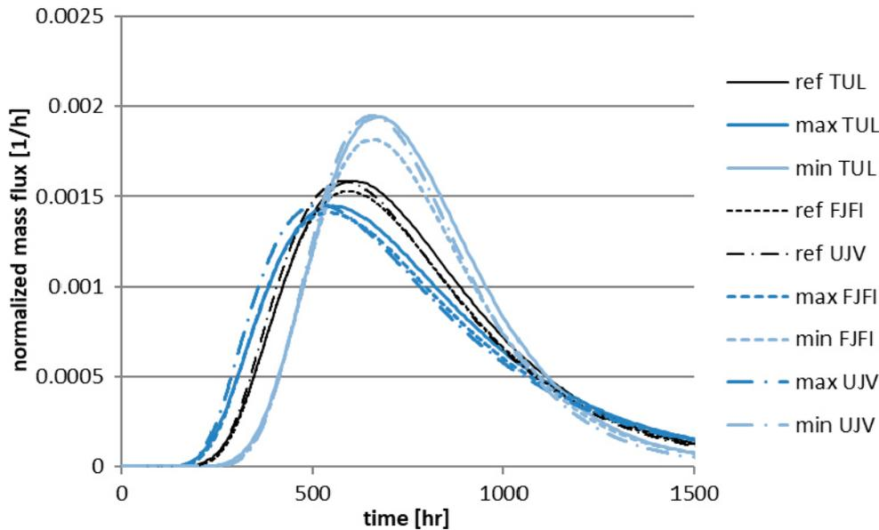
**Figure 3-17.** Sensitivity of HTO breakthrough curves in WPDE-2 to dispersion (min/max according to Table 3-7) with a comparison of three calculations.
