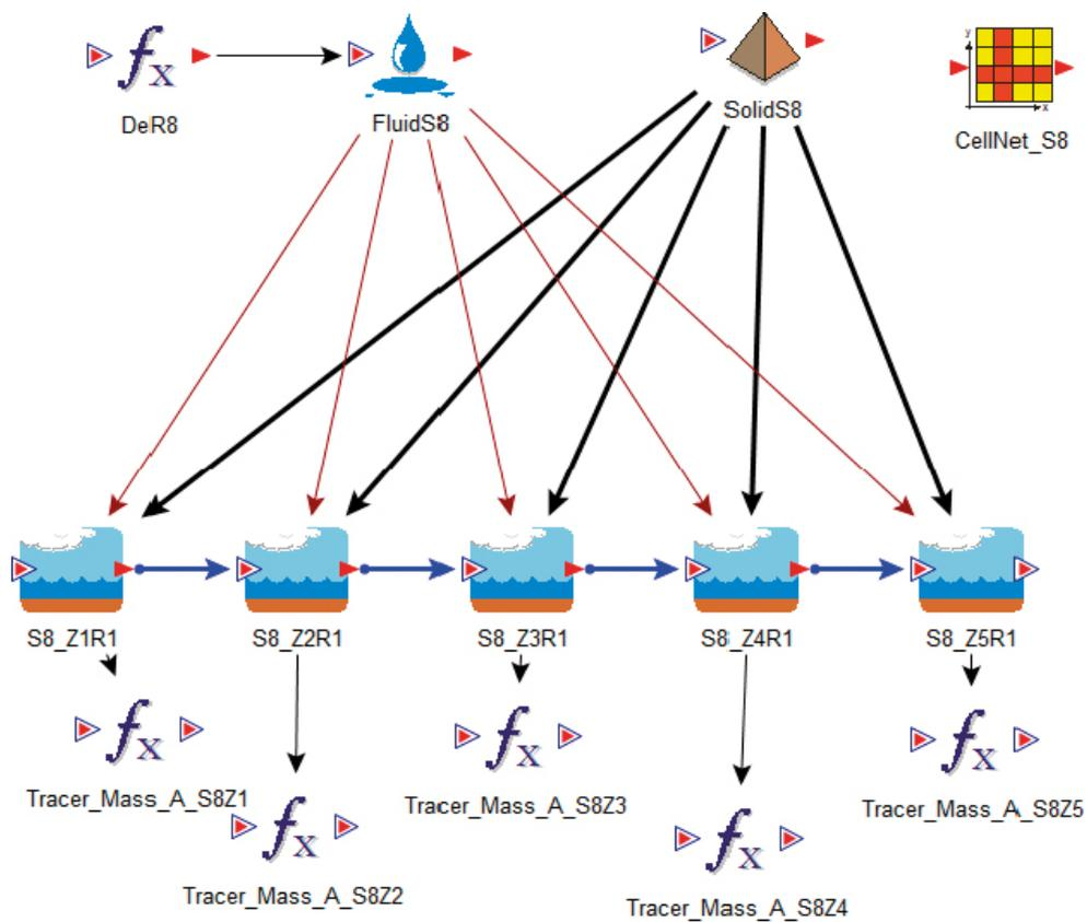
**Figure 4-23.** One of 15 separate parts of the 1D network in the graphical interface of GoldSim. In the separate parts are defined the values of the transport parameters using the FluidS8 and SolidS8 elements. The actual sub-network of the finite volumes was made up of five Cell elements (S8\_ZIR1- S8\_Z5R1), with diffusion lengths varying for the separate sections similar to the thickness of the individual sections taken from the rock.
