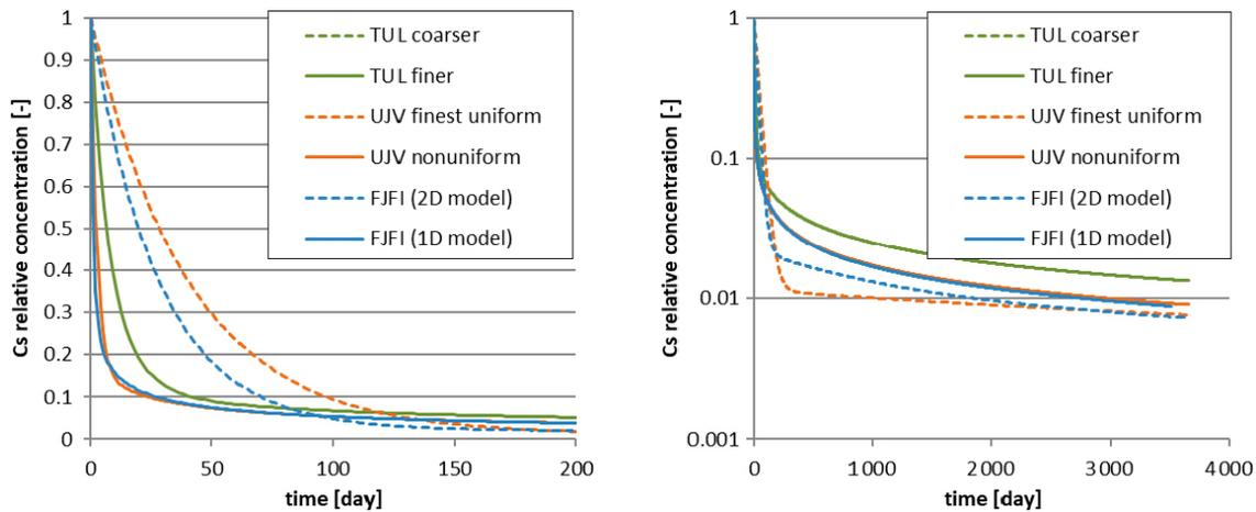
**Figure 6-12.** Comparison of results of individual investigators/software for the reference parameters – tracer Cs-134, course in the injection borehole.
