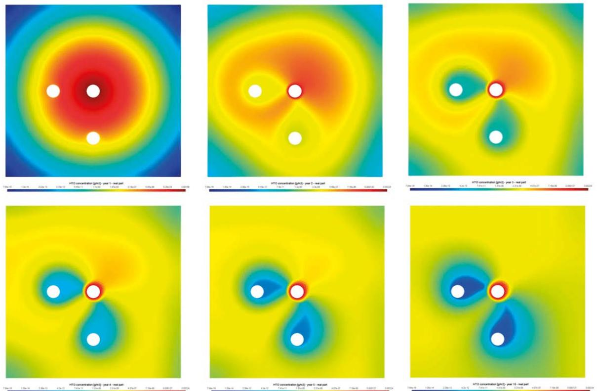
**Figure 6-20.** Task 9C – Flow123d – influence of pressure gradient – artificial pressure gradient – advection towards the injection borehole – development of the concentration field (in time 1, 2, 3, 4, 5 and 10 years).
