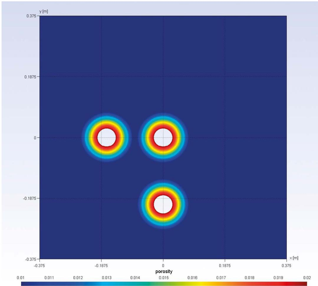
Figure 6-25. Task 9C – Flow123d – distribution of porosity in the model area.
