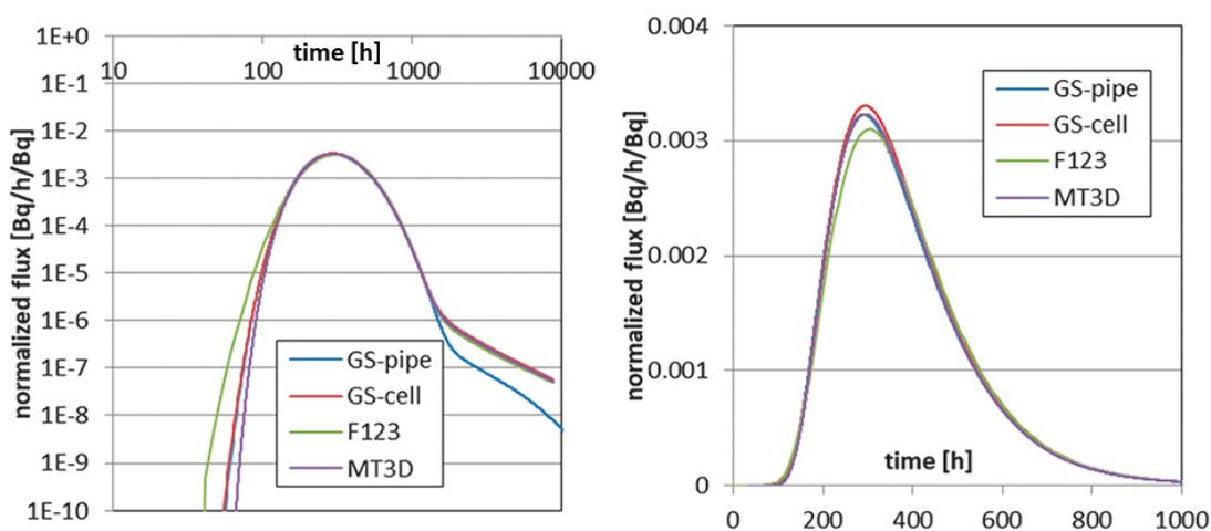
Figure 3-11. Comparison of the calculated breakthrough curves of WPDE-1 by individual models for Cl-36.
