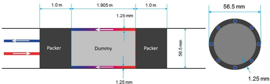
**Figure 3-1.** Configuration diagram of the WPDE experiment, which is modelled in step 9A (the solution is described below in this report) (Löfgren and Nilsson 2019).
