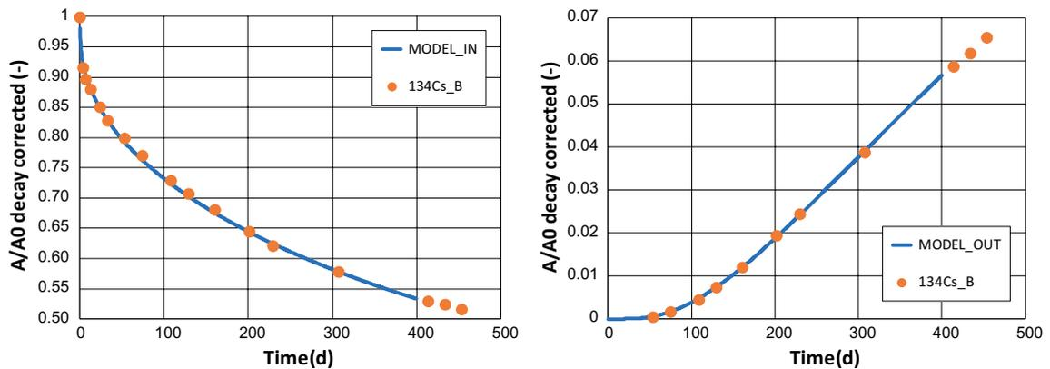
**Figure 5-8. Laboratory diffusion experiment LTDIII – comparison of the measured breakthrough curves with results of the calibrated model (inlet reservoir on the left, outlet reservoir of the diffusion cell on the right).**
