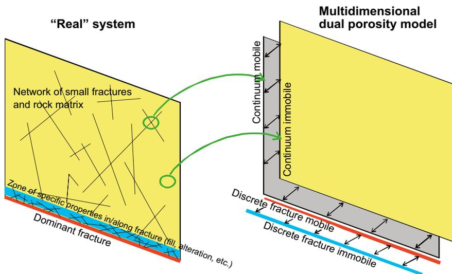
**Figure 2-1.** Illustration of the importance of connecting sub-regions of different dimensions in the transport model used in Flow123d.
