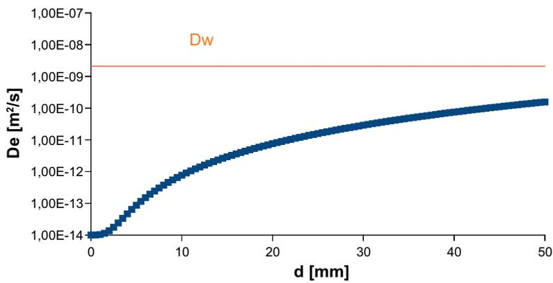
Figure 4-26. Dependence of the  $D_e$  Equation (4-1) on the distance from the source for the Cl-36 for the optimal parameter values  $D_{e0} = 1.002 \times 10^{-14}$  m<sup>2</sup>/s,  $\alpha = 3.18 \times 10^{-6}$ ,  $n = 3.13$ . The orange line indicates the limit value of the diffusion coefficient in water.
