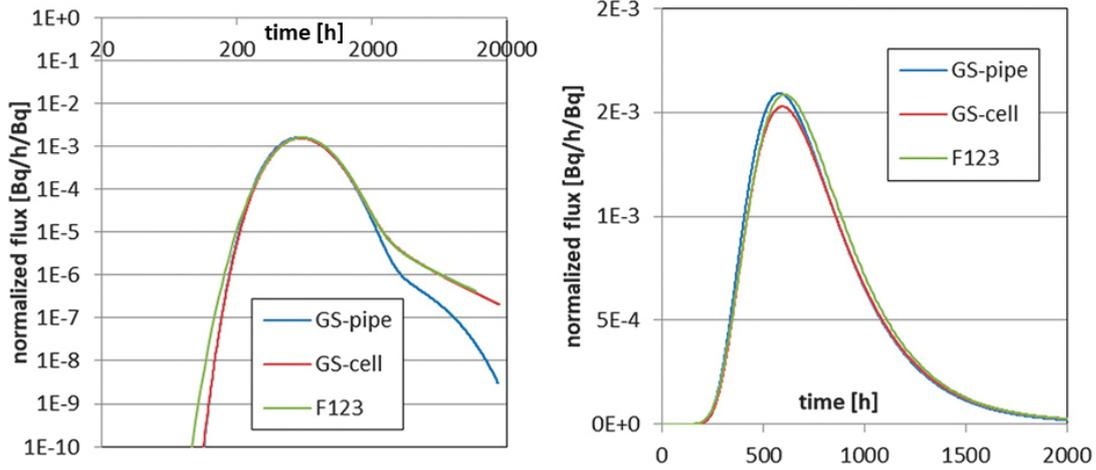
Figure 3-12. Comparison of the calculated breakthrough curves of WPDE-2 by individual models for HTO.
