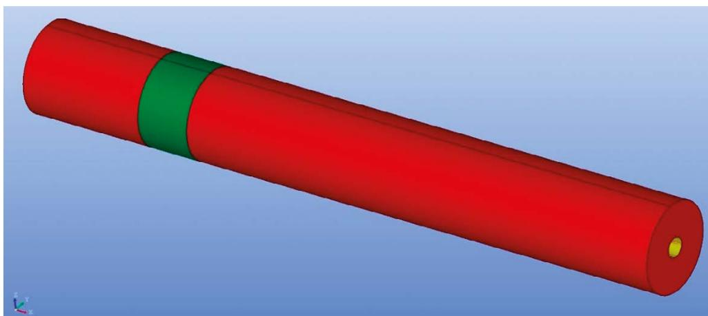
**Figure 3-5.** Geometry of the WPDE model for the blind prediction. The red part represents the veined gneiss (VGN) and the green part represents the pegmatite granite (PGR).
