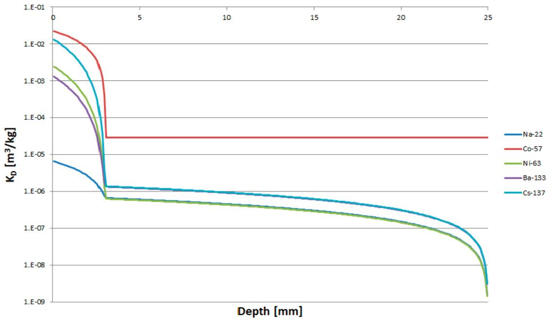
**Figure 4-12. LTDE-SD – dependence of the value of distribution coefficient of linear sorption on depth (distance from the borehole wall).**
