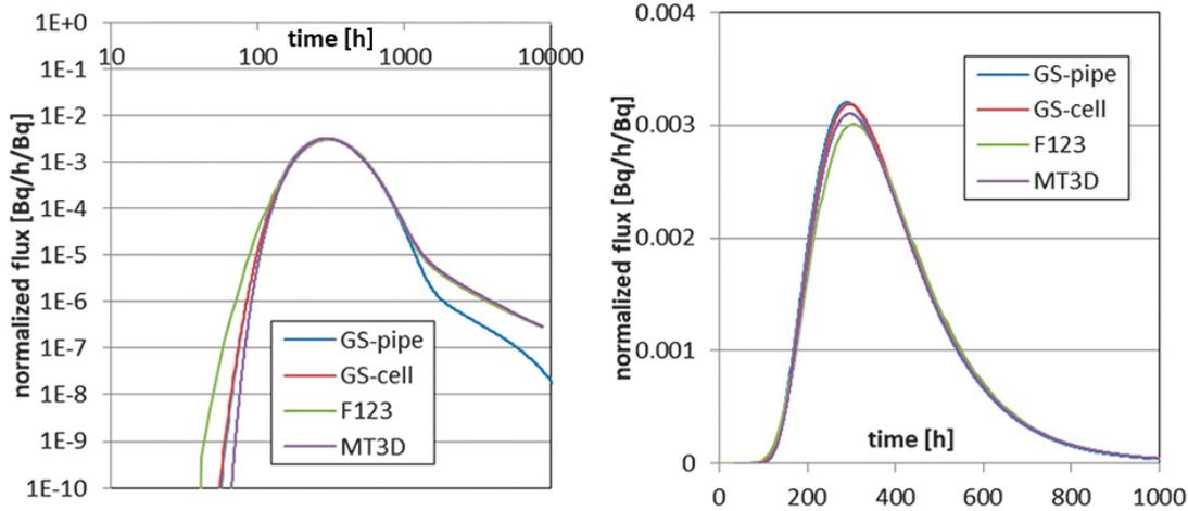
Figure 3-9. Comparison of the calculated breakthrough curves of WPDE-1 by individual models for HTO.
