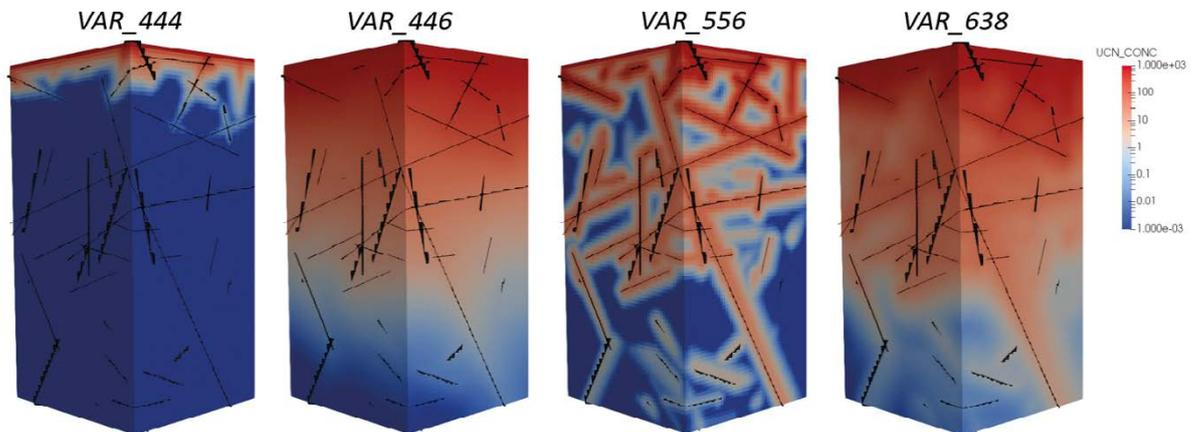
**Figure 5-5.** Variant simulations of the penetration of the tracer for various settings of transport parameters of smaller micro-fractures in the background – spatial distribution of activity in the 3D domain.
