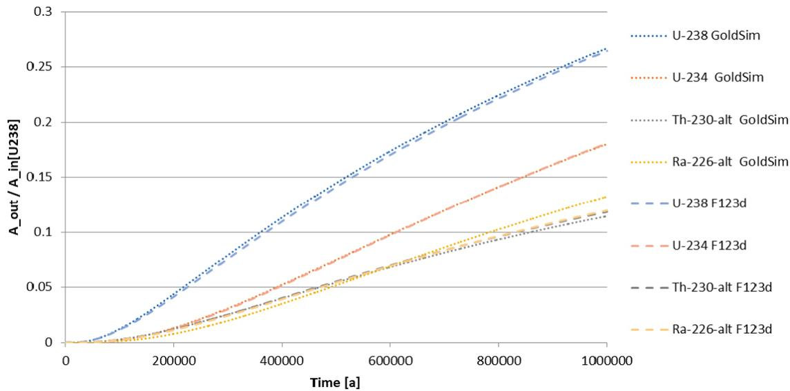
**Figure 7-16.** Breakthrough curves of the auxiliary model (profiles Po and Pb are identical to Ra in both models).
