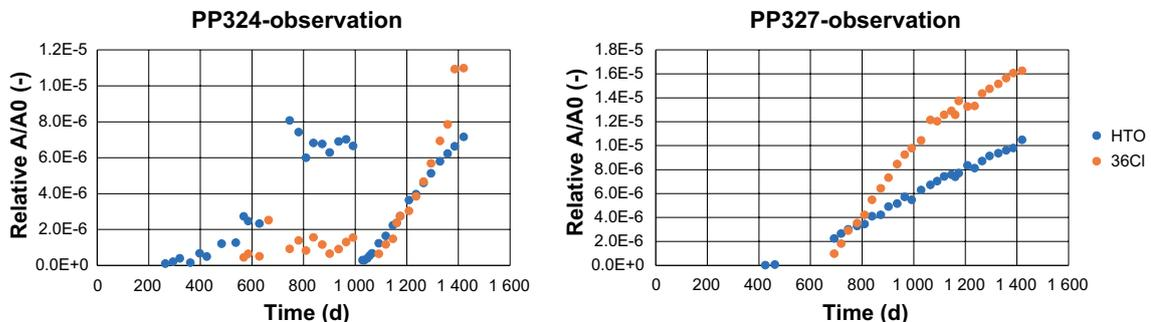
**Figure 6-44.** Task 9C – measured relative activity of HTO and Cl-36 in observation boreholes PP324 and PP327.
