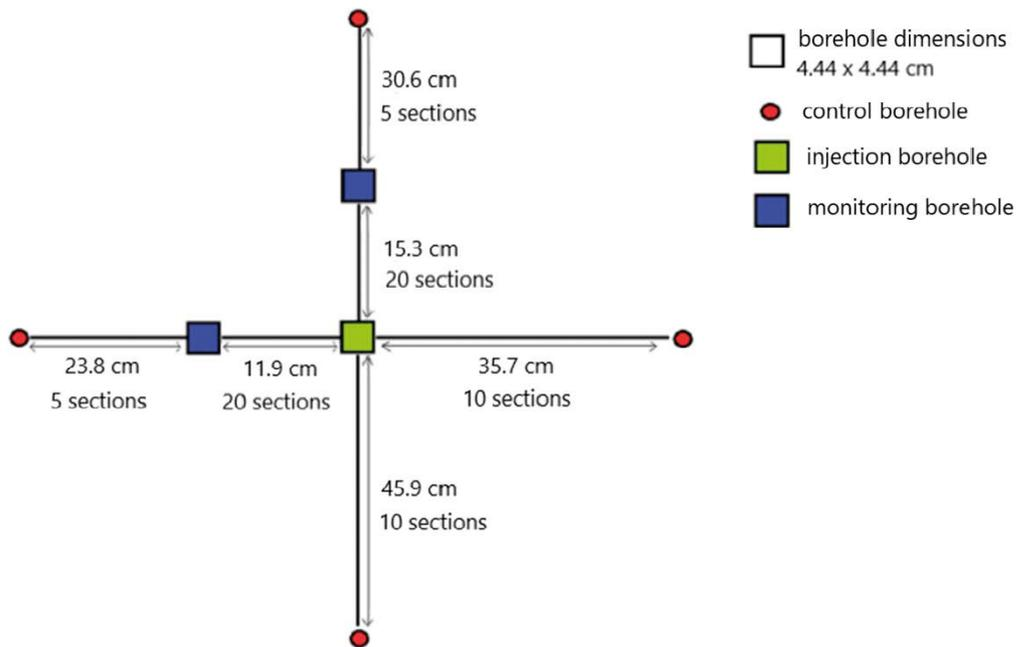
**Figure 6-4.** Representation of discretisation for non-sorbing radionuclides, finer division of the model area between the monitoring and injection boreholes.
