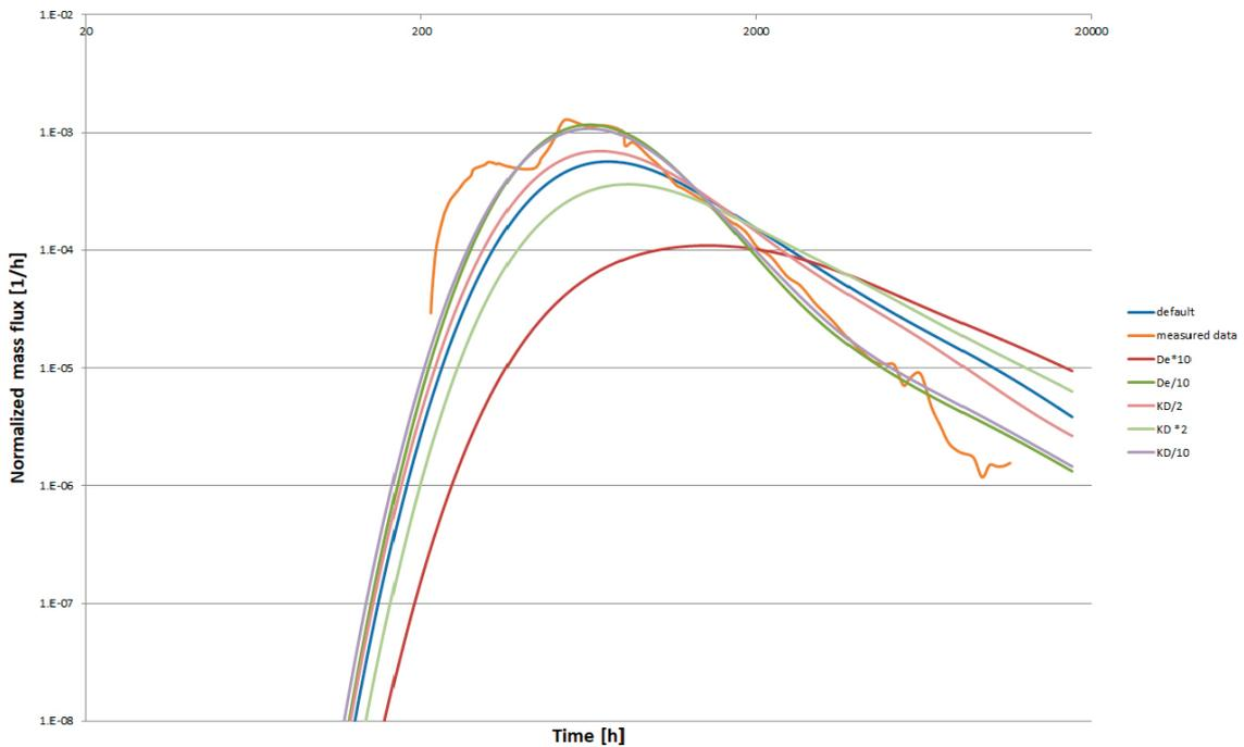
**Figure 3-22. WPDE-2 – Additional simulation, measured data – Sr-85.**
