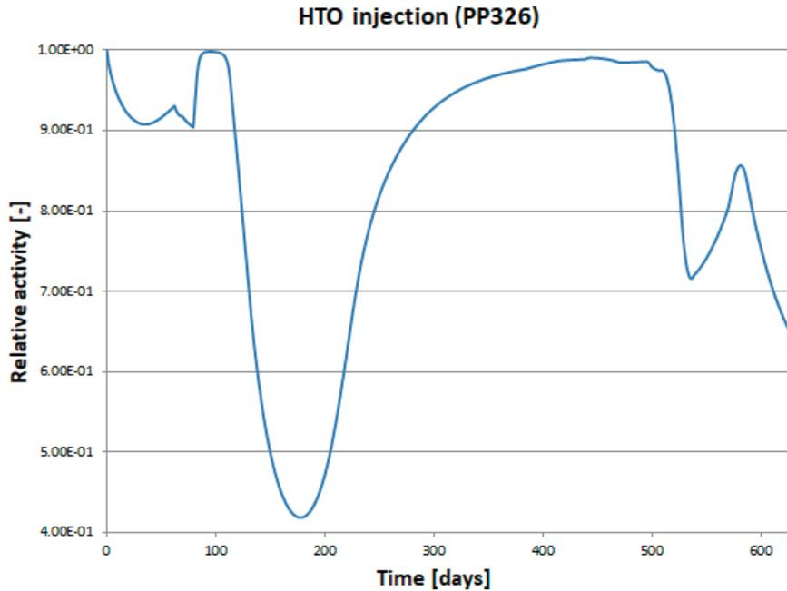
Figure 6-22. Task 9C – Flow123d – influence of pressure gradient – measured pressure gradient – dependence of the relative activity on time in the injection borehole.
