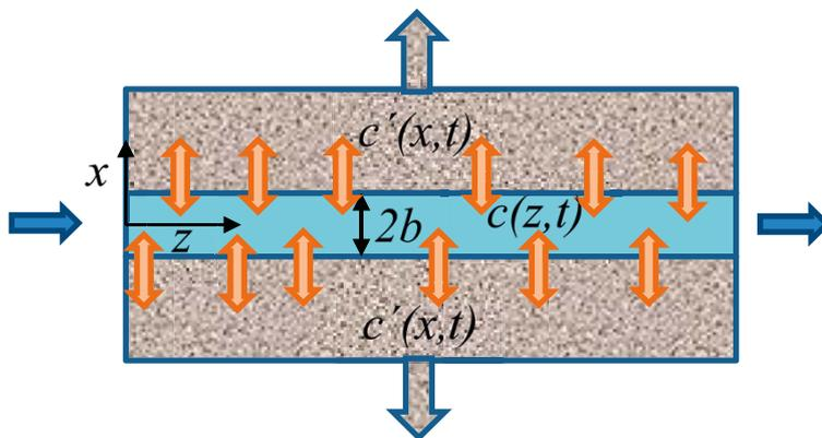
**Figure 7-3.** Diagram of transport in an idealised fracture with aperture  $2b$ ; the blue arrows indicate the direction of advective flow, orange arrows diffusion into the matrix,  $c(z,t)$  indicates the concentration of radionuclide in the flowing water,  $c'(x,z,t)$  the concentration in the pore water of the rock matrix.
