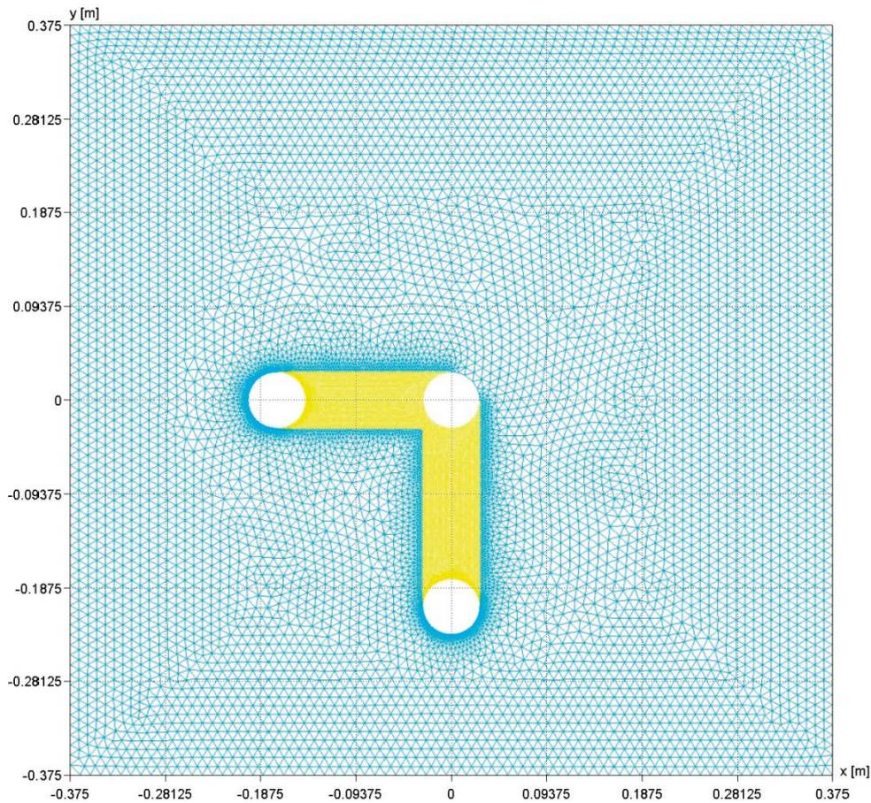
**Figure 6-2.** Task 9C – Flow123d – computational mesh of the model.
