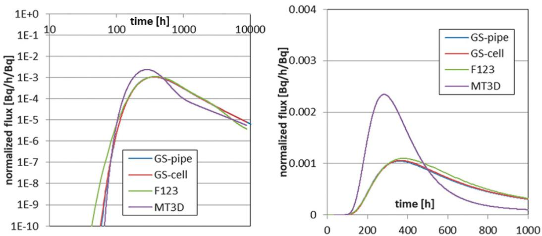
Figure 3-10. Comparison of the calculated breakthrough curves of WPDE-1 by individual models for Na-22.
