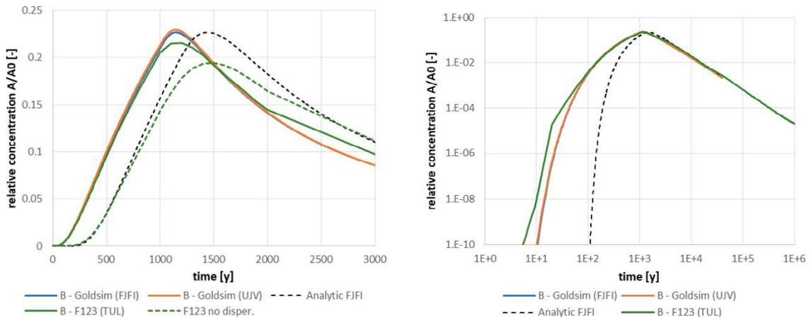
**Figure 7-8.** Comparison of solution 9D-1-a breakthrough curves in two types of axis scales for tracer B (three models and variants without dispersion corresponding to the analytical solution).
