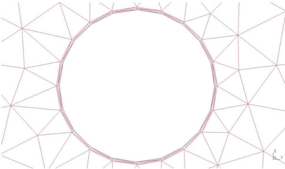
**Figure 3-7.** Computational mesh of WPDE for the blind prediction – cross-section. Two thin layers of matrix elements around the fracture.
