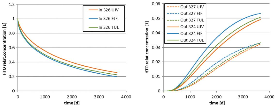
**Figure 6-8.** Comparison of results of individual investigators/software for the reference parameters – tracer HTO, course in the injection borehole on the left and in both detection boreholes on the right.
