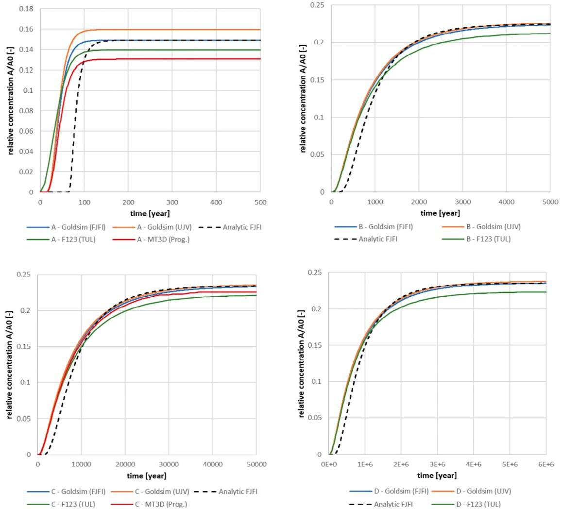
Figure 7-11. Comparison of solution 9D-1-b breakthrough curves for all of the tracers (A – 4 models, B – 3 models, C – 4 models, D – 3 models).
