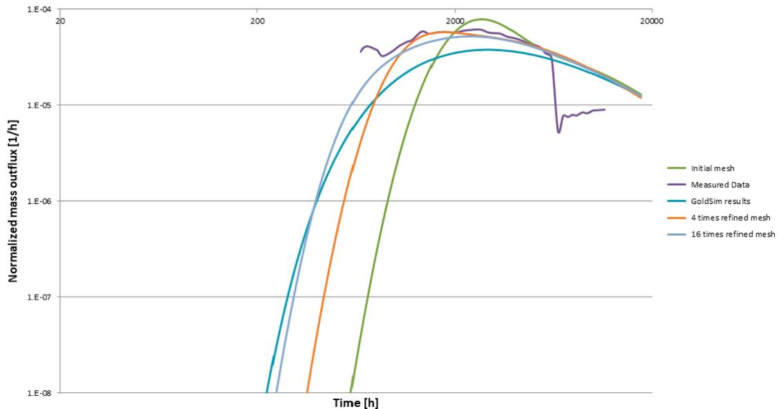
**Figure 3-24.** WPDE-2 – Ba-133 – effect of discretisation, comparison between measured data and results of the GoldSim model.
