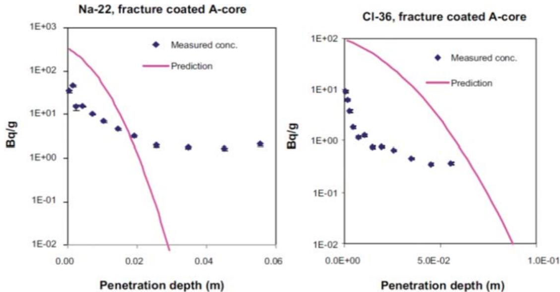
**Figure 4-5.** Results of the in-situ diffusion experiment LTDE-SD – concentration profiles for Na-22 and Cl-36. Measured data vs the model. Taken from Nilsson et al. (2010, Figures 4-1a and 4-2a).
