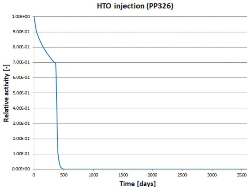
**Figure 6-16.** Task 9C – Flow123d – influence of pressure gradient – artificial pressure gradient – advection towards the monitoring boreholes – dependence of relative activity on time in the injection borehole.
