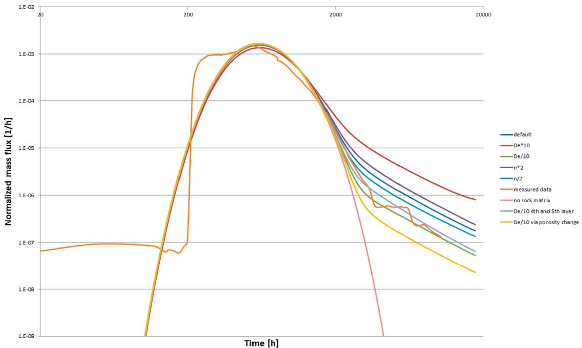
**Figure 3-21.** WPDE-2 – Additional simulation, measured data – HTO.
