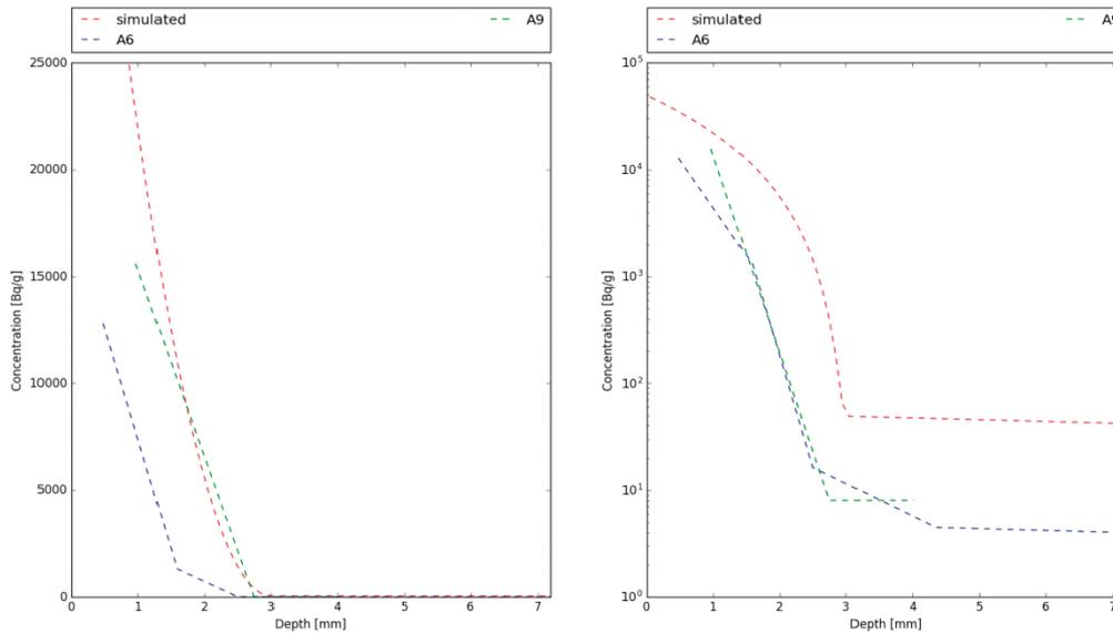
**Figure 4-21.** *LTDE-SD – Stage\_2 – concentration profiles in the rock in a linear (left) and logarithmic (right) scale – Ni-63.*
