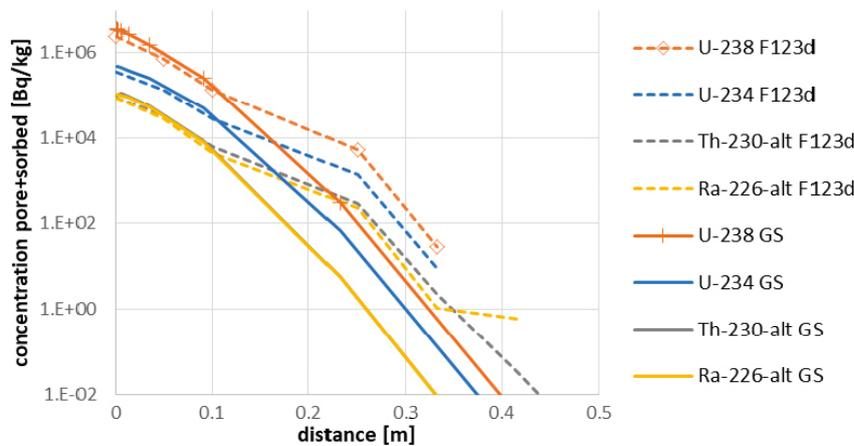
**Figure 7-17.** Transverse profiles in the auxiliary model (Po and Pb profiles are identical to Ra in both models).
