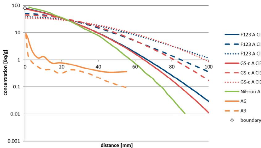
**Figure 4-7.** Comparison of profiles of Cl-36 calculated by Flow123d, GoldSim (Cell Net) for Type A and times 197 d, 310 d and 460 d, versus the measurement of profiles A6 and A9 and the original calculation in Nilsson et al. (2010).
