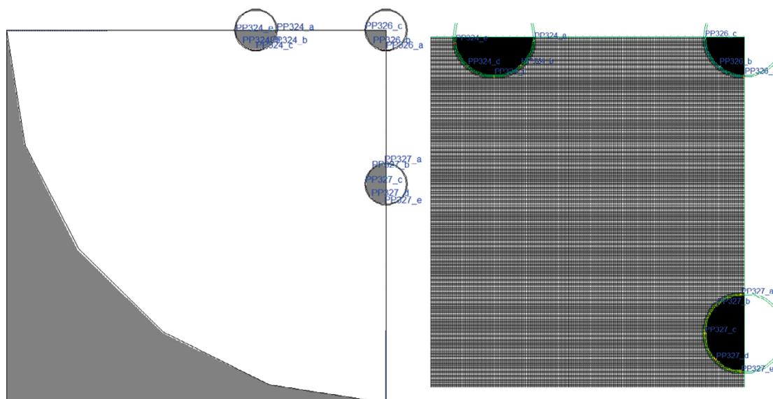
**Figure 6-45.** Task 9C – MT3DMS – discretisation of the model domain – size of the whole model  $500 \times 500$  mm on the left, the cutting with the grid of model cells  $1 \times 1$  mm on the right.
