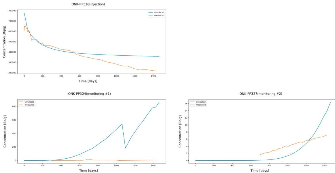
Figure 6-27. Task 9C – Flow123d – results of the inverse model, HTO variant 2.
