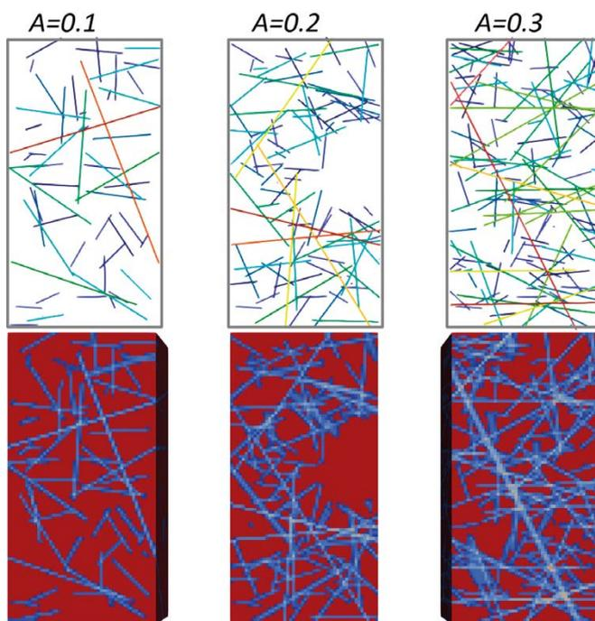
**Figure 5-4.** Cross-sections generated by micro-fracture networks for different values of parameter A of the power function. Above: cross-sections of the micro-DFN model, below: models converted to the micro-CPM model.
