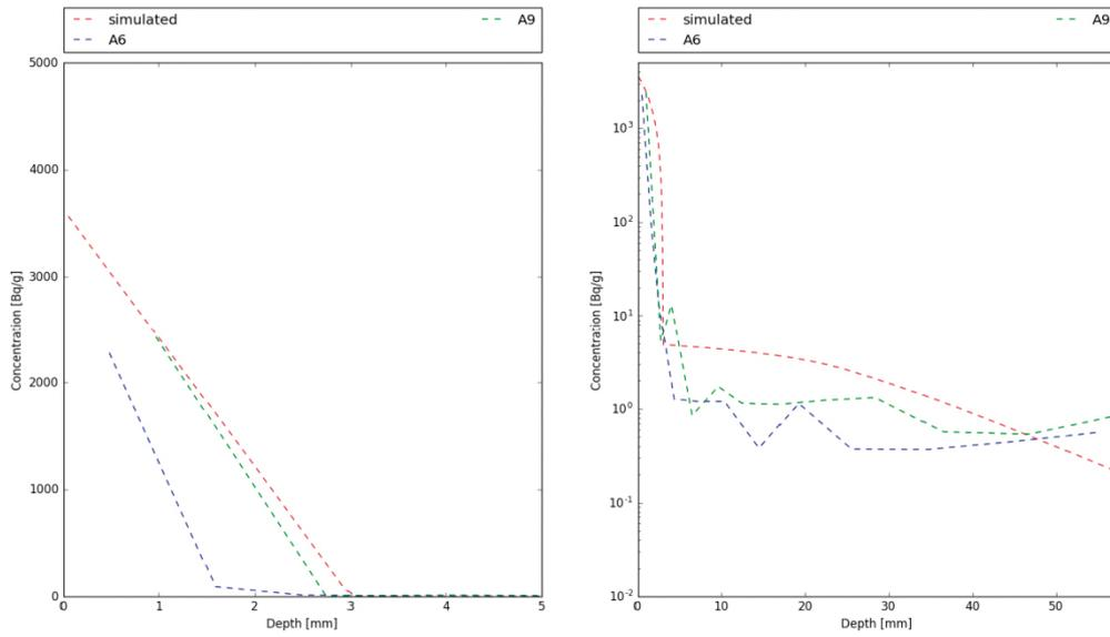
Figure 4-15. LTDE-SD – concentration profiles in the rock in a linear (left) and logarithmic (right) scale – Co-57.
