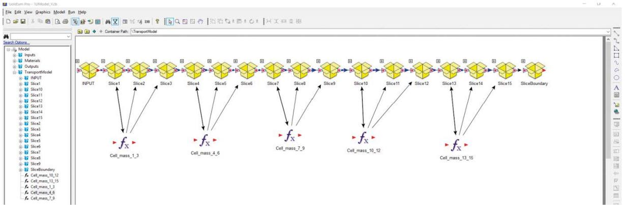
**Figure 4-22.** Division of the 1D network into 15 separate parts in the graphical interface of GoldSim.
