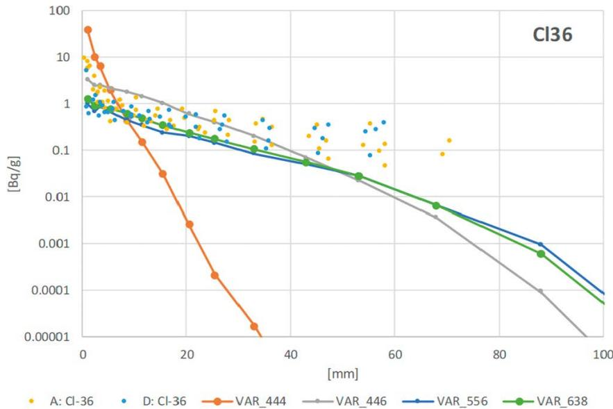
**Figure 5-6.** Variant simulation of the penetration of the tracer for various settings of transport parameters of smaller micro-fractures in the background – amount of tracer in cross-sections by the model domain.
