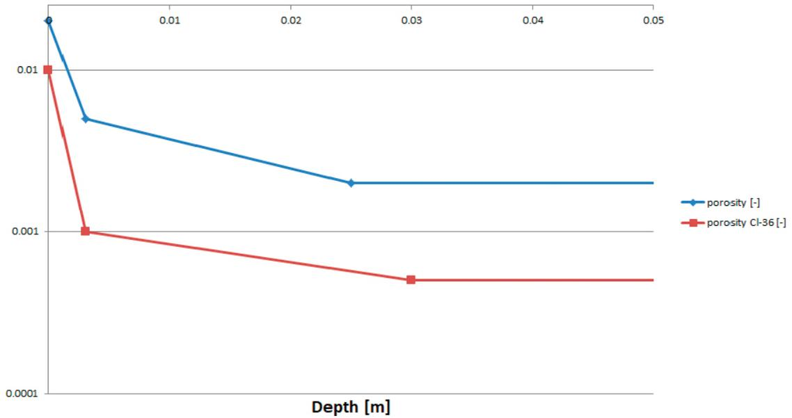
**Figure 4-11. LTDE-SD – dependence of the porosity value on depth (distance from the borehole wall).**
