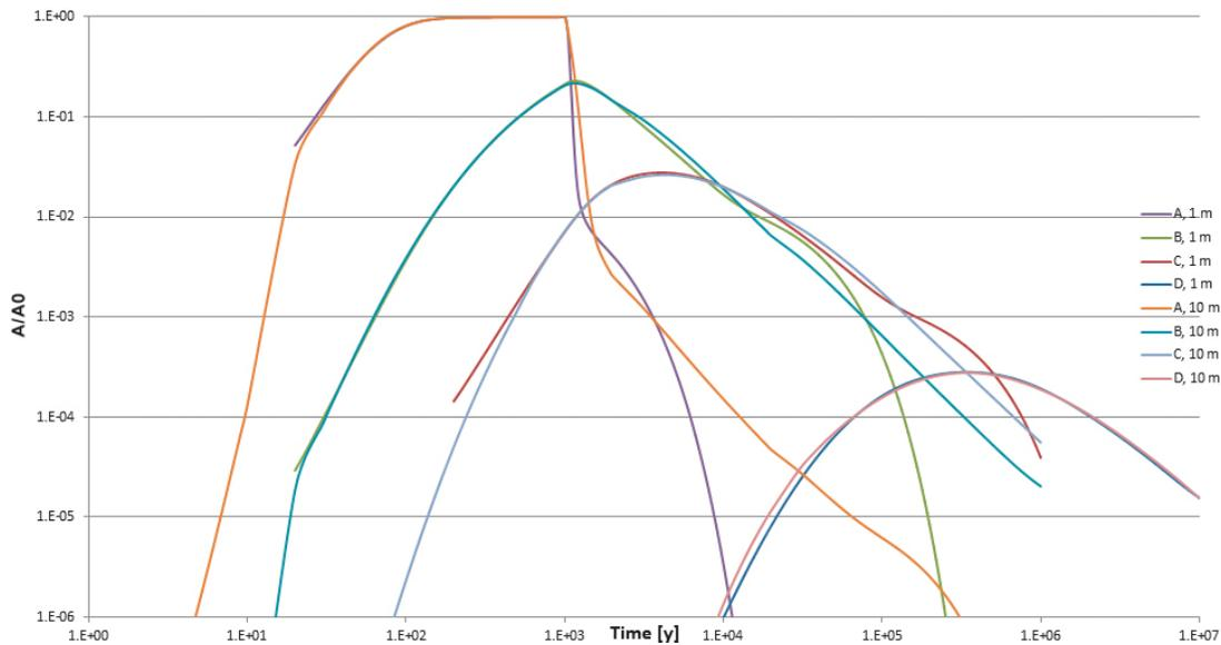
Figure 7-22. Task9D-1a – influence of rock matrix thickness – normalised breakthrough curves.
