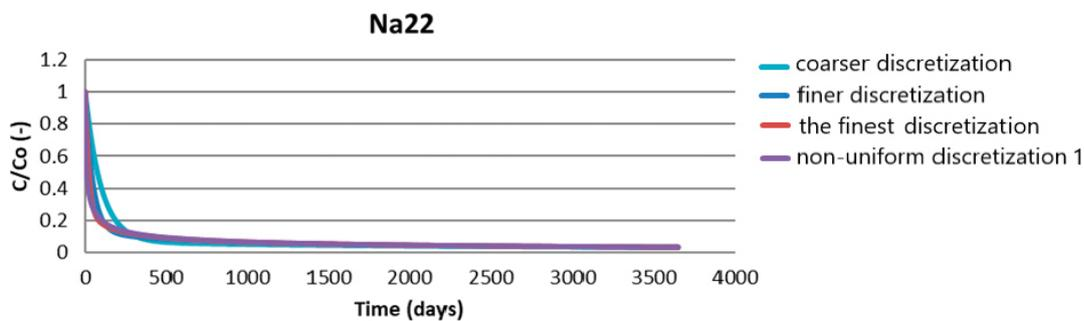
**Figure 6-13.** Development of Na-22 activity in the injection borehole for the four considered types of discretisation of the ÚJV-GoldSim model.
