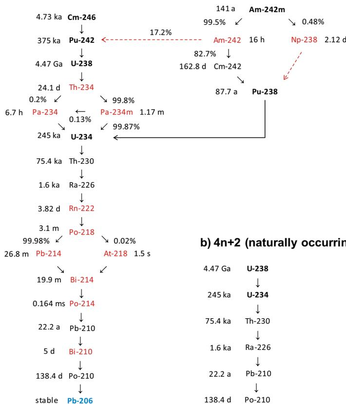
**Figure 7-2. Derivation of a simplified decay series (taken from Crawford et al. 2021).**
