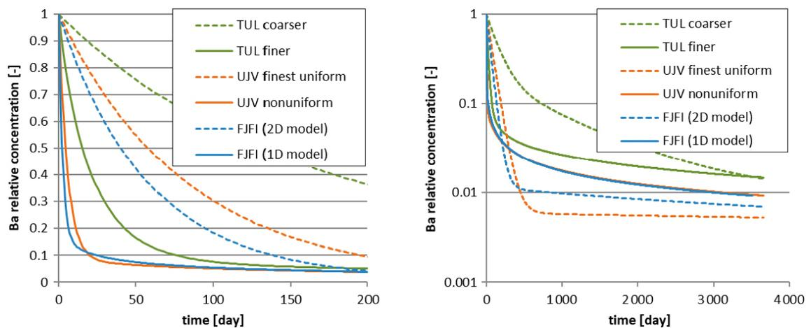
**Figure 6-11.** Comparison of results of individual investigators/software for the reference parameters – tracer Ba-133, course in the injection borehole.
