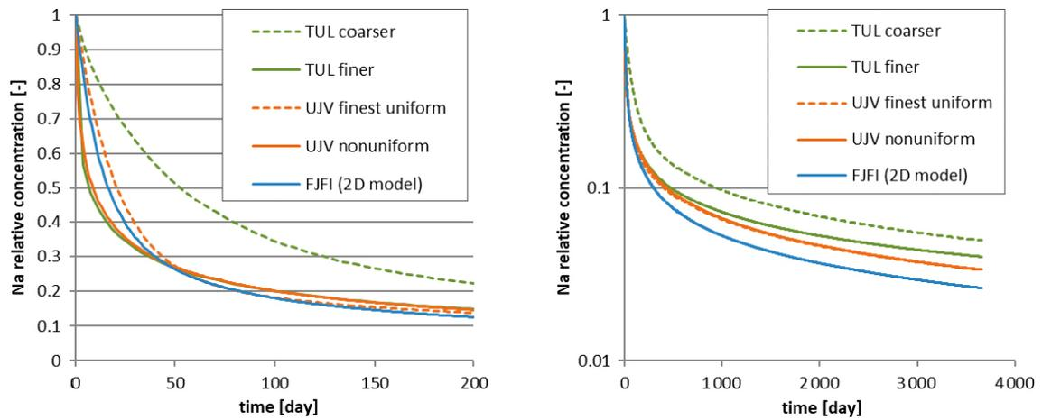
**Figure 6-10.** Comparison of results of individual investigators/software for the reference parameters – tracer Na-22, course in the injection borehole in two different axis scales.
