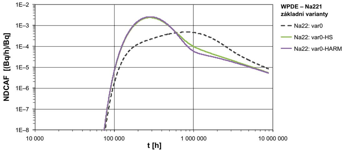
Figure 3-25. Effect of the model discretisation on the course of the breakthrough curve for Na-22 (var0).
