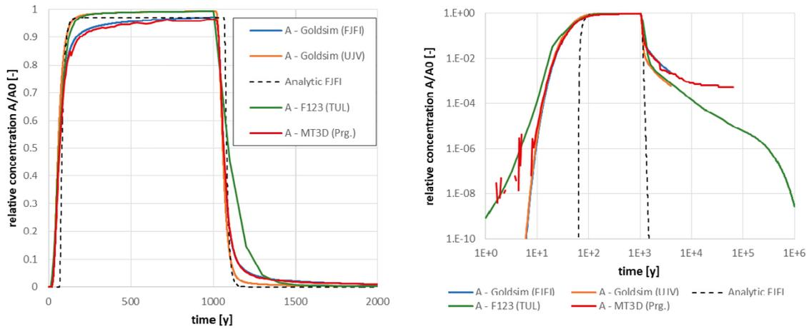
**Figure 7-7.** Comparison of solution 9D-1-a breakthrough curves in two types of axis scales for tracer A (four models); in this case, the analytical solution is for the advection-only model (without the matrix diffusion).
