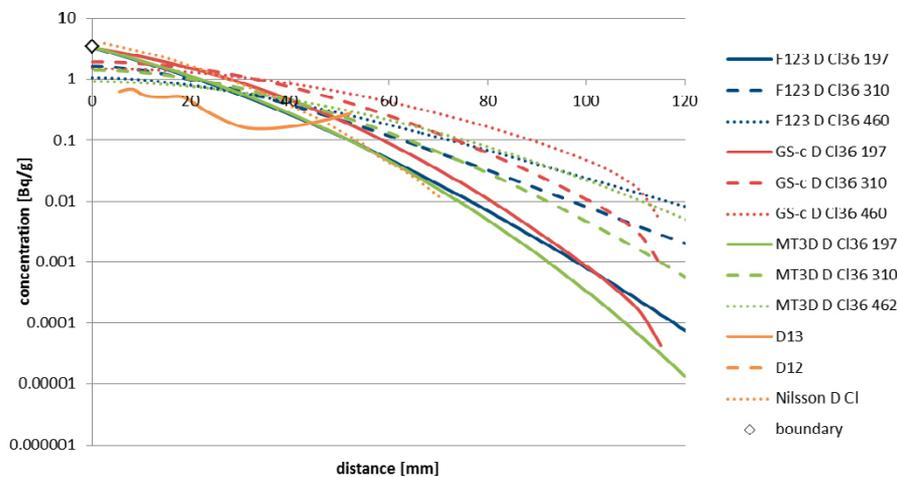
**Figure 4-10.** Comparison of profiles of Cl-36 calculated by Flow123d, GoldSim (Cell Net) and MT3DMS for Type D and times 197 d, 310 d and 460 d, versus the measurement of profiles D12 and D13 and the original calculation in Nilsson et al. (2010).
