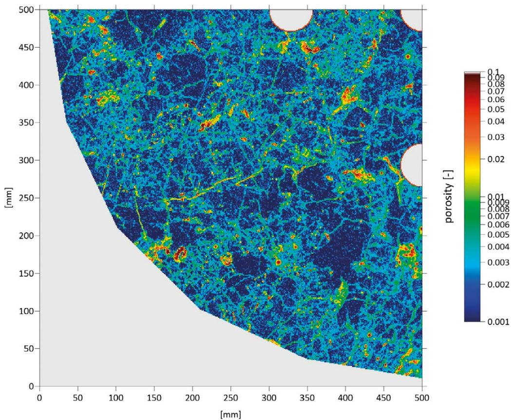
**Figure 6-48.** Task 9C – Variant 3 – heterogeneous porosity based on the rock matrix micrograph.
