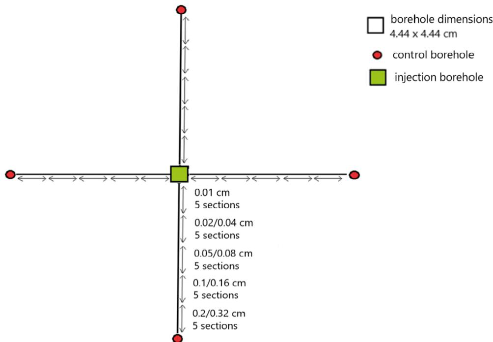
**Figure 6-6.** Representation of non-uniform discretisation for sorbing radionuclides, discretisation of the model area was made in two variants, the discretisation in the x-axis direction is the same as the discretisation in the y-axis direction.
