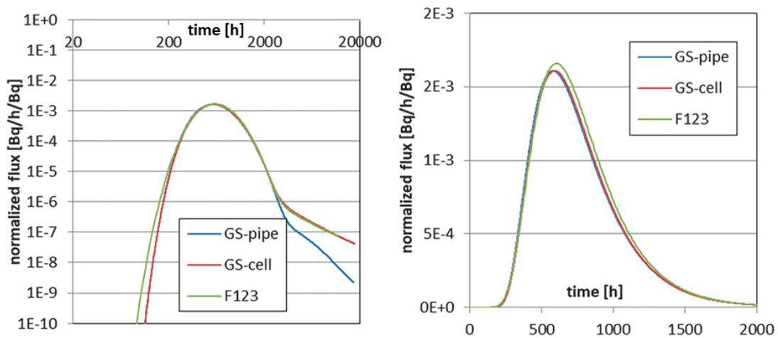
Figure 3-14. Comparison of the calculated breakthrough curves of WPDE-2 by individual models for Cl-36.
