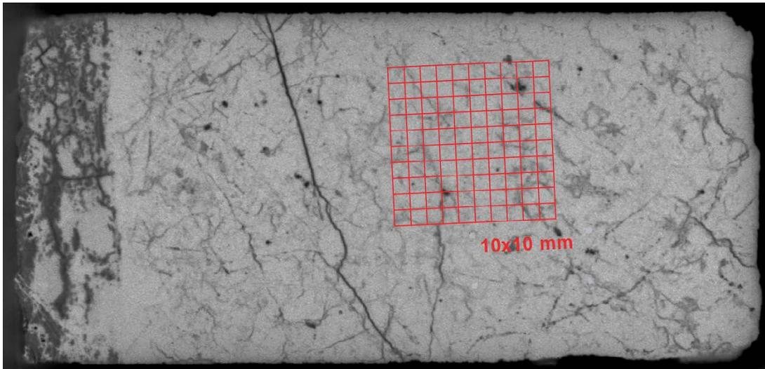
*Figure 5-2. Microstructure image obtained by the C-14-PMMA method – sample LTDE-SD2 (DD18, 2017).*
