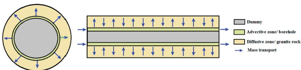
**Figure 3-2.** Conceptual model of radionuclide transport in the WPDE experiment for Task 9A.
