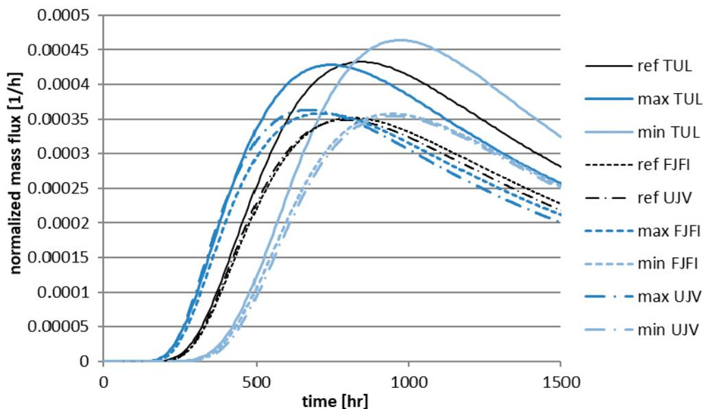
**Figure 3-18.** Sensitivity of N-22 breakthrough curves in WPDE-2 to dispersion (min/max according Table 3-7) with a comparison of three calculations.
