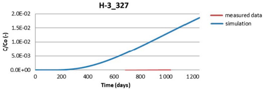
Figure 6-35. Development of activity in the monitoring borehole.
