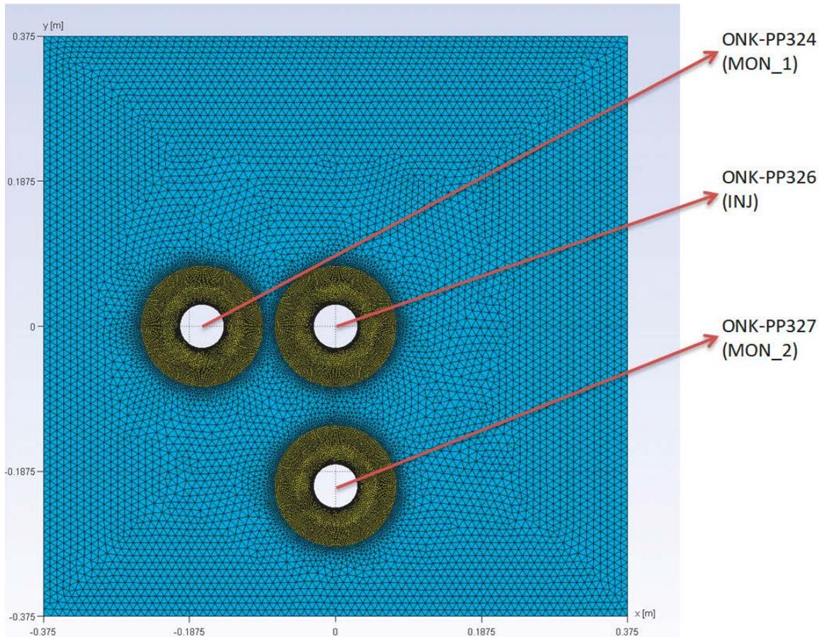
**Figure 6-24.** Task 9C – Flow123d – updated computational mesh for the inverse model.
