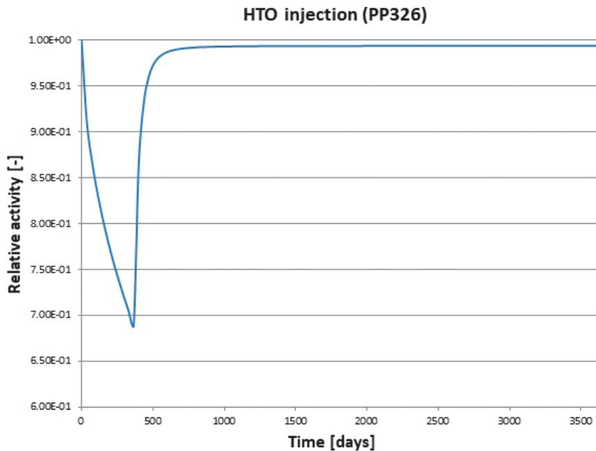
**Figure 6-18.** Task 9C – Flow123d – influence of pressure gradient – artificial pressure gradient – advection towards the injection borehole – dependence of relative activity on time in the injection borehole.
