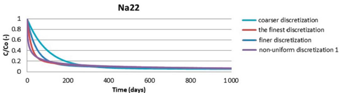
**Figure 6-14.** Detail of the development of Na-22 activity in the injection borehole for the four considered types of discretisation of the ÚJV-GoldSim model.
