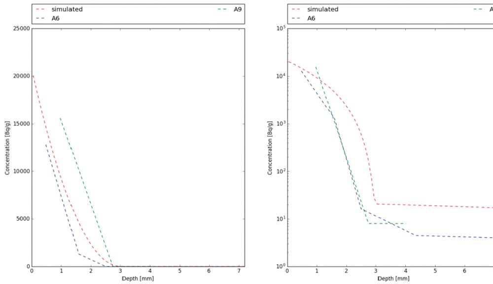
Figure 4-16. LTDE-SD – concentration profiles in the rock in a linear (left) and logarithmic (right) scale – Ni-63.
