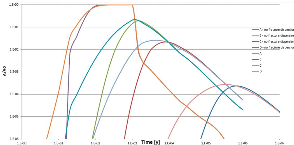
Figure 7-23. Task9D-1a – influence of dispersion in the fracture – normalised breakthrough curves.
