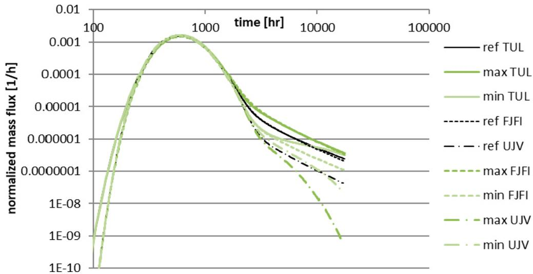
**Figure 3-19.** Sensitivity of HTO breakthrough curves in WPDE-2 to porosity (min/max according to Table 3-7) with a comparison of three calculations.
