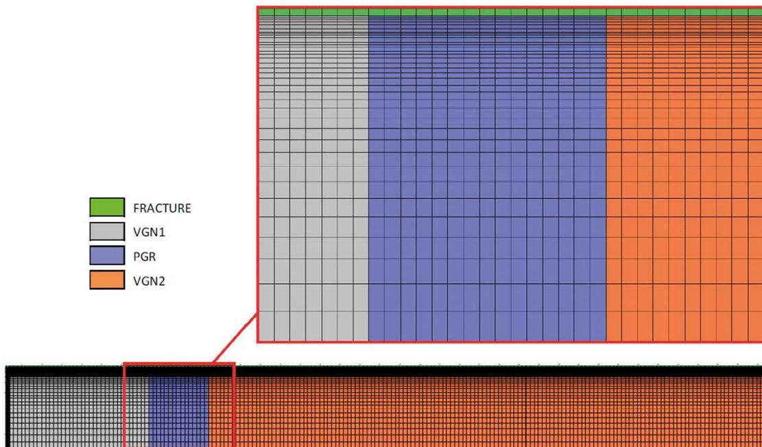
*Figure 3-8. Geometry and discretisation of the model.*
