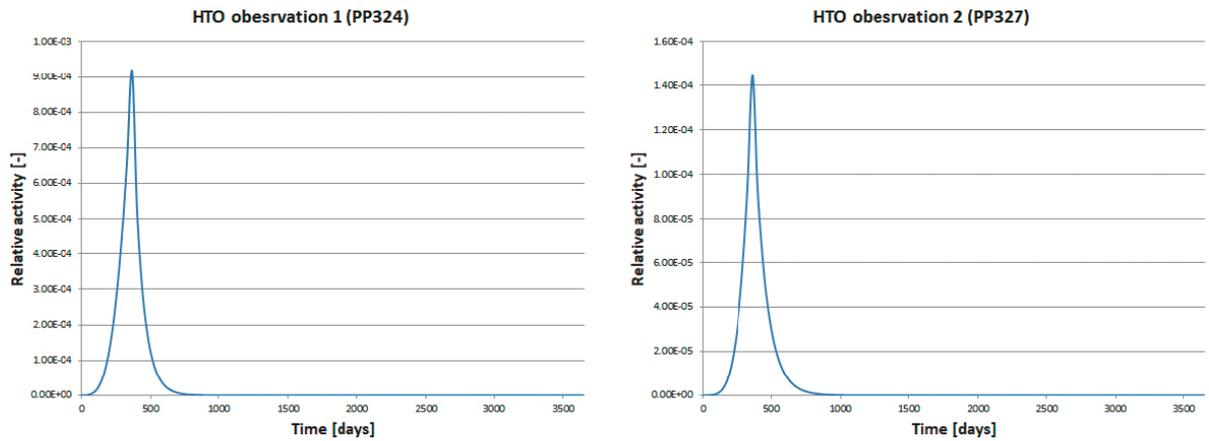
**Figure 6-19.** Task 9C – Flow123d – influence of pressure gradient – artificial pressure gradient – advection towards the injection borehole – dependence of relative activity on time in the monitoring boreholes.
