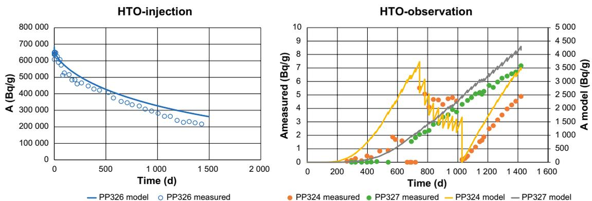
**Figure 6-46.** Task 9C – simulation of HTO in MT3DMS – Variant 1 – calibration of activity in injection borehole PP326. Comparison of the measured and model evolutions in the injection boreholes on the left and breakthrough curves in the observation boreholes on the right.
