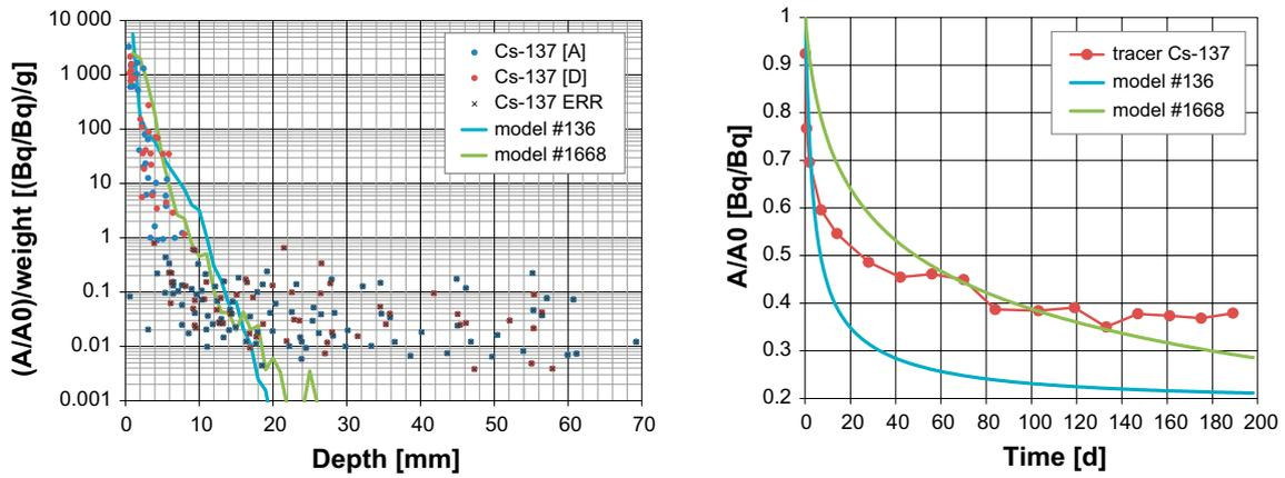
Figure 5-11. Cs-137 – comparison of measured data and model results – cross-sections of the sample and model domain on the left, course of the activity in the source reservoir on the right.
