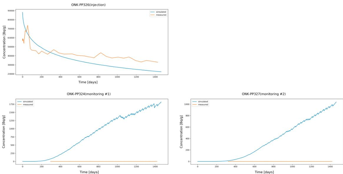
**Figure 6-29.** Task 9C – Flow123d – results of the inverse model, Na-22.
