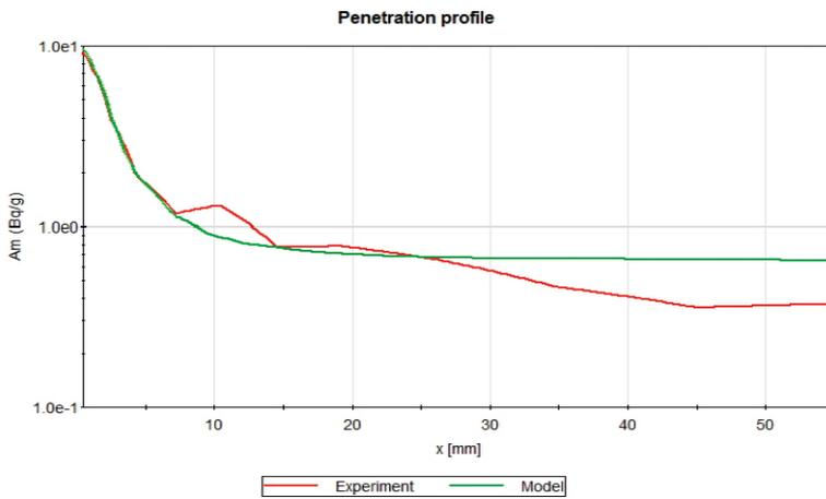
Figure 4-25. Comparison of experimental and model profile of Cl-36 activity in the rock layer.
