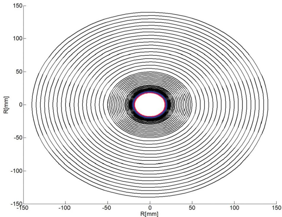
**Figure 4-29.** Detail of the geometry of the cylindrical grid of the model of the D sample; the different areas of the various different model rocks (spatially variable parameters) are represented by different colours.
