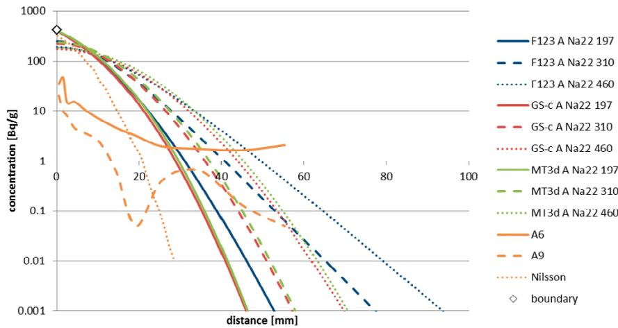
**Figure 4-6.** Comparison of profiles of Na-22 calculated by Flow123d, GoldSim (Cell Net) and MT3DMS for Type A and times 197 d, 310 d and 460 d, versus the measurement of profiles A6 and A9 and the original calculation in Nilsson et al. (2010).
