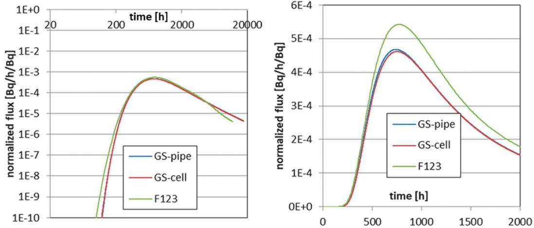
Figure 3-15. Comparison of the calculated breakthrough curves of WPDE-2 by individual models for Sr-85.
