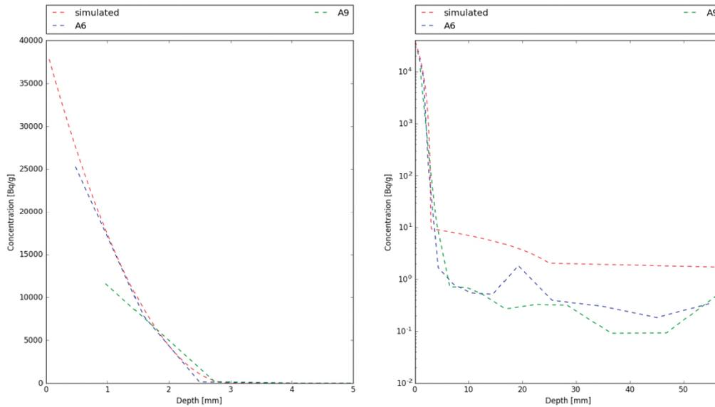
**Figure 4-18.** LTDE-SD – concentration profiles in the rock in a linear (left) and logarithmic (right) scale – Cs-137.
