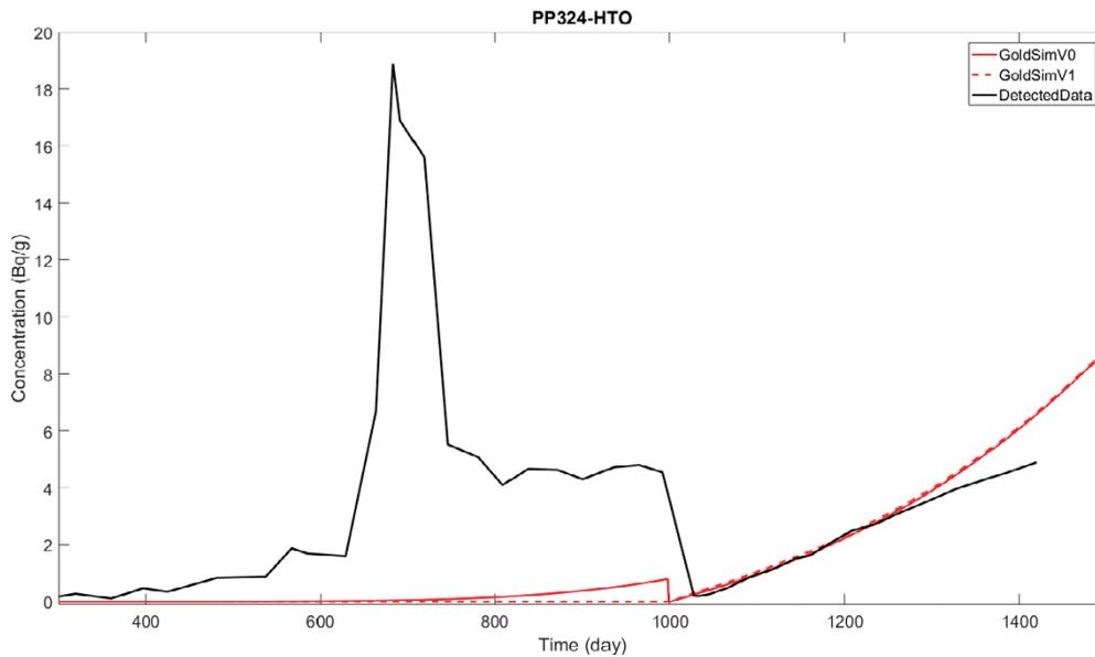
**Figure 6-51.** Comparison of the time course of concentrations in PP324 for a model with PP324 without boundary conditions.
