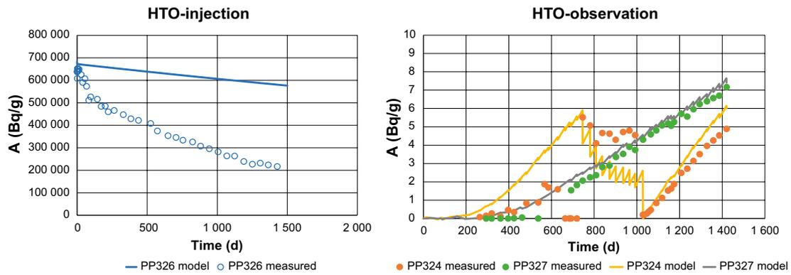
**Figure 6-47.** Task 9C – simulation of HTO in MT3DMS – Variant 2 – calibration of activity in observation boreholes PP324 and PP327. Comparison of the measured and model evolutions in the injection boreholes on the left, in the observation boreholes on the right.
