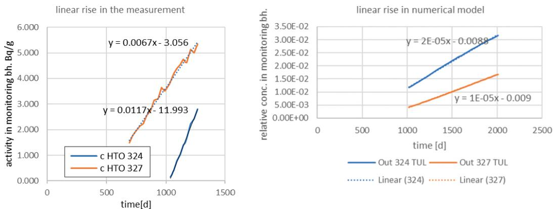
**Figure 6-49.** Verification of assumption of a linear increase of concentrations in monitoring boreholes (324/327) and of the related steady-state diffusive transport. Linear regressions: left for the measured data (original units) and right for the numerical model result for a representative time interval (dimensionless).
