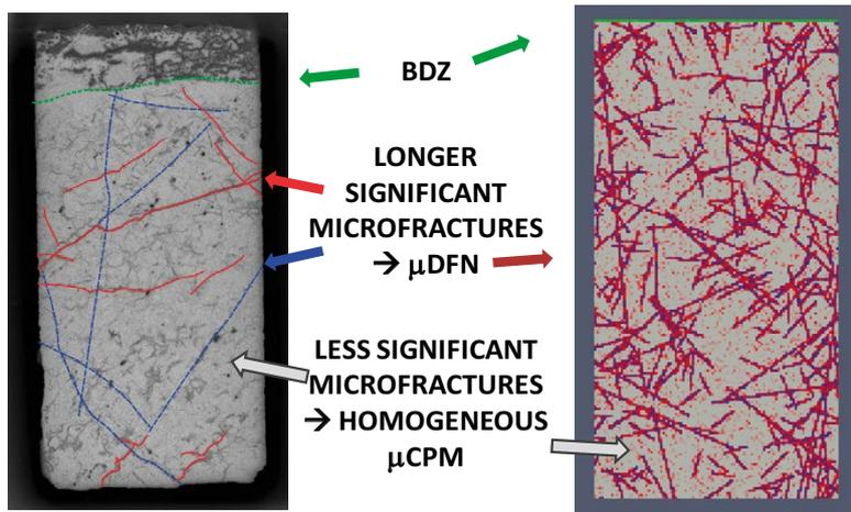
**Figure 5-3.** Definition of the basic elements characteristic of the rock matrix – BDZ, longer significant micro-fractures and less significant micro-fractures forming the background of the image. Rock matrix micrograph (LTDE-SD2 sample) on the left and a micro-CPM model with a randomly generated network of micro-fractures in the cross-section on the right.
