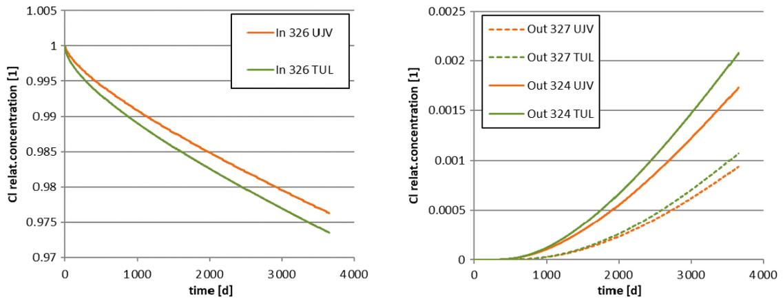
**Figure 6-9.** Comparison of results of individual investigators/software for the reference parameters – tracer Cl-36, course in the injection borehole on the left and in both detection boreholes on the right.
