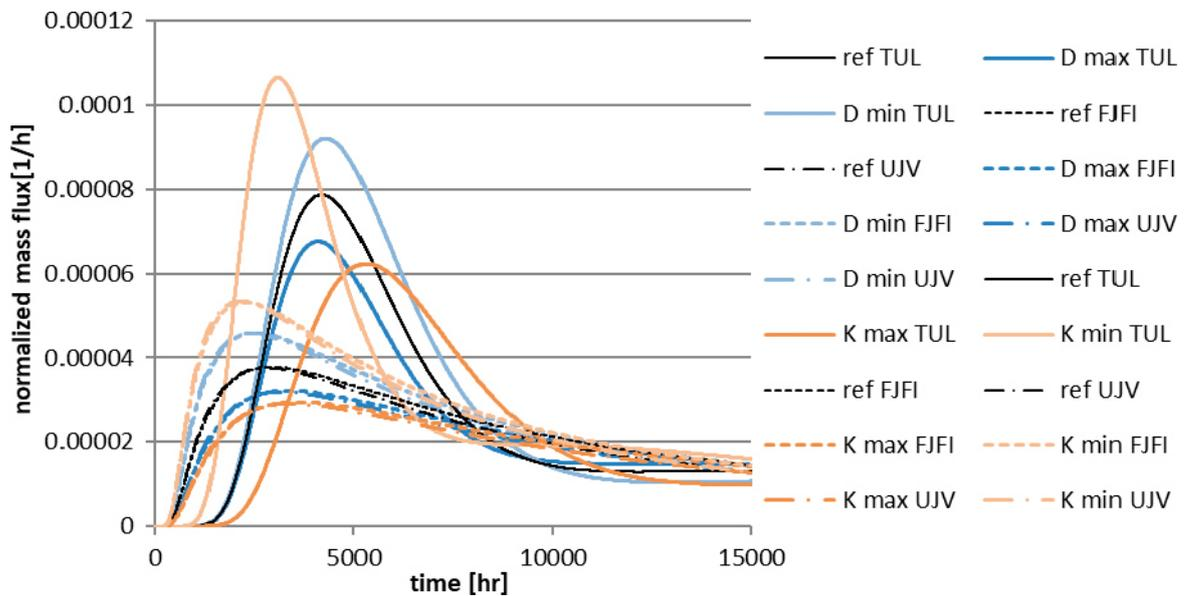
**Figure 3-20.** Sensitivity of Ba-133 breakthrough curves in WPDE-2 to the effective diffusion coefficient (D) and sorption coefficient (K) (min/max according to Table 3-7) with a comparison of three calculations.
