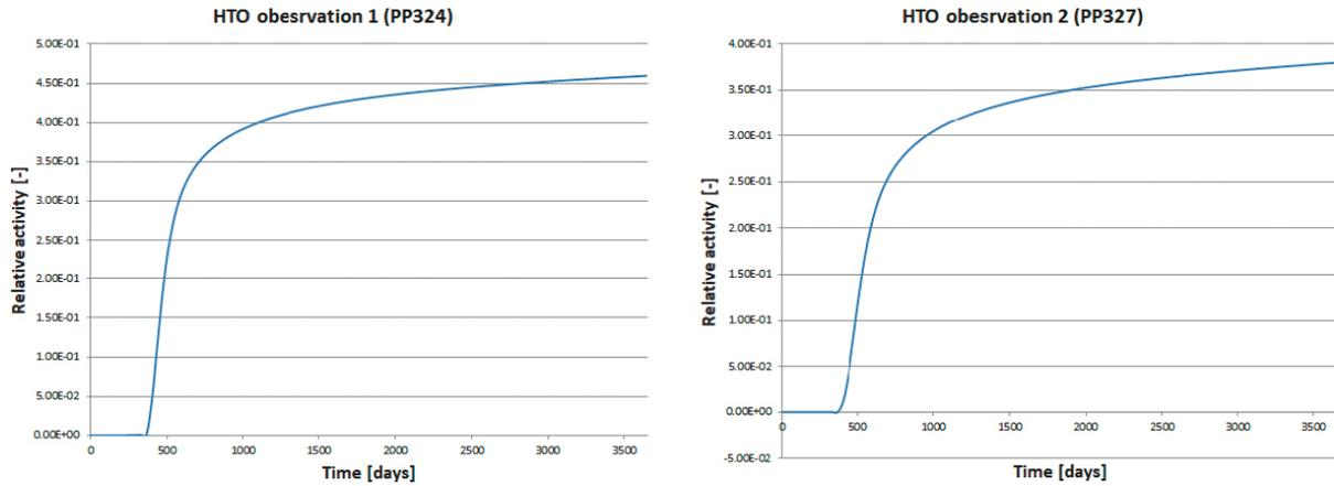
**Figure 6-17.** Task 9C – Flow123d – influence of pressure gradient – artificial pressure gradient – advection towards the monitoring boreholes – dependence of relative activity on time in the monitoring boreholes.
