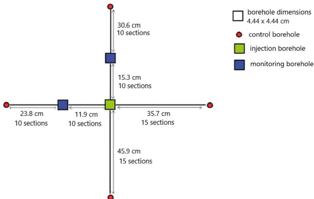
**Figure 6-3. Representation of discretisation for non-sorbing radionuclides, coarser division of the model area between the monitoring and injection boreholes.**
