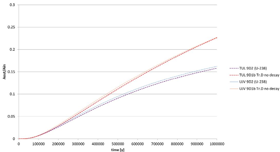
**Figure 7-15.** A control comparison of the breakthrough curves of 9D-1 (tracer *D*) and 9D-2 (uranium) between Flow123d(*TUL*) and GoldSim (*UJV*).
