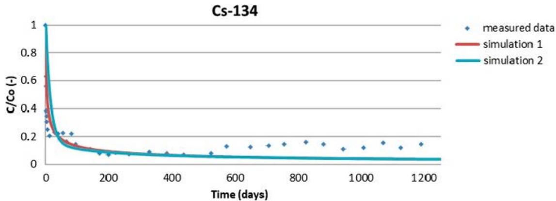
**Figure 6-43.** Agreement between the measured and model results for different combinations of model parameters, development of activity in the injection borehole.
