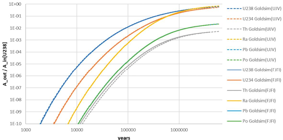
Figure 7-13. Comparison of solution 9D-2 breakthrough curves for six radionuclides in the decay series (Pb is graphically indistinguishable from Po) – two independently processed GoldSim calculations.
