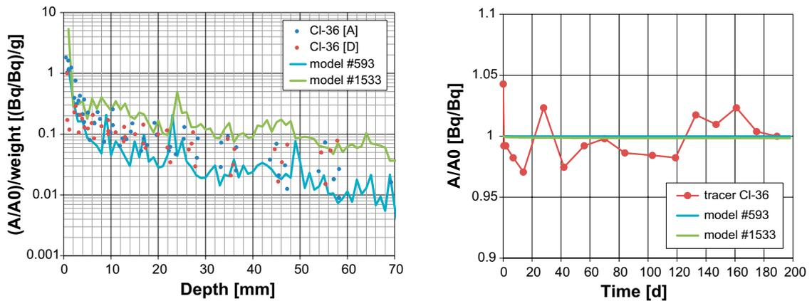
**Figure 5-9. Cl-36 – comparison of measured data and model results – cross-sections of the sample and model domain on the left, course of the activity in the source reservoir on the right.**
