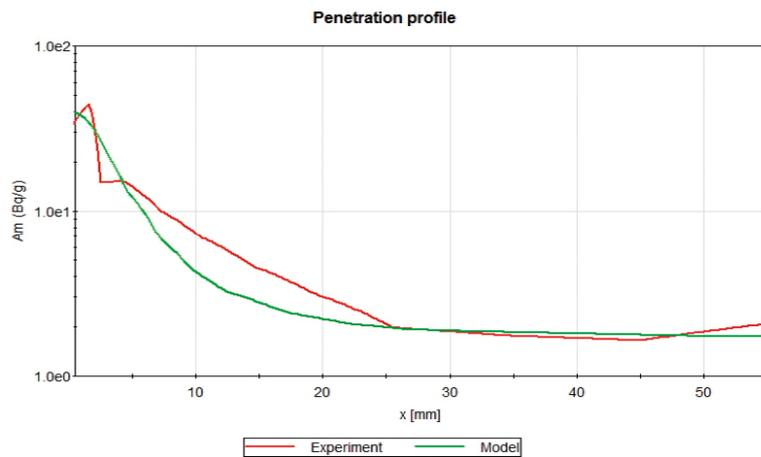
**Figure 4-27.** Comparison of experimental and model profile of Na-22 activity in the rock layer.
