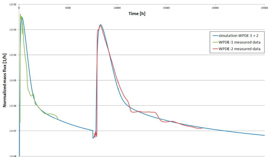
Figure 3-23. WPDE – sequential simulation of both experiments – results – HTO.
