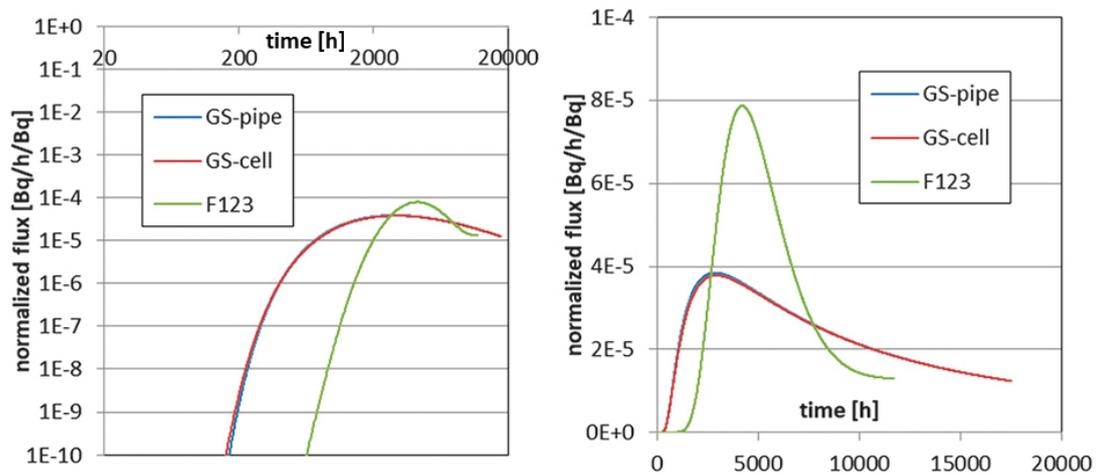
Figure 3-16. Comparison of the calculated breakthrough curves of WPDE-2 by individual models for Ba-133.
