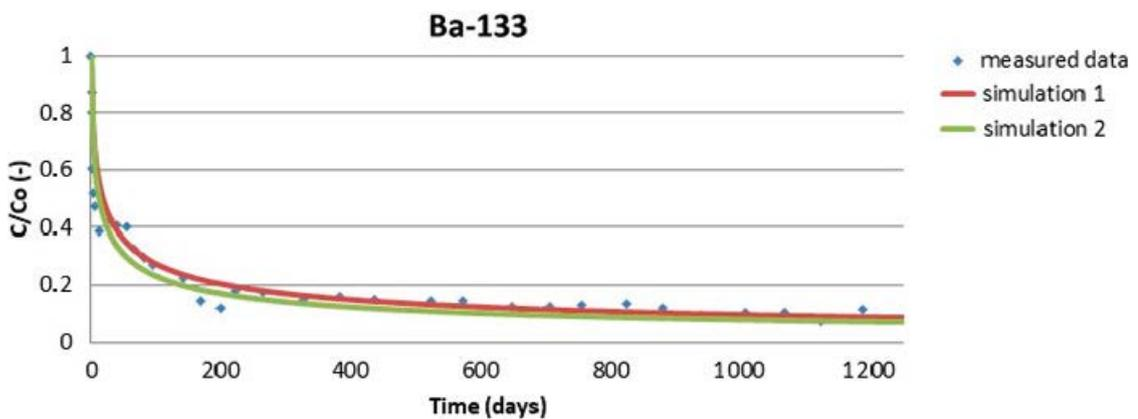
Figure 6-42. Agreement between the measured and model results for different combinations of model parameters, development of activity in the injection borehole.
