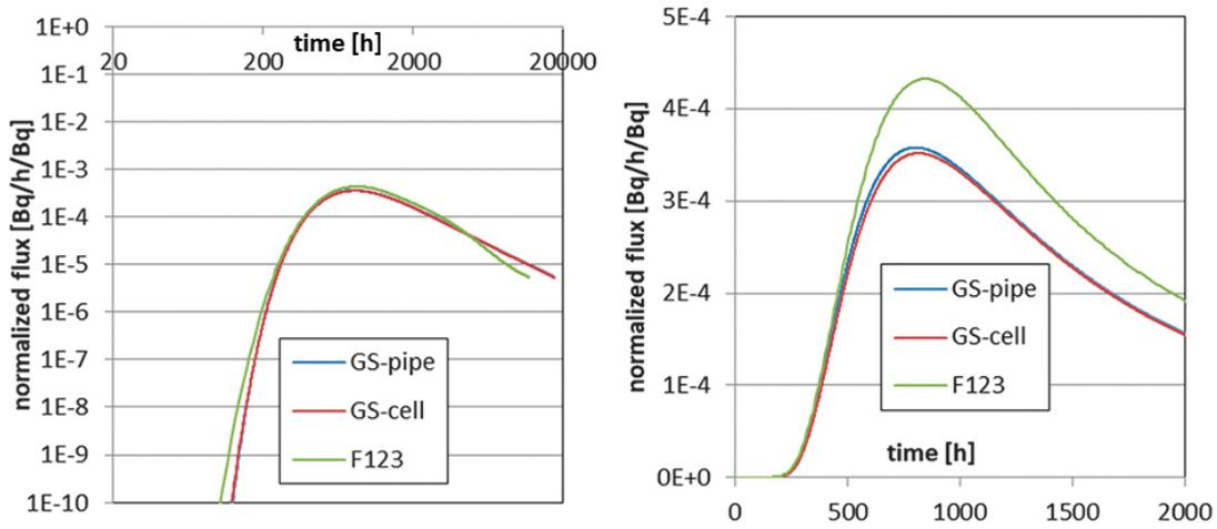
Figure 3-13. Comparison of the calculated breakthrough curves of WPDE-2 by individual models for Na-22.
