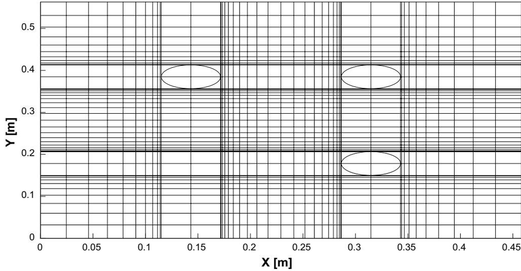
**Figure 6-7.** Planar 2D grid in GoldSim for Task 9C.
