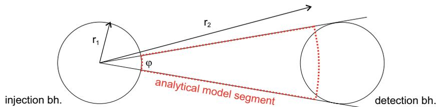
**Figure 6-50.** Geometry for the steady-state radial symmetric model of TDE experiment – determining angle for ratio of mass captured by detection boreholes.
