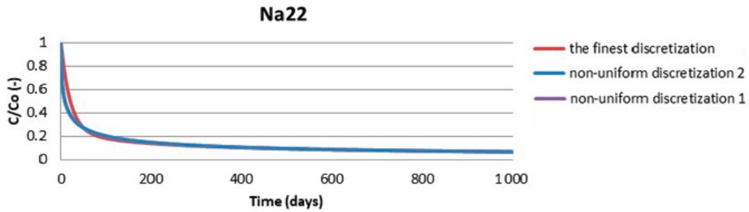
**Figure 6-15.** Detail of the development of Na-22 activity in the injection borehole according to the ÚJV-GoldSim model – comparison of uniform and non-uniform division of the model area, curves for the non-uniform division of the area overlap.
