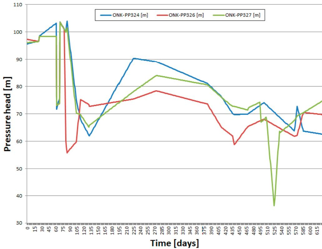
Figure 6-21. Task 9C – Flow123d – influence of pressure gradient – measured pressure gradient – development of boundary conditions of flow dependence of the relative activity on time in the monitoring boreholes.
