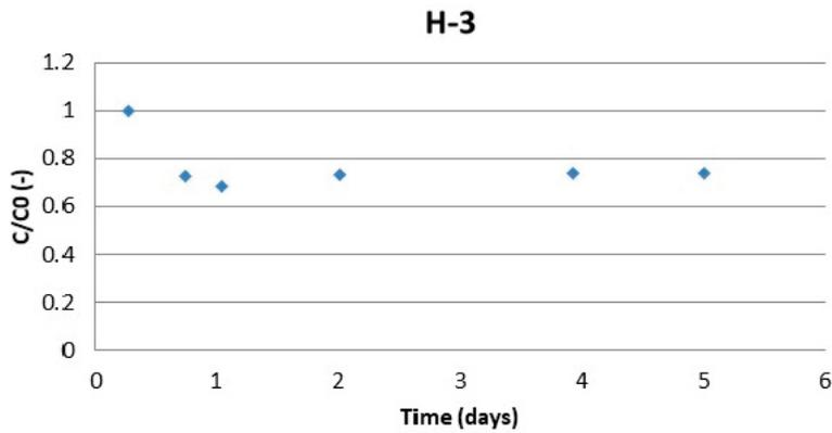
Figure 6-32. Original measurement data, steep decrease during the first day attributed to the setup of the experiment.
