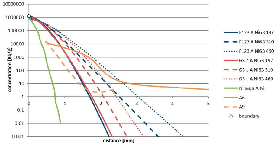
**Figure 4-8.** Comparison of profiles of Ni-63 calculated by Flow123d, GoldSim (Cell Net) for Type A and times 197 d, 310 d and 460 d, versus the measurement of profiles A6 and A9 and the original calculation in Nilsson et al. (2010).
