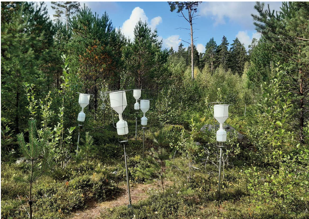
Figure 4-3. Precipitation sampler setup of six funnel-shaped polyethylene containers (summer type) at new location PFM008126.
