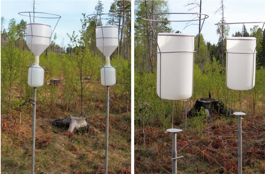
Figure 4-2. Precipitation samplers: two summer setups (to the left) and two winter setups (to the right) at location PFM002564.
