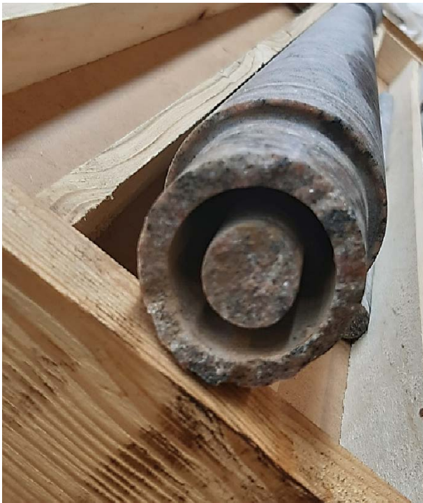
Figure 5-3. First overcore test with the pilot core still attached in the bottom end. Only the first short part has thinner walls until the special overcoring crown is used. The thickness of the hollow core walls is about 12 mm. The rock type of the core is (101057).
