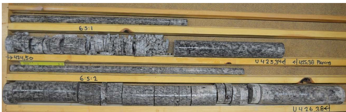
Figure 5-8. Deepest drilled overcore (6:5:2) in KFM07C down to 426.38 meters borehole depth. Example of more pale 101057, presumably more towards “granodioritic” composition and/or more albitized with little or total absence of potassium feldspar.
