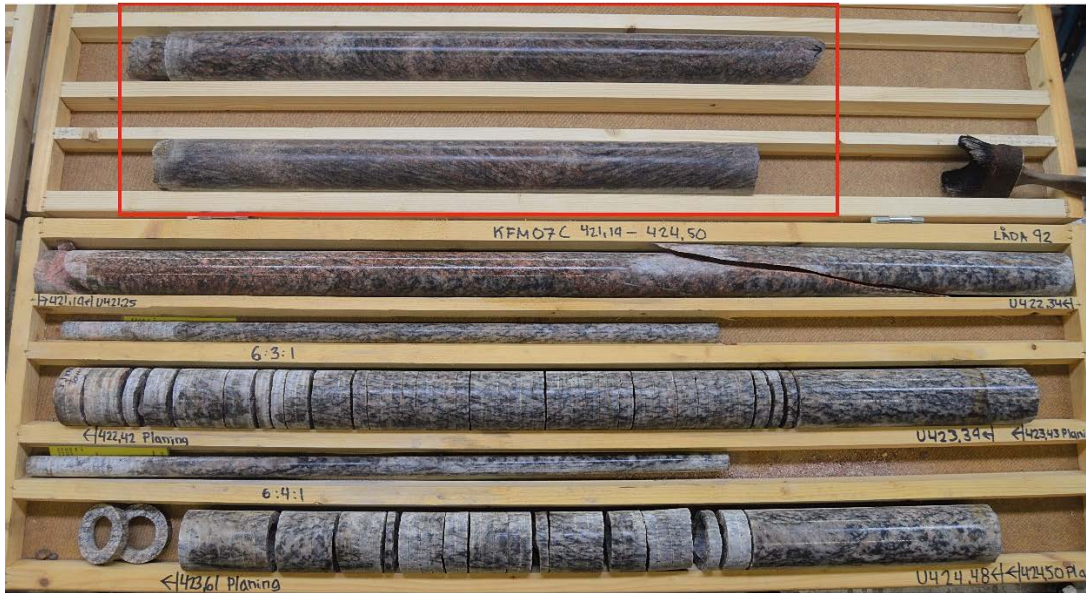
Figure 5-9. For comparison the image shows overcores from KFM24 (red box) and overcores (6:3:1 and 6:4:1) from KFM07C below. Note the ring disking and the pale colour of 101057 in both overcores from KFM07C.
