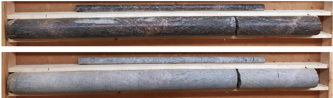
Figure 5-7. Wet (up) and dry (down) pictures of overcore 2 and pilot core 2. The two open fractures in the bottom are induced as a consequence of taking the core out. Shifting of foliation is visible.
