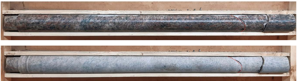
Figure 5-4. Wet (up) and dry (down) pictures of overcore 1. The open fracture with minor chlorite is marked with a dashed red line, the second fracture at the bottom is induced as a consequence of taking the core out.
