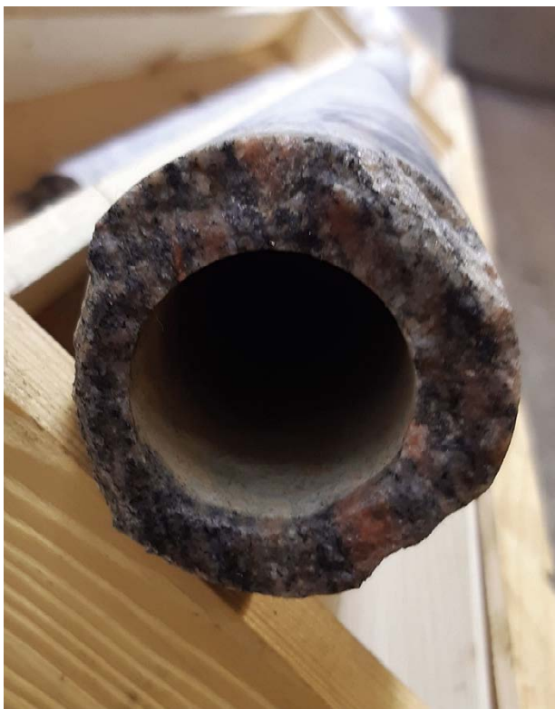
Figure 5-6. The pilot hole of overcore no. 2 was not fully centered. Wall thickness of thinnest part is ~10 mm (to the left) and ~15 mm on the thicker side to the right. The foliation is well visible.
