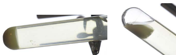
Figure A-4. Behaviour of sediment in #3 after tilting.
