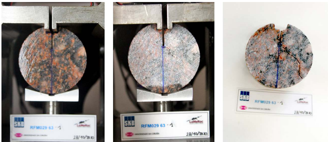
Figure A2-17. Sample 101057 63-1 before (left) and after (middle and right) conducting a pCT test. The K_{IC} value obtained was of 1.38 \text{ MPa m}^{1/2} obtained for a maximum load of 1.49 kN.
