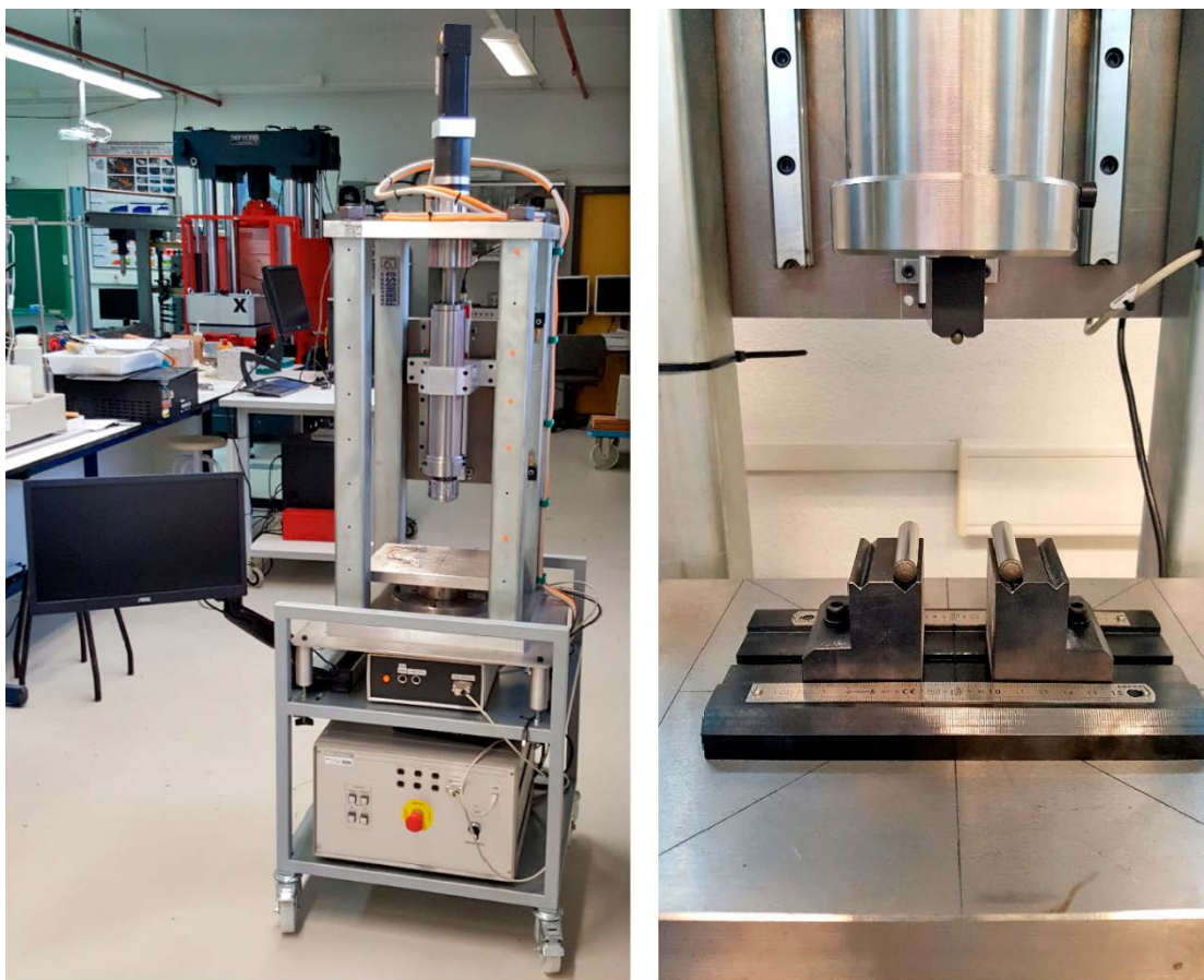
Figure 2-2. General view of the test frame used to conduct the SCB tests (left) and detail of the testing fixture (right).
