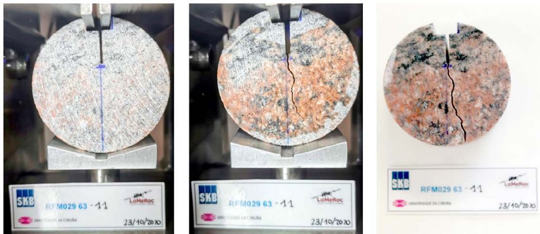
Figure A2-28. Sample 101057 63-11 before (left) and after (middle and right) conducting a pCT test. The K_{IC} value obtained was of 1.84 \text{ MPa m}^{1/2} obtained for a maximum load of 1.94 \text{ kN} .
