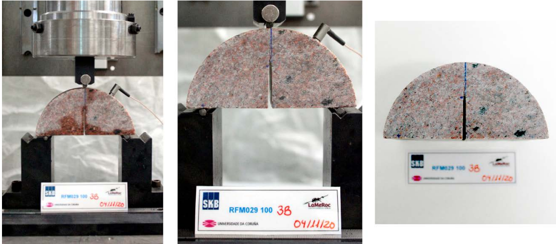
Figure A2-9. Sample 101057 100-3b before (left) and after (middle and right) conducting a SCB test. The KIC value obtained was of 1.36 MPa m 1/2 obtained for a maximum load of 3.13 kN.
