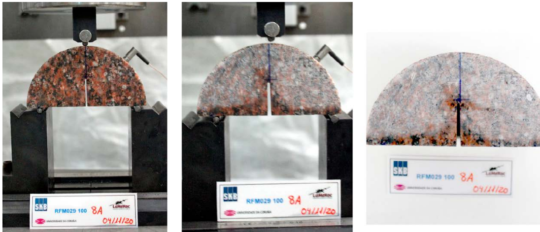
Figure A2-12. Sample RFM029 100-8a before (left) and after (middle and right) conducting a SCB test. The K_{IC} value obtained was of 1.99 \text{ MPa m}^{1/2} obtained for a maximum load of 4.07 kN.
