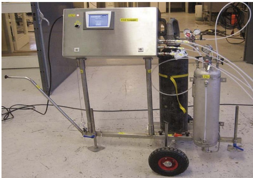
Figure 3-7. Equipment for injection of water/tracer.
