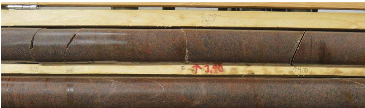
Figure 4-4. Core box photo showing the core from Bh2 and the Ävrö granodiorite with two subparallel fractures at 3.5–3.7 m, see also Figure 4-5.
