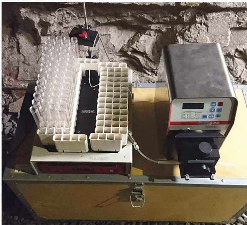
Figure 3-9. Sampling equipment, sampling changer and peristaltic pump.
