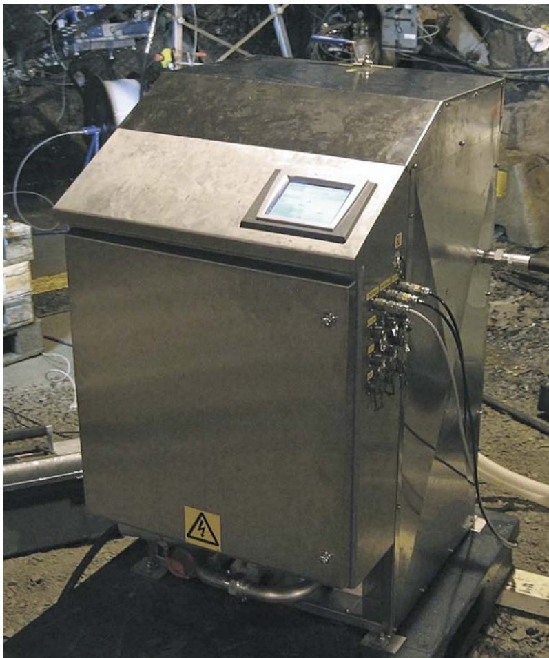
Figure 3-2. High pressure Water Injection Controller (HWIC).
