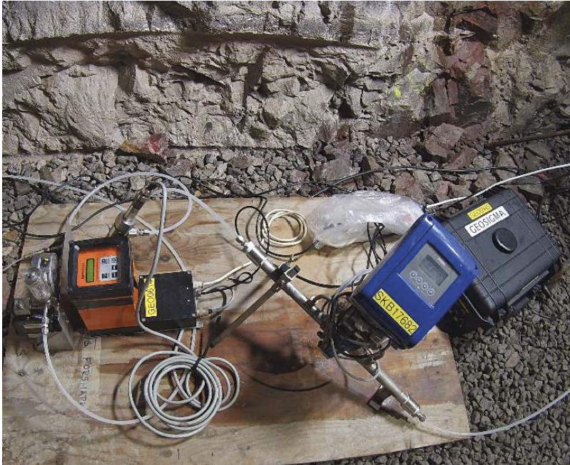
Figure 3-8. Equipment for measurements of EC and flow and data logger.
