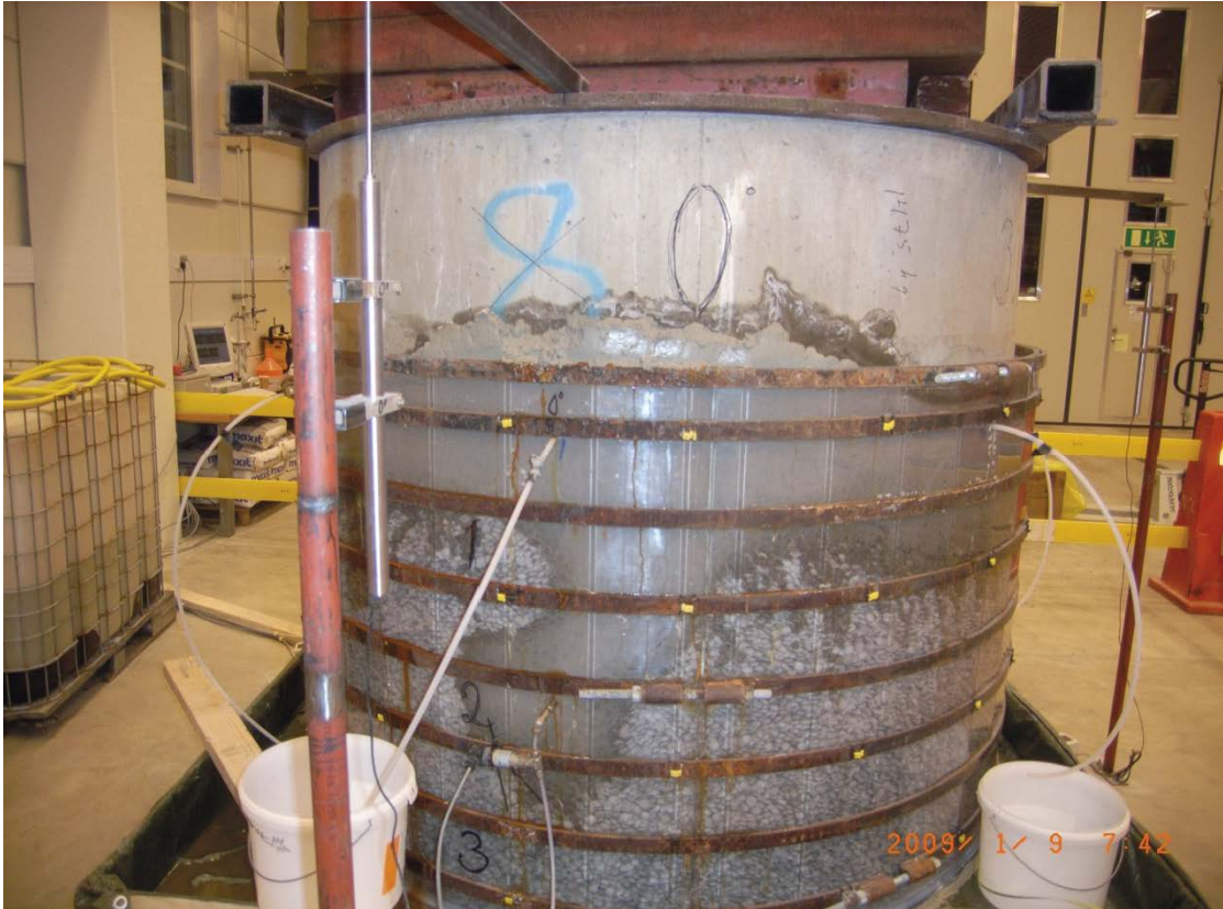
Figure 3-6. Picture The wetting pattern for an inflow of 0.001 l/min. the water initially goes upwards until it reaches the top surface and the water starts to spread over the top surface. The picture is taken approximately 40 days after the test was started.
