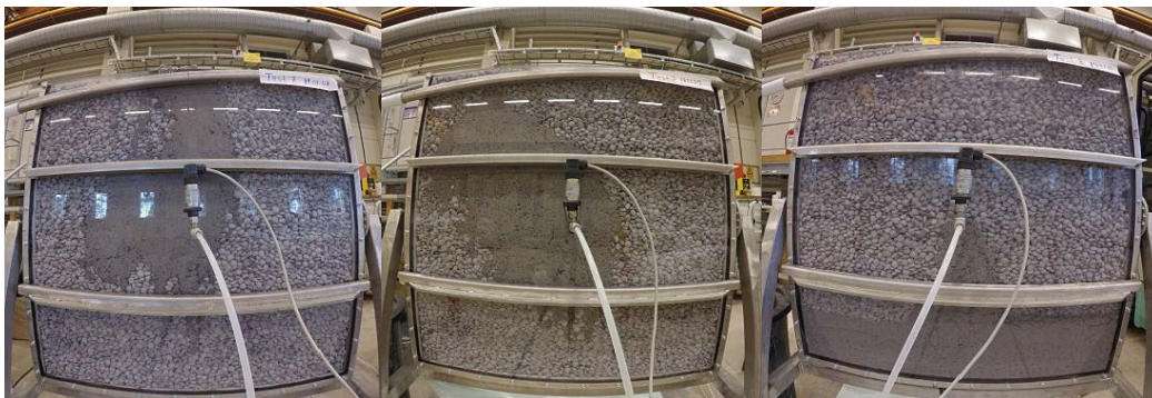
Figure 3-9. Wetting patterns for three different inflows 0.001 l/min, 0.01 l/min and 0.1 l/min. The lowest inflow to the left and the highest inflow to the right.
