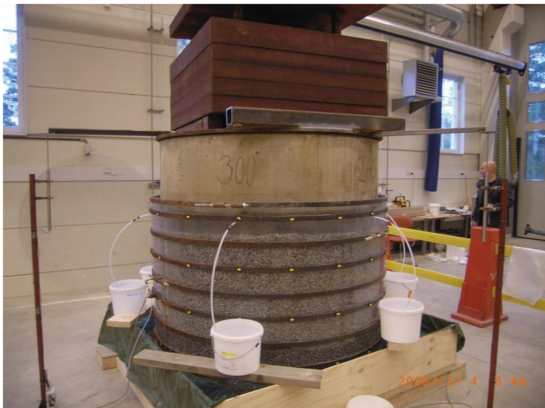
Figure 3-4. Picture showing the setup. Two buffer blocks with pellet filled slot around with 10 ton of weight on top. The hoses in the top of the container are drainage pipes and the inflow point is seen to the left.
