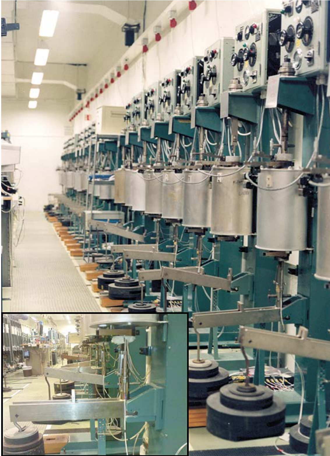
Figure 3-4. Creep testing laboratory showing the creep rigs. Inset: a close-up of the lever arm.
