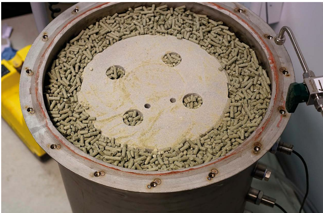
Figure 2-5. Test container filled with bentonite blocks and surrounding pellets.
