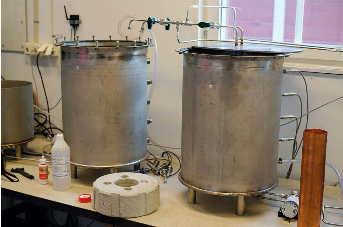
Figure 2-2. Two stainless steel containers equipped with sensors for temperature and relative humidity (RH) and connections for online analysis of gas composition.
