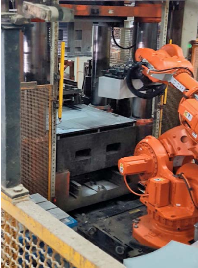
Figure 2-4. The industrial robot grabbing a finished block from the SACMI press.
