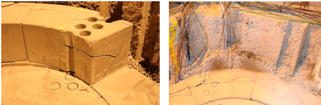
Figure 3-27. Left: Block from layer C12. Right: Sampling of pellets in layer C12.
