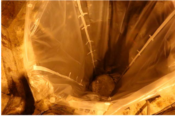
Figure 3-3. Plastic tube attached to the aluminium plate in the bottom of the test hole.
