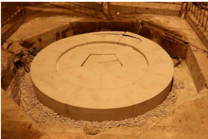
Figure 3-26. Layer C14 after removal of the protection lid. Note that the top surface was even when the test started.
