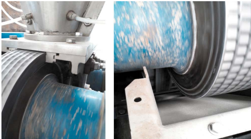
Figure 2-9. The press used for producing pellets, a) the filling of the bentonite between the two wheels and b) the perforating of the wheel filled with compacted bentonite.
