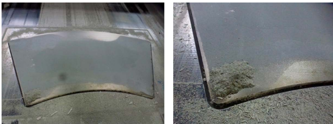
Figure 2-8. Bottom mould plate with material that got stuck.
