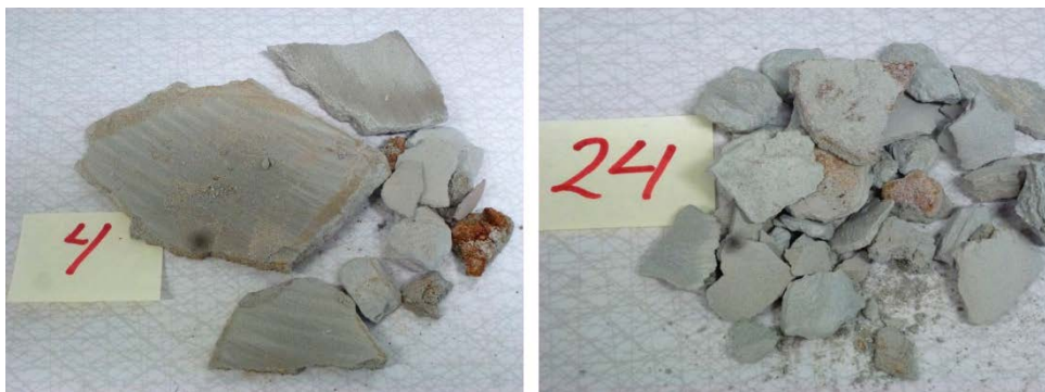
Figure 2-6. Bentonite lumps found during production.
