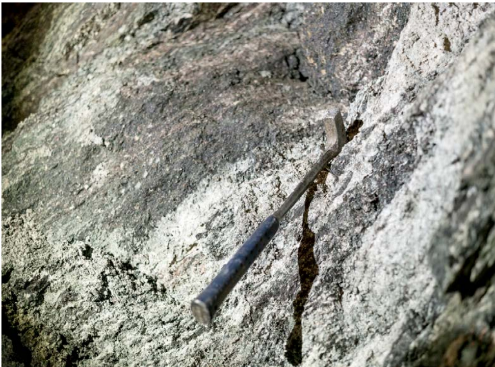
Figure 5-3. Naturally present smectite at -1100 m level in the Kiruna mine. These swelling clay minerals are very similar to bentonite and this location is very promising for a natural analogue study.
