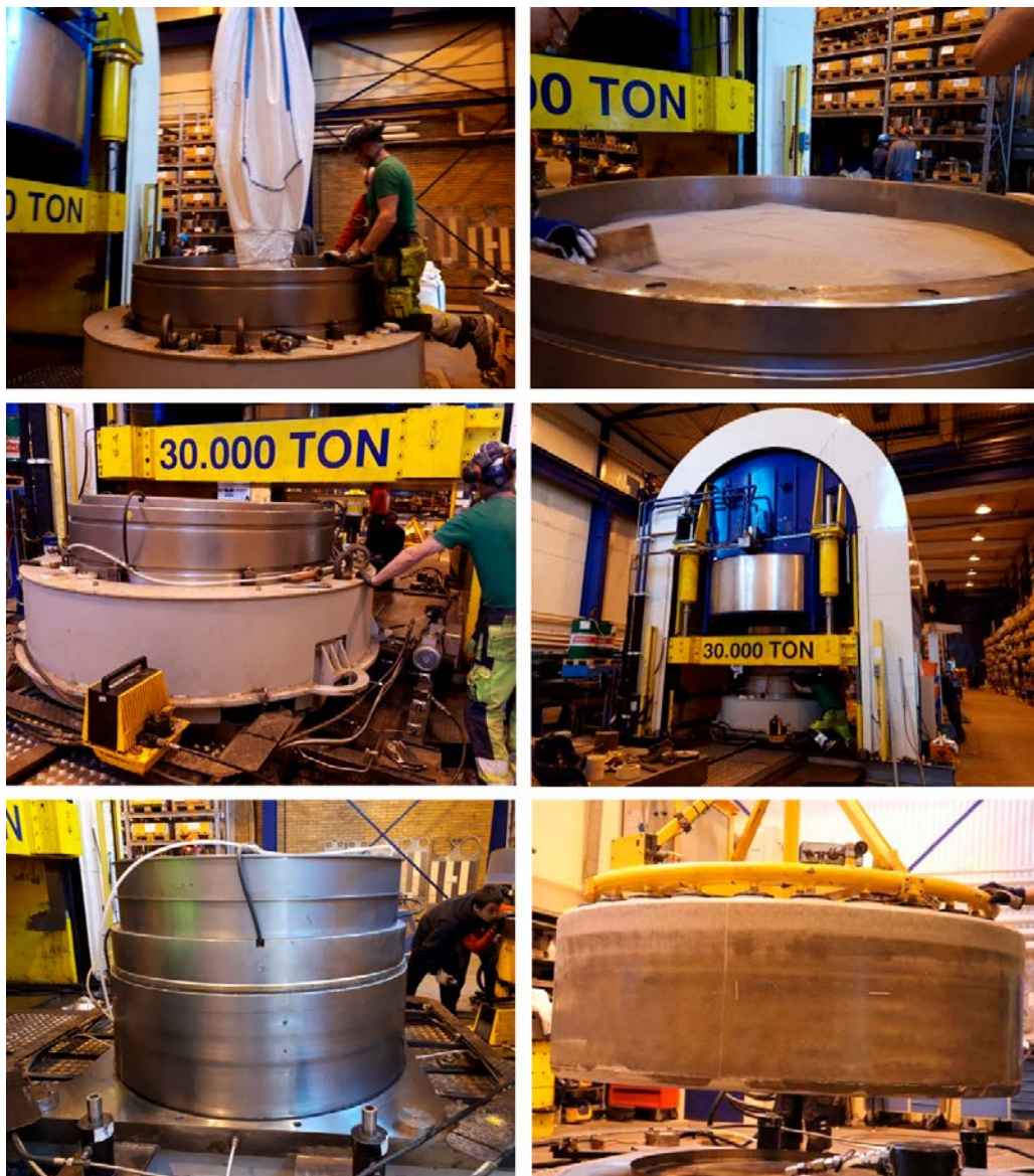
Figure 3-20. The production of the bentonite blocks.
