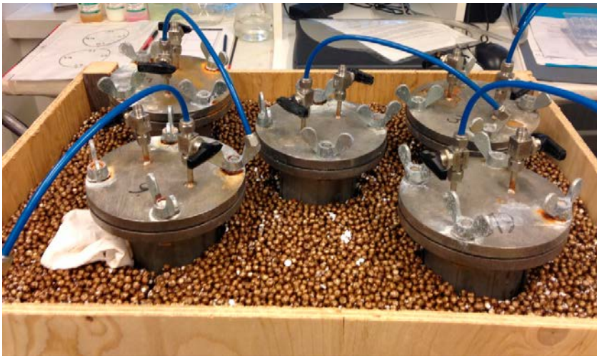
Figure 3-26. Steel containers placed in the transport box.
