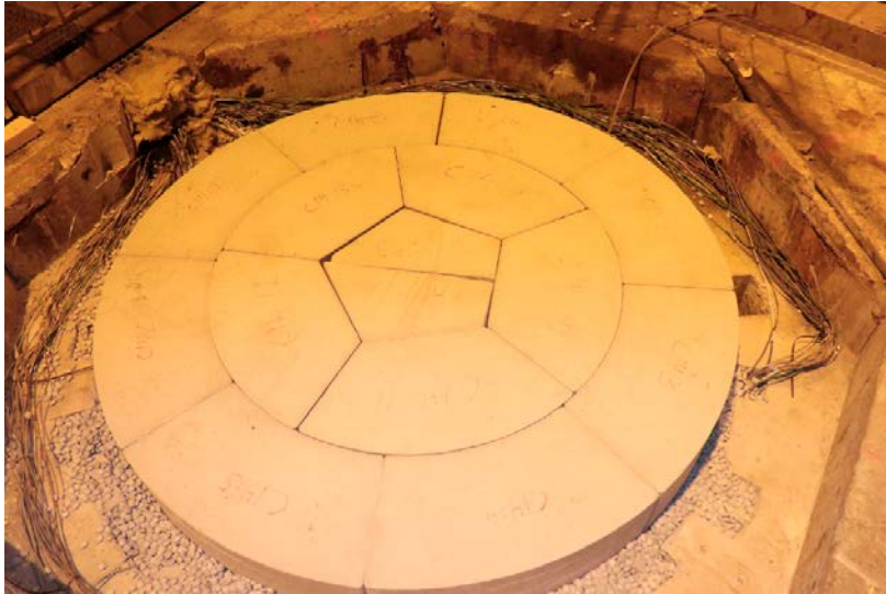
Figure 3-9. Test after completed buffer installation but before placement of the lid.
