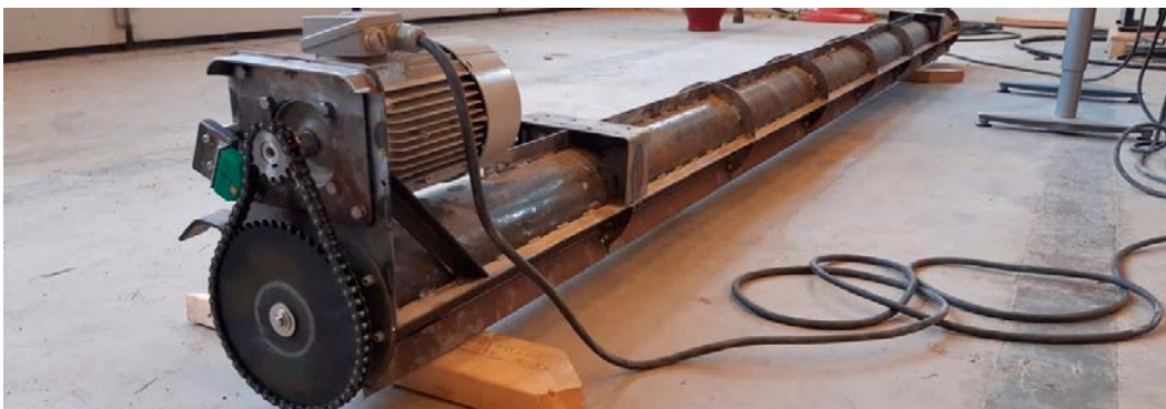
Figure 4-5. Equipment for installation of a pellet bed on the tunnel floor.
