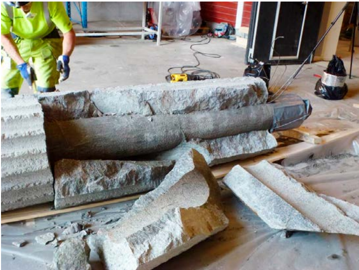
Figure 3-38. Large pieces of rock were removed from the test parcels and the bentonite exposed to allow for sampling.
