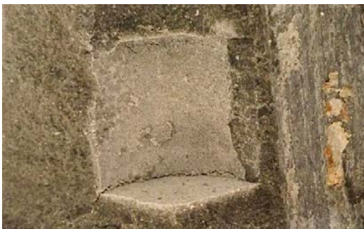
Figure 3-25. Image showing the interface zone where MX-80 bentonite had been in contact with a specimen made of standard cement paste.
