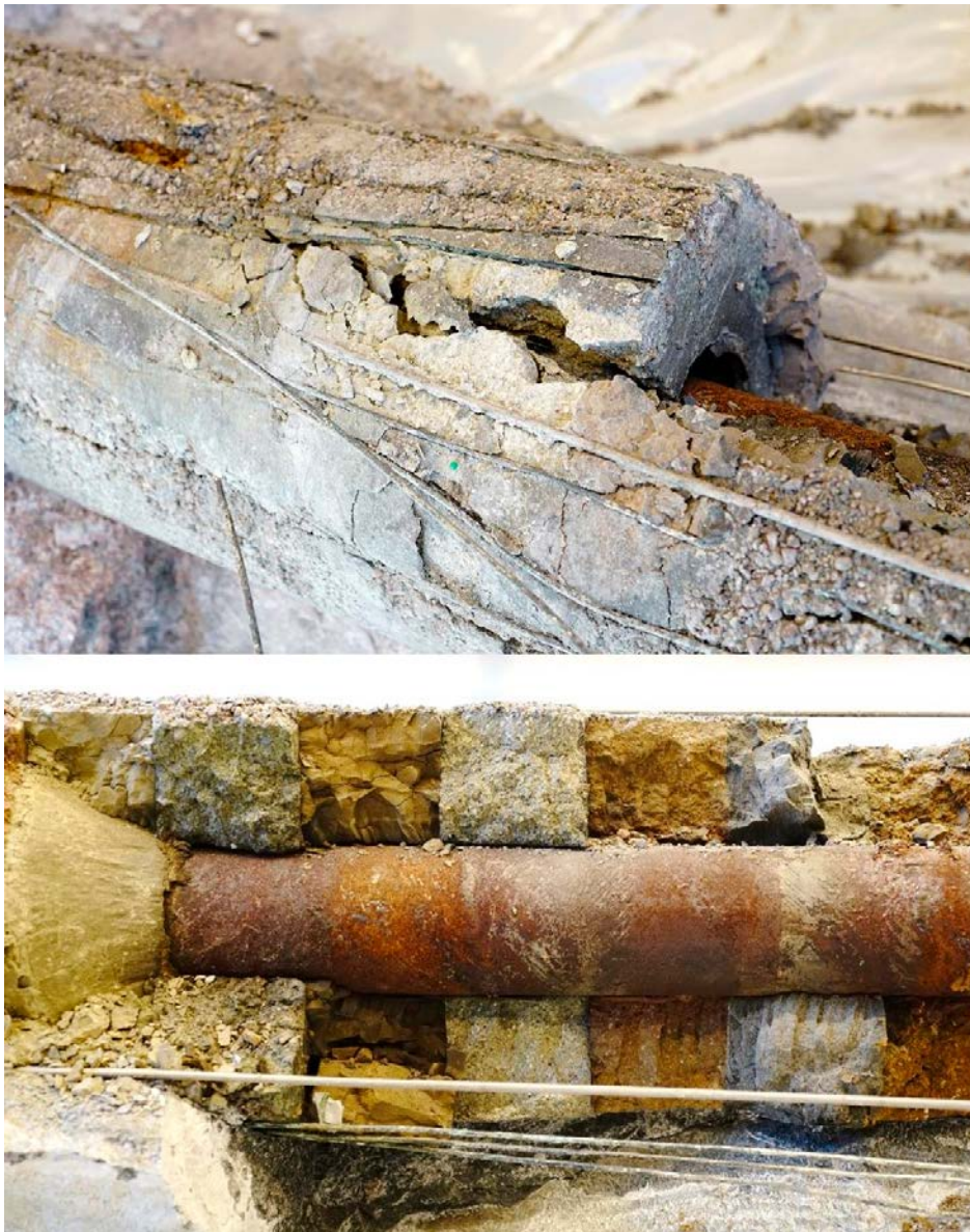
Figure 3-29. Highly fractured bentonite blocks from the very high temperature experiment ABM5 excavated in 2017.
