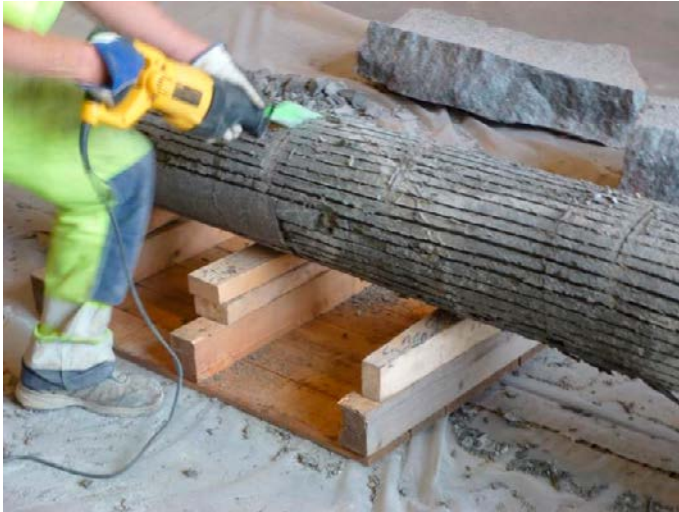
Figure 3-39. A saber saw was used to cut of blocks from the test parcel. The cuts were made approximately at the original block interfaces. The lines along the parcel that can be seen on the bentonite surface originate from thermocouples and other tubes that had been placed on the test parcel periphery (photo from test parcel A3).
