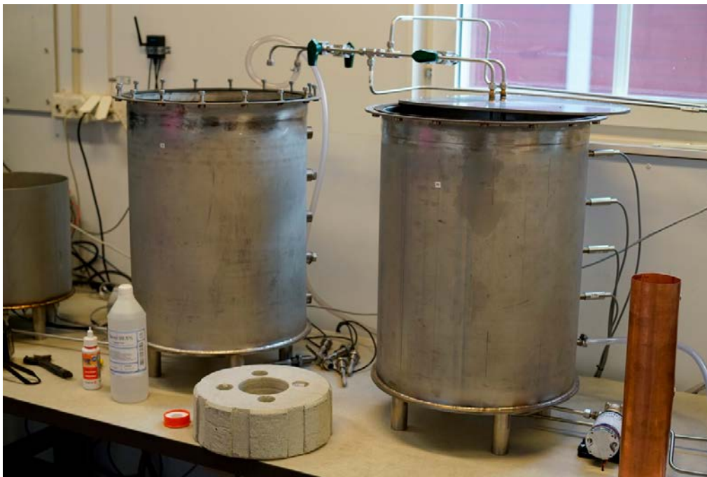
Figure 5-1. Deposition hole atmosphere test. Bentonite blocks, pellets and a copper heater are placed in a confined volume while oxygen, hydrogen and hydrogensulfide gases are monitored with time.
