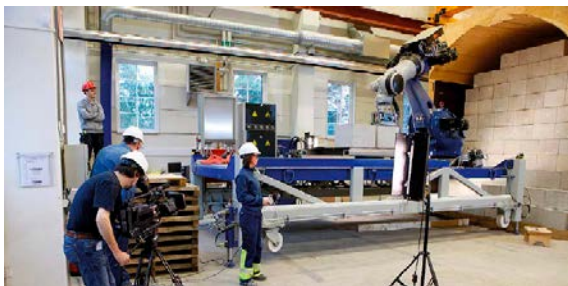
Figure 4-2. Robot stacking blocks in a full scale test in the Multipurpose test facility. Tests were also performed in the underground laboratory.
