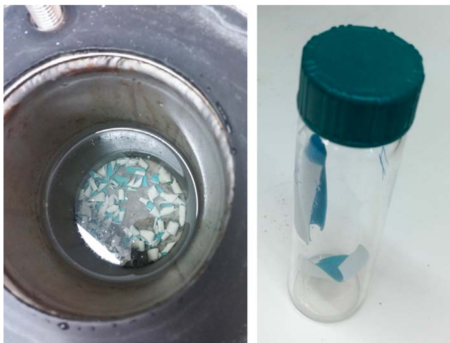
Figure 3-27. Top view of a container containing pieces of rubber gloves and the rubber pieces taken for solid state NMR measurements.
