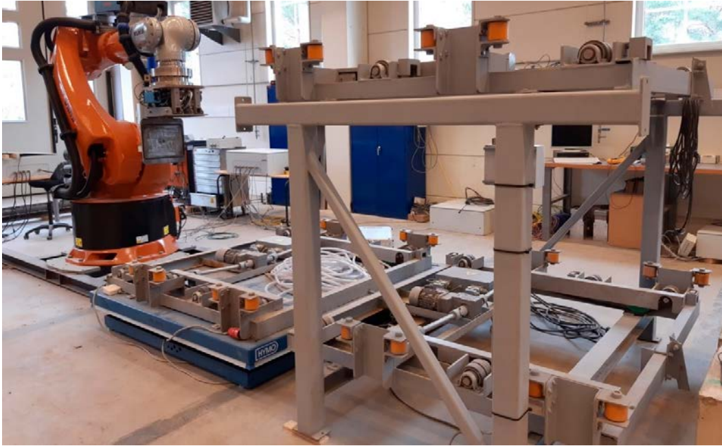
Figure 4-3. A smaller updated robot has been purchased in the project, software from the old one has been converted, and it is being tested together with transport equipment and pallets.
