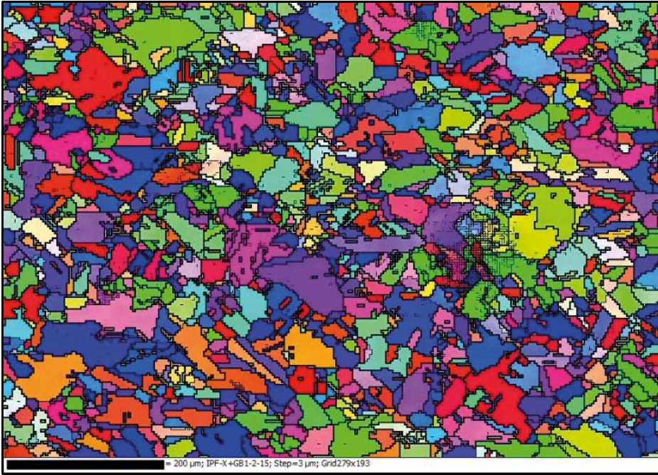
Figure 3-21. 250 °C, 6 months. The microstructure is completely recrystallized. Some deformation remained from specimen preparation. 200 μm scale bar.
