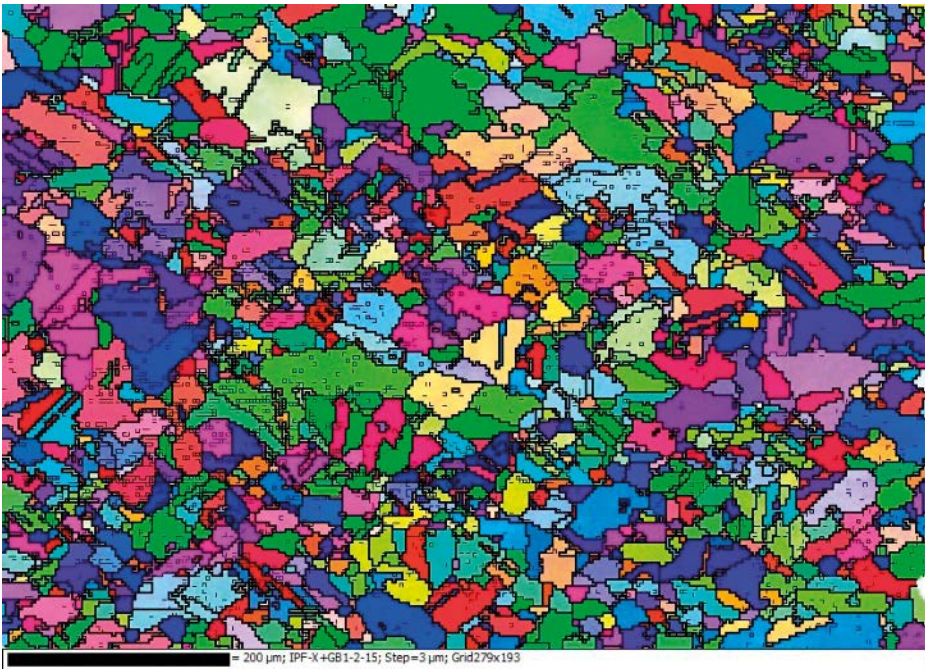
Figure 3-22. 250 °C, 12 months. Some deformation remained from specimen preparation. However, the specimen is completely recrystallized. 200 μm scale bar.
