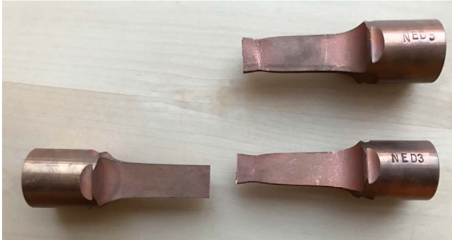
Figure 4-1. The type of creep test specimens the specimens for the Auger studies were taken from. These pieces were used for other purposes, but the necking region is clearly visible on the right hand parts. (Mannesson and Andersson-Östling 2014)
