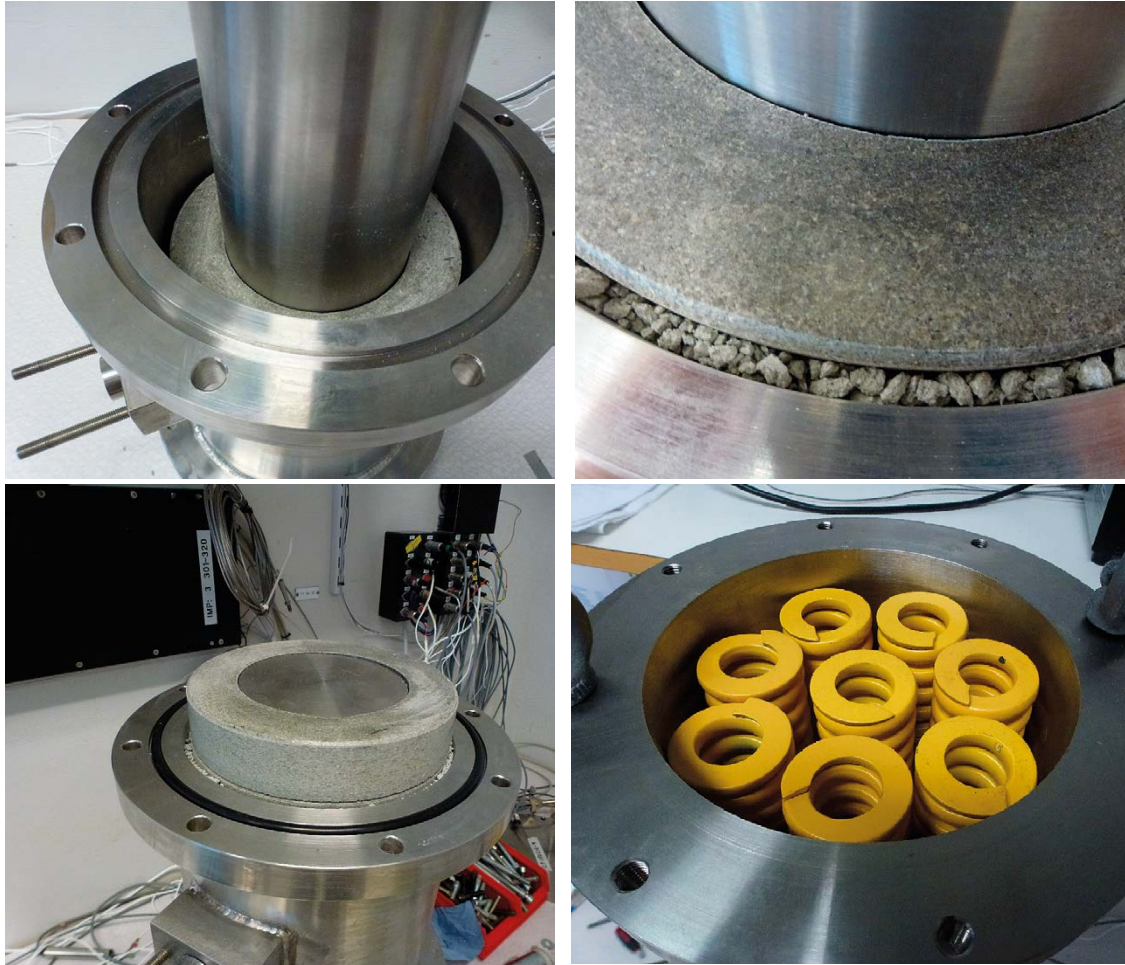
Figure 6-3. Photos taken during the assembling of the deposition hole tests. Upper left: The bottom block and the first two ring-shaped blocks are installed together with the canister. Upper right: Close-up showing the pellet filling between block and test cell wall. Lower left: The last ring-shape block is installed. Lower right: The springs installed at the top of the deposition hole. The springs simulate the resistance from the backfill during the buffer swelling.
