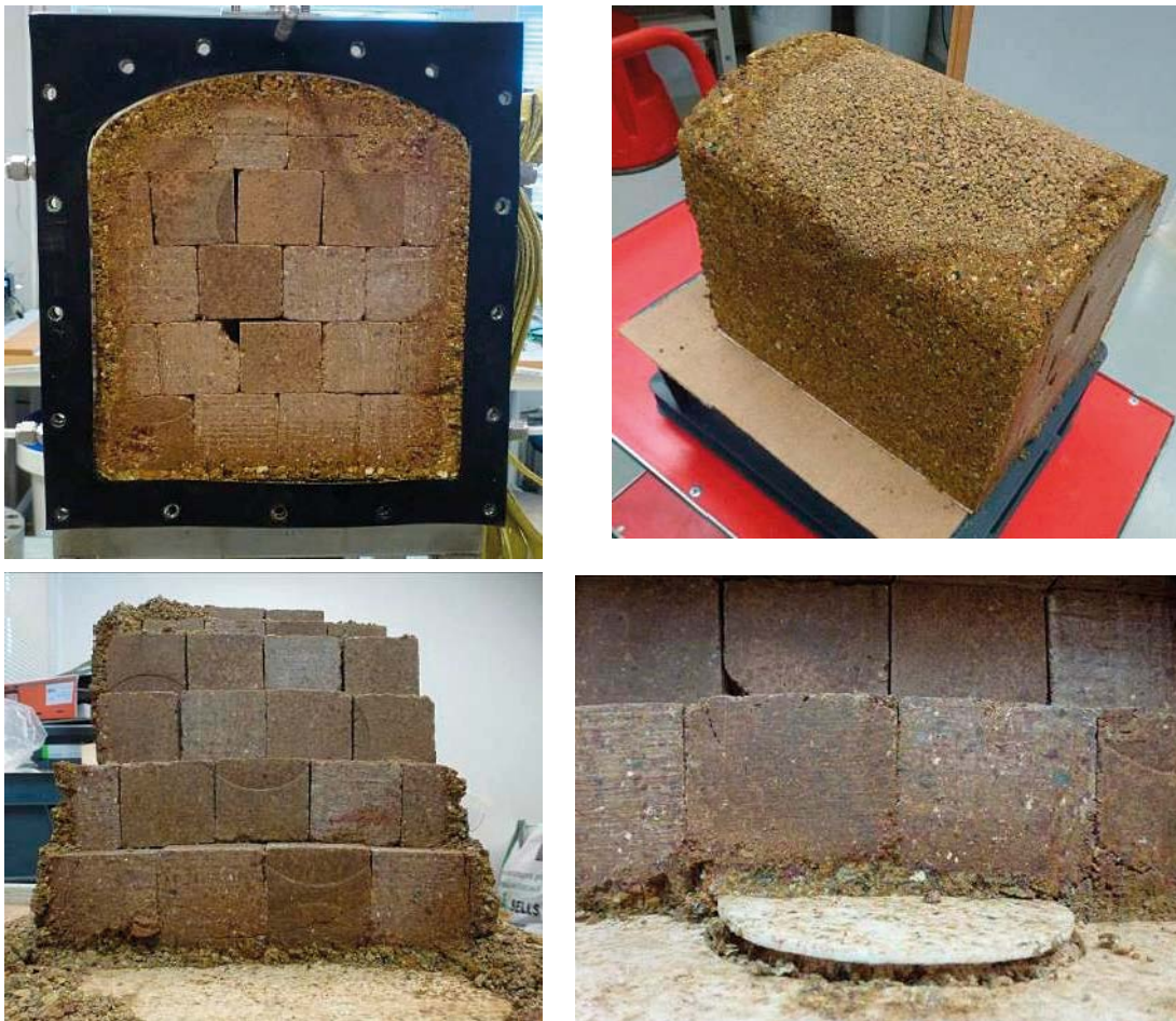
Figure 3-14. Upper left: It is mainly the pellet filling that has been affected by the limited water volume. Upper right: The complete backfill section has been removed from the steel tunnel. Lower left: The block stack is clearly affected of the simulated swelling buffer. Lower right: The top of the simulated deposition hole.
