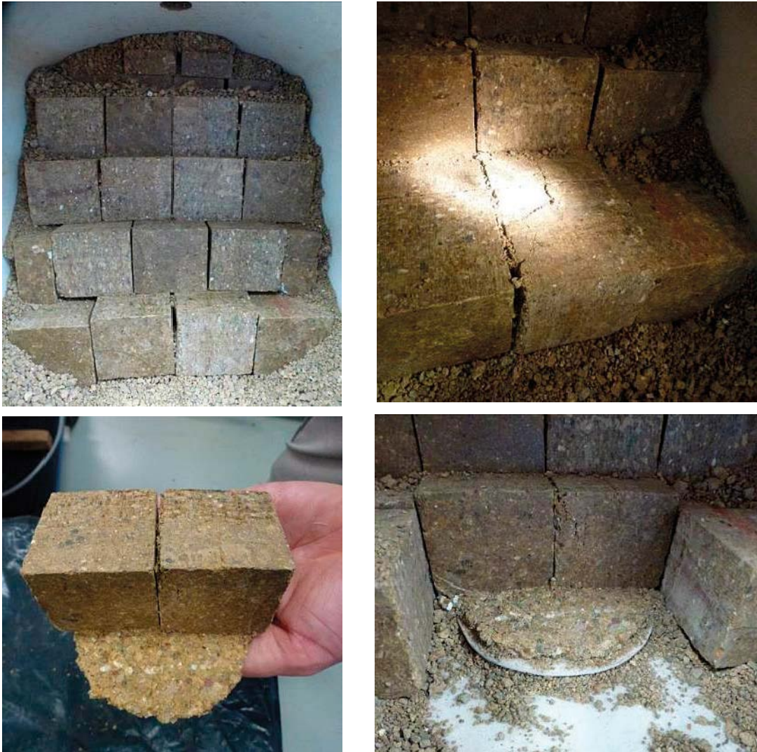
Figure 3-11. Upper left: The block stack is clearly affected of the simulated swelling buffer. Upper right: Some of the blocks close to the deposition hole had cracked. Lower left: The pellet filling on the floor had been compressed. Lower right: The top of the simulated deposition hole.
