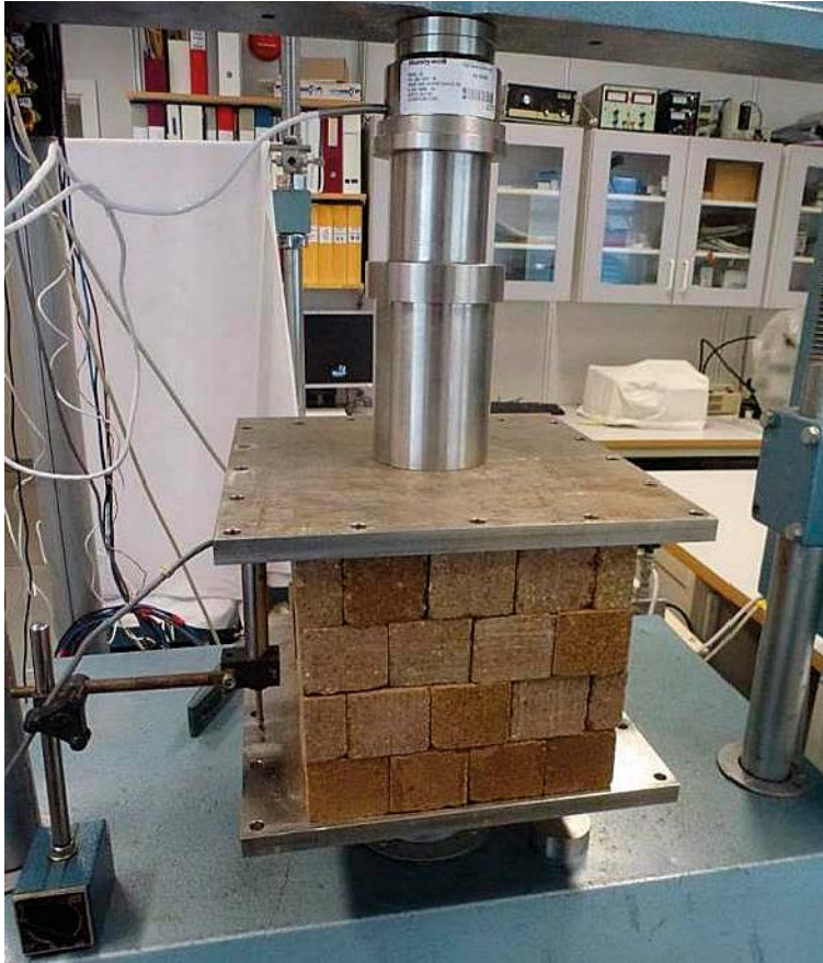
Figure 4-5. Photo showing the test setup for determining the compression properties of a block stack.
