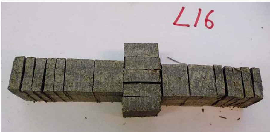
Figure 6-9. Samples were cut out from each of the sampling sections using a band saw.
