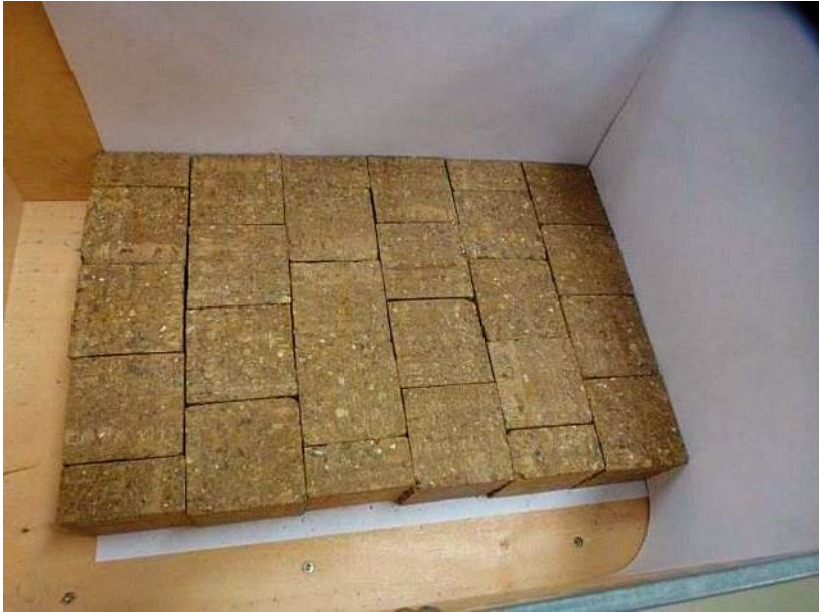
Figure 4-4. Backfill blocks were stacked in a corner of a rigid box.
