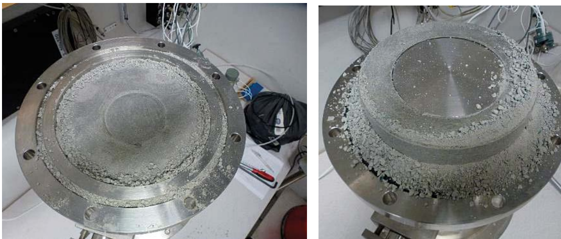
Figure 6-12. Left: The first cylindrical block above the canister, and the surrounding pellets, were visually unaffected of the wetting from the bottom of the deposition hole. Right: Photo showing the uppermost ring-shaped block. This block was also visually unaffected.
