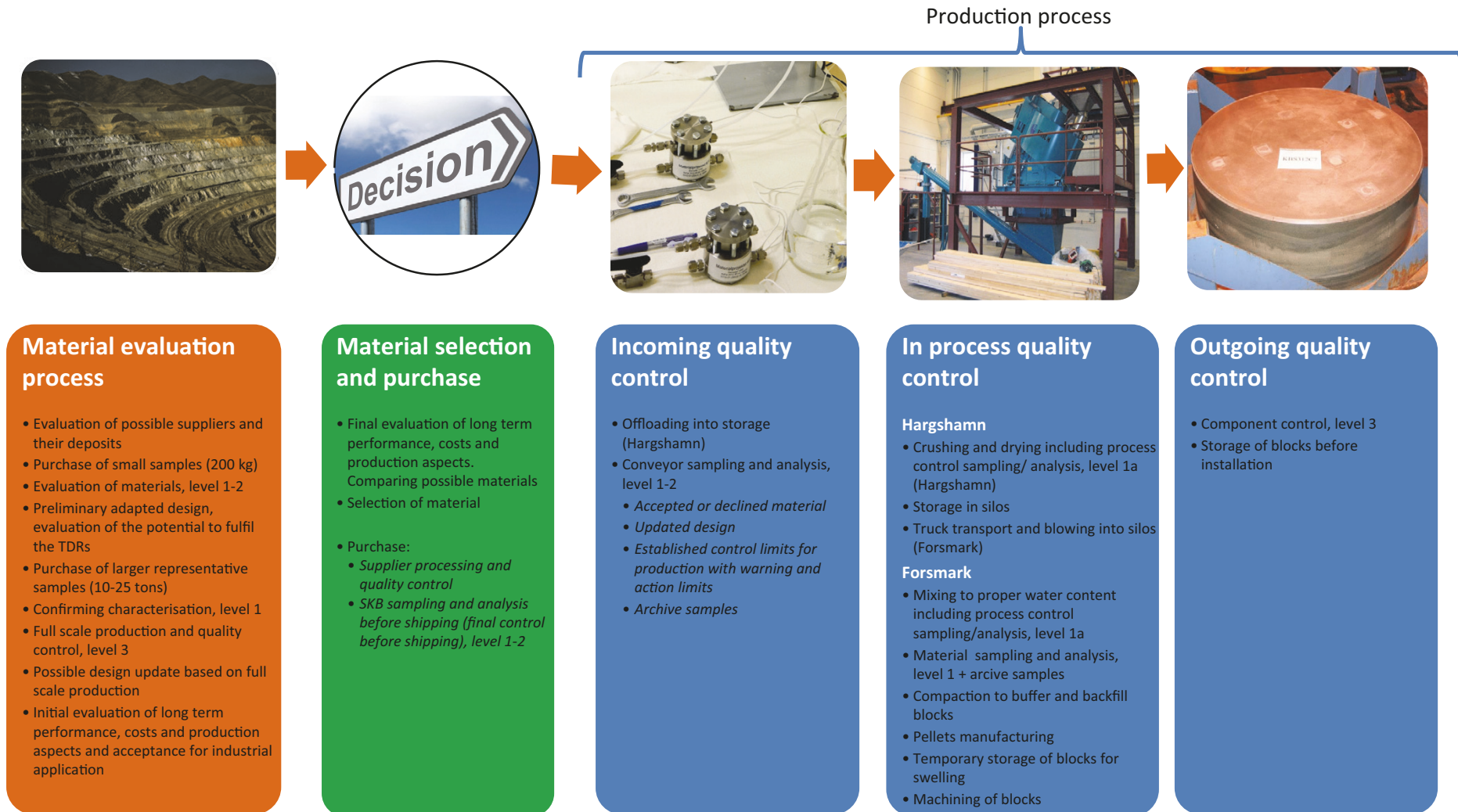
Figure 4-2. Division of the activities and quality control procedure into three main steps. For the referred analysis levels, see Section 5.3.
