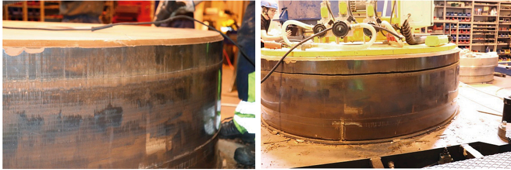
Figure 6-5. A block compacted with the bentonite India 2018 (Johannesson et al. 2020).
