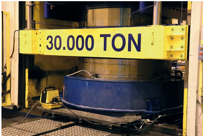
Figure 6-4. The mould placed in the press (Johannesson et al. 2020). For block manufacturing the press is limited to 10 000 tons.
