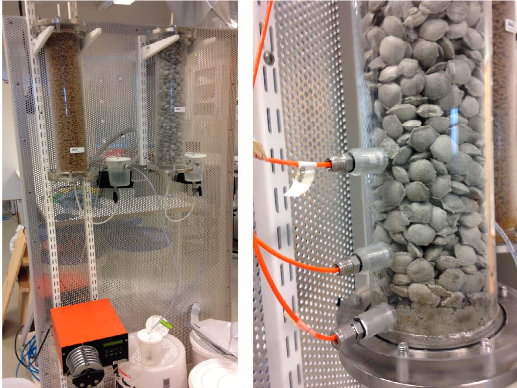
Figure 3-2. Test set-up for the water uptake tests (Test type A). Left photo: Extruded pellets in the left tube and roller compacted in the right tube. The peristaltic pump and the two external reservoirs can be seen beneath the test set-up. Right photo: Close up of the bottom part of a test with MX-80 pellets with installed RH-transducers.
