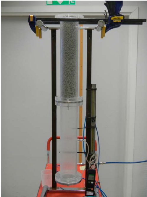
Figure 6-1. Test set up for the air permeability tests.
