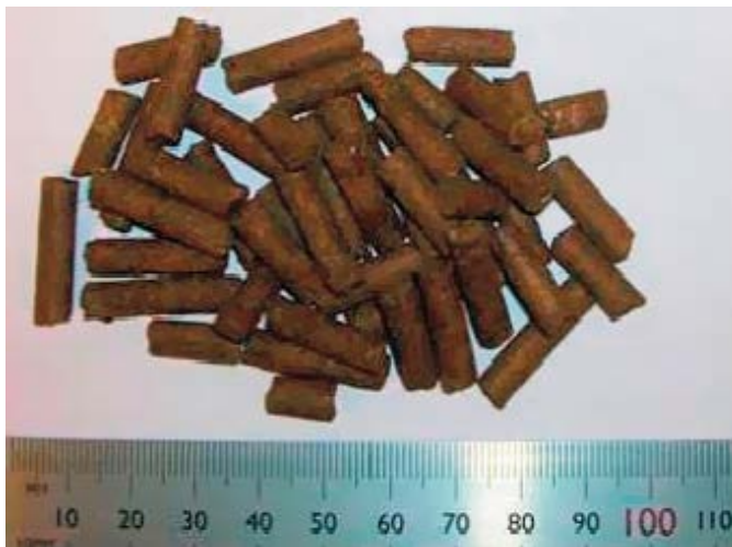
Figure 2-1. Extruded 6 mm rod shaped extruded pellets (Asha).
