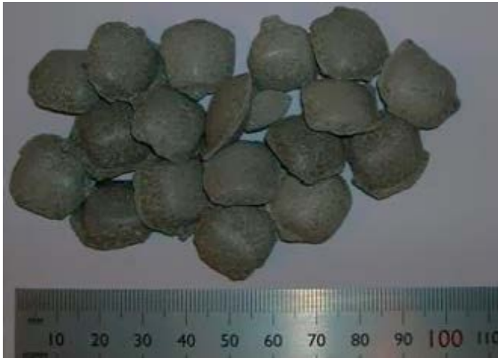
Figure 2-2. Compacted pillow shaped roller compacted pellets (MX-80-11).
