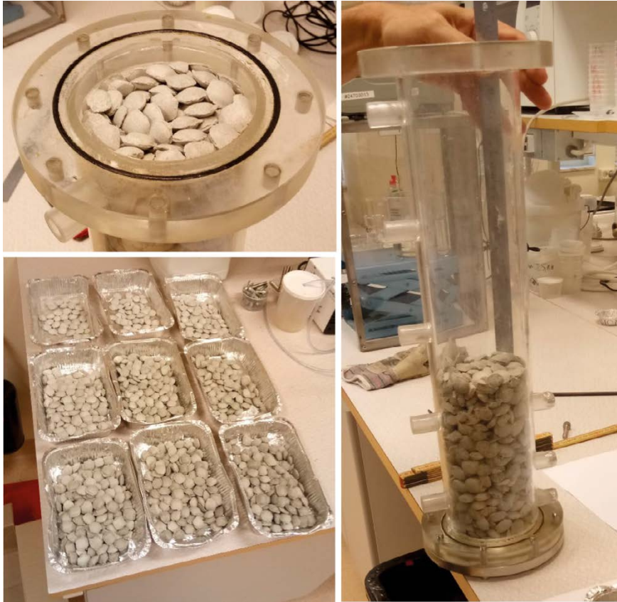
Figure 4-4. Sampling of pellets. Opening of lower end of test tube (upper left); removal of material down to a specified level (right); samples in aluminium containers (lower left).
