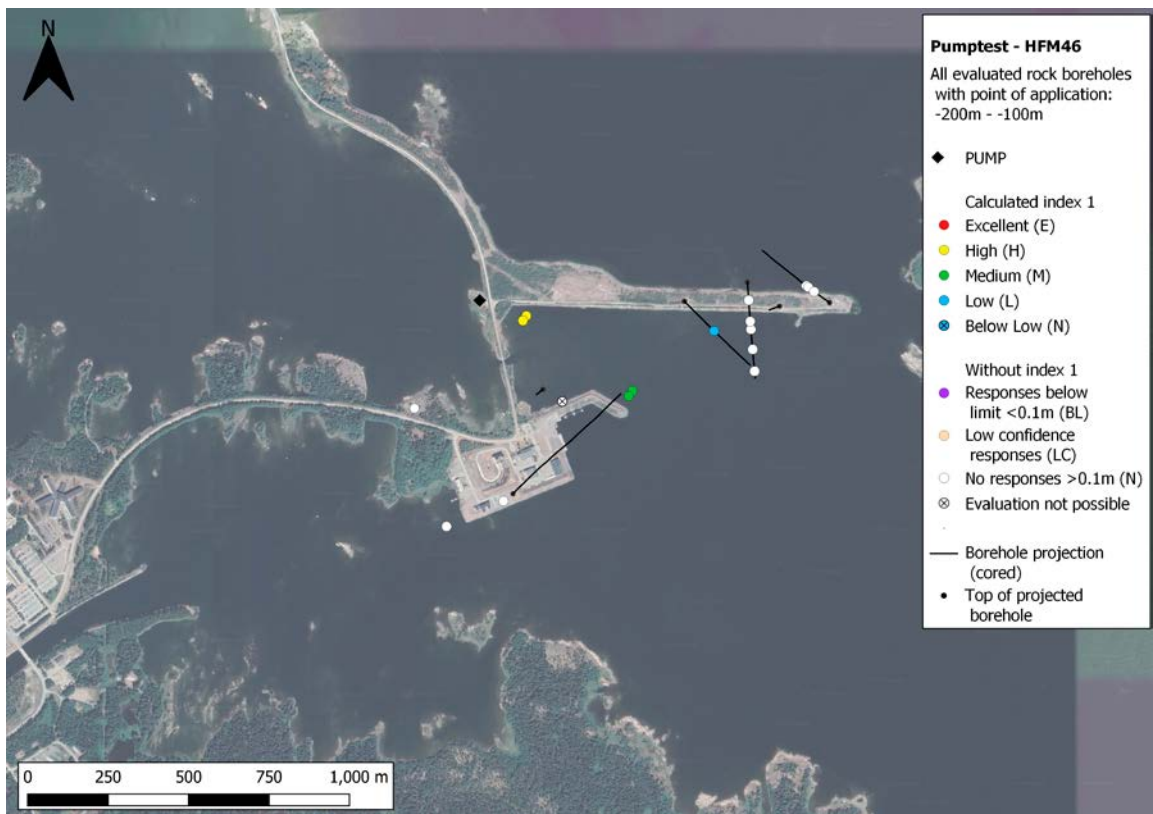
Figure A5-53. Calculated Index 1 from the interference tests in HFM46. All evaluated rock borehole sections with point of application of -200 to -100 m. Background map origin: Google maps.
