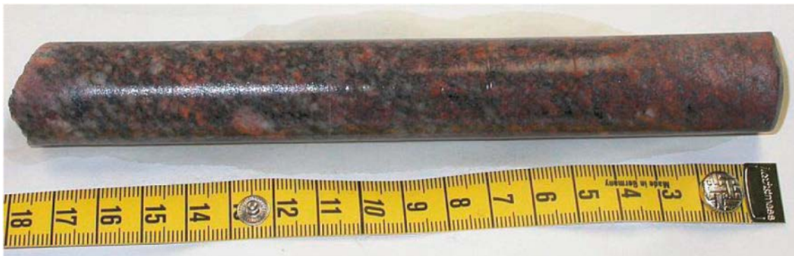
Figure 4-3. Photo of core sample A9, above a cm-ruler. The target fracture is on the right-hand side. Reproduced from Nilsson et al. (2010, Appendix 3).
