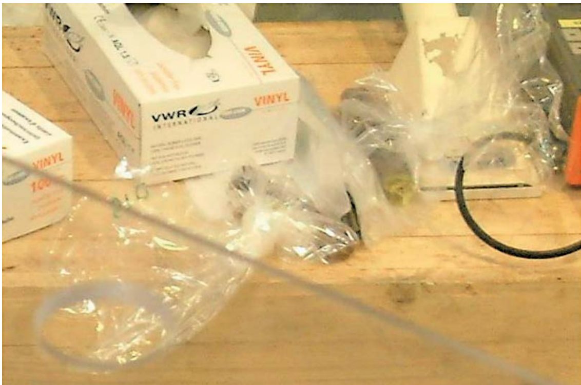
Figure A-1. Rock core samples contained in thin plastic bags, mainly to avoid cross-contamination during cutting, drilling and storage of rock core samples. Plastic bags were not primarily used to prevent drying of the pore water and air was not evacuated from them during storage.
