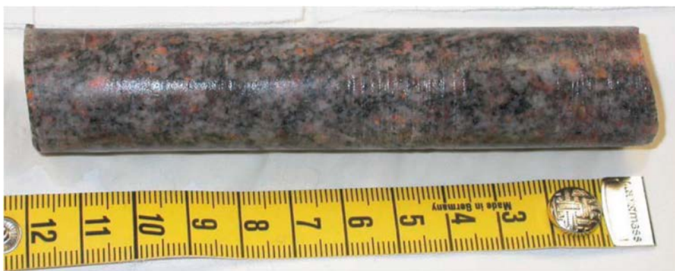
Figure 4-4. Photo of core sample D12, above a cm-ruler. The slim hole surface is on the right-hand side. Reproduced from Nilsson et al. (2010, Appendix 3)
