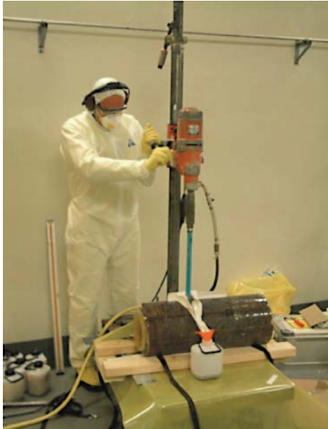
Figure 3-4. Drilling of core samples from the over-cored rock volume. This image also demonstrates the scale of the exposed rock volume in the experiment. Reproduced from Nilsson et al. (2010, Figure 2-4).
