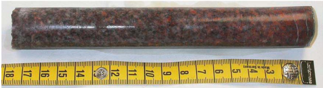
Figure 4-2. Photo of core sample A6, above a cm-ruler. The target fracture is on the right-hand side. Reproduced from Nilsson et al. (2010, Appendix 3).
