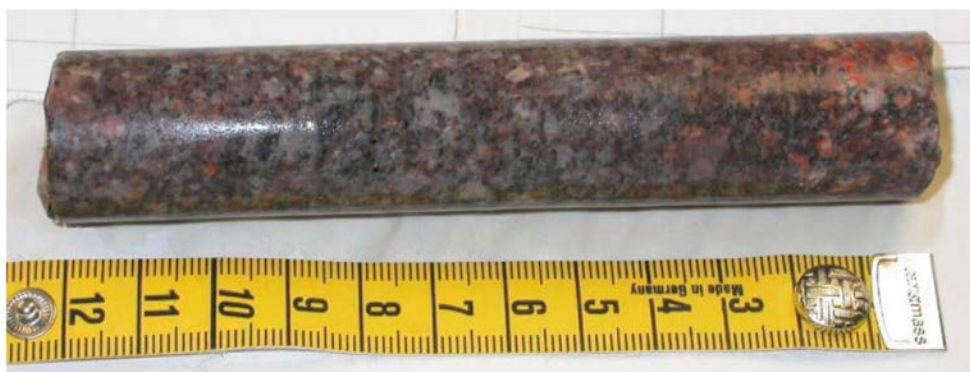
Figure 4-5. Photo of core sample D13, above a cm-ruler. The slim hole surface is on the right-hand side. Reproduced from Nilsson et al. (2010, Appendix 3).
