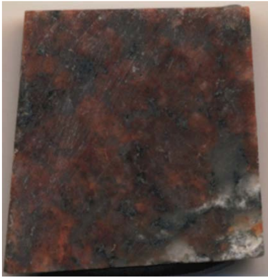
A11.1. Epoxy cover on the opposite side. Grain boundaries partly porous.
