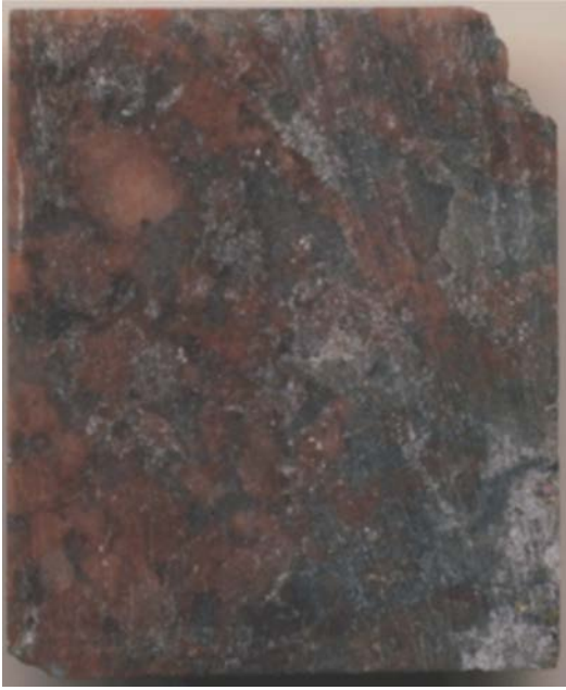
A4.1. The first rock slice is slightly irregular. Mainly consisting of fracture minerals (although the picture shows the opposite side, i.e. the wall rock side, fracture minerals are visible in the right lower corner), chiefly calcite and grains of chalcopyrite.
