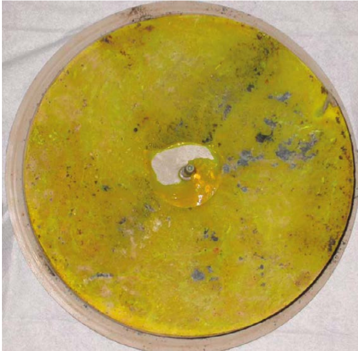
Figure 8-4. The epoxy resin adhering to the PEEK lid, protecting the fracture surface during overcoring. Reproduced from Nilsson et al. (2010, Figure 2-8).
