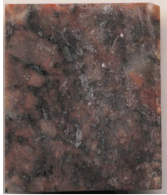
A4.2. Titanite is strongly altered, (weathered and decomposed).
