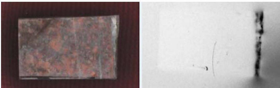
Figure 4-9. Autoradiograph of the first few centimetres of the cuboid sawn rock core A6, prior to further sawing into slices A6.1 to A6.9. The size of the rock sample is approximately 27×16 mm.
