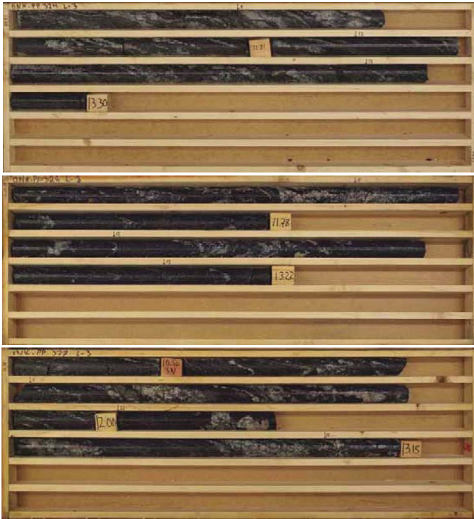
Figure 2-10. Photos of extracted drill cores of the lower parts of the TDE drillholes, where the tracer test is carried out. Upper photo = ONK-PP324, middle photo = ONK-PP326, and lower photo = ONK-PP327. The drill cores are wetted. Reproduced from Toropainen (2012).
