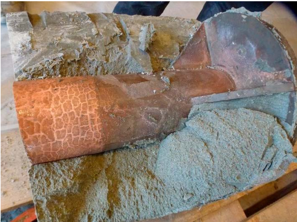
Figure 5-5. The bottom part of the central copper tube, including the bottom plate, was cut off together with three bentonite blocks (photo from test parcel S2).
