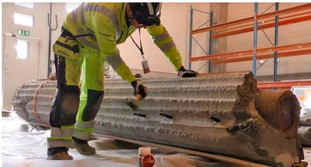
Figure 5-3. Photo showing the removal of the rock cover from the test parcels. Wedges were used to create fractures in the rock.
