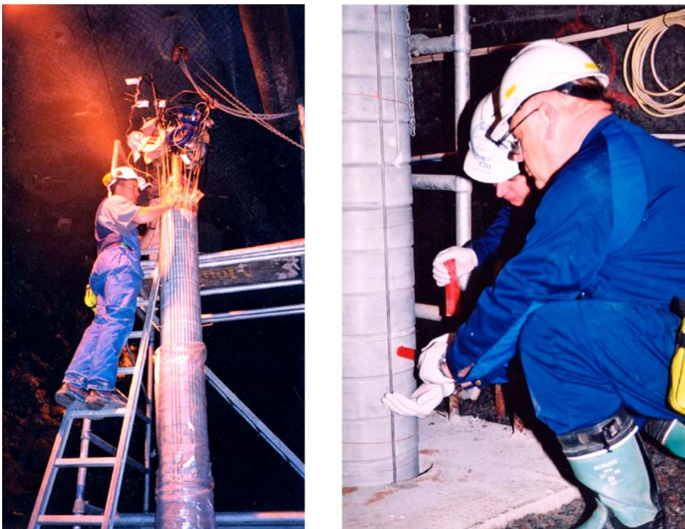
Figure 3-1. Left: Finalising the construction of a LOT test parcel at test site, note the large number of tubes from sensors. Right: Insertion of the plug containing ^{60}\text{Co} during lowering the parcel into the test hole. Note the lack of disturbing sensor tubing in the lower hot section.
