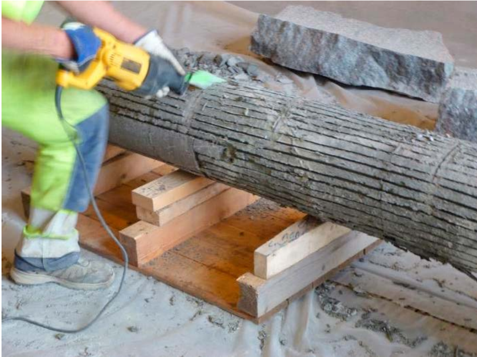
Figure 5-6. A saber saw was used to cut of blocks from the test parcel. The cuts were made approximately at the original block interfaces. The lines along the parcel that can be seen on the bentonite surface originate from thermocouples and other tubes that had been placed on the test parcel periphery (photo from test parcel A3).
