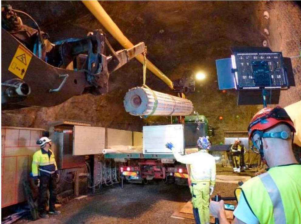
Figure 5-2. The entire test parcels, including rock-cover, were being placed on a lorry for transport to the ground surface.
