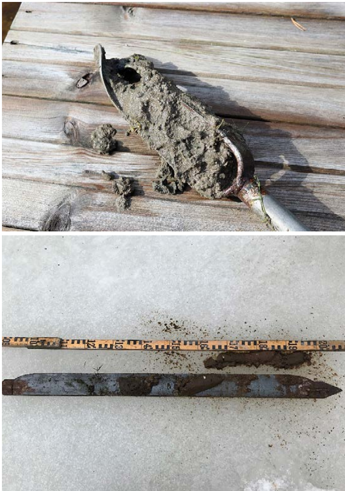
Figure 3-2. The hand driven probe (upper picture) and the Russian peat corer (lower) used for sampling.
