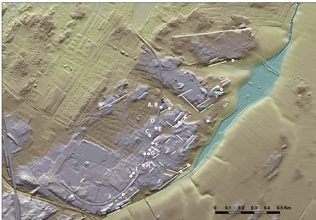
Figure 3-39. Major lineaments and interpreted fractures around Sandhem. Green dots indicate presence of a sub-horizontal fracture; white dots are sites where no significant sub-horizontal fractures are seen. These planar flats have local parallelism with sub-horizontal fractures but sheet structures are absent from the low cliffs along the road section. Letters refer to photo locations in the next figure. Elevation data from Lantmäteriet.
