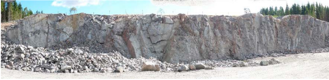
Figure 3-35. Håberg Quarry. Grey, coarse-grained granite gneiss. Steeply-inclined fractures oriented mainly N-S and WNW-ENE.
