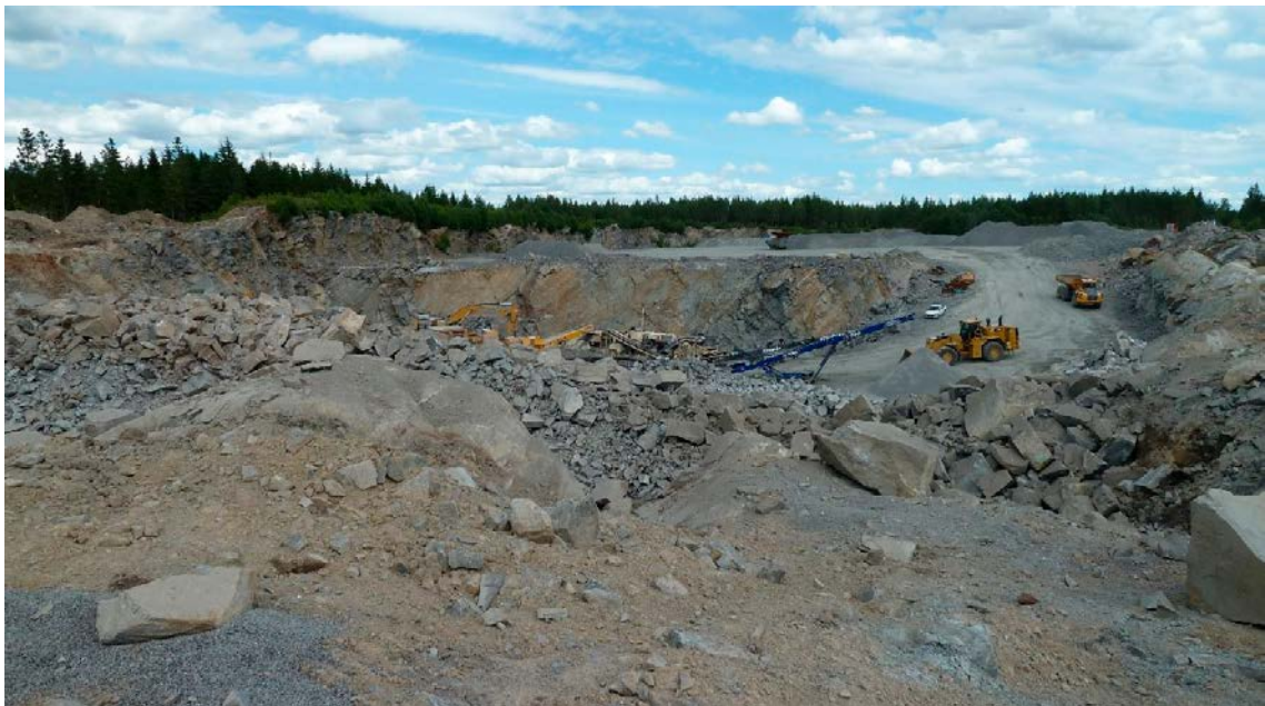
Figure 3-36. Kuleskog Quarry, Vane-Åsaka. Granite gneiss with foliation dipping to NNW. Zones of more widely-spaced fractures form low WSW-ENE trending ridges between shallow, strike-parallel valleys.
