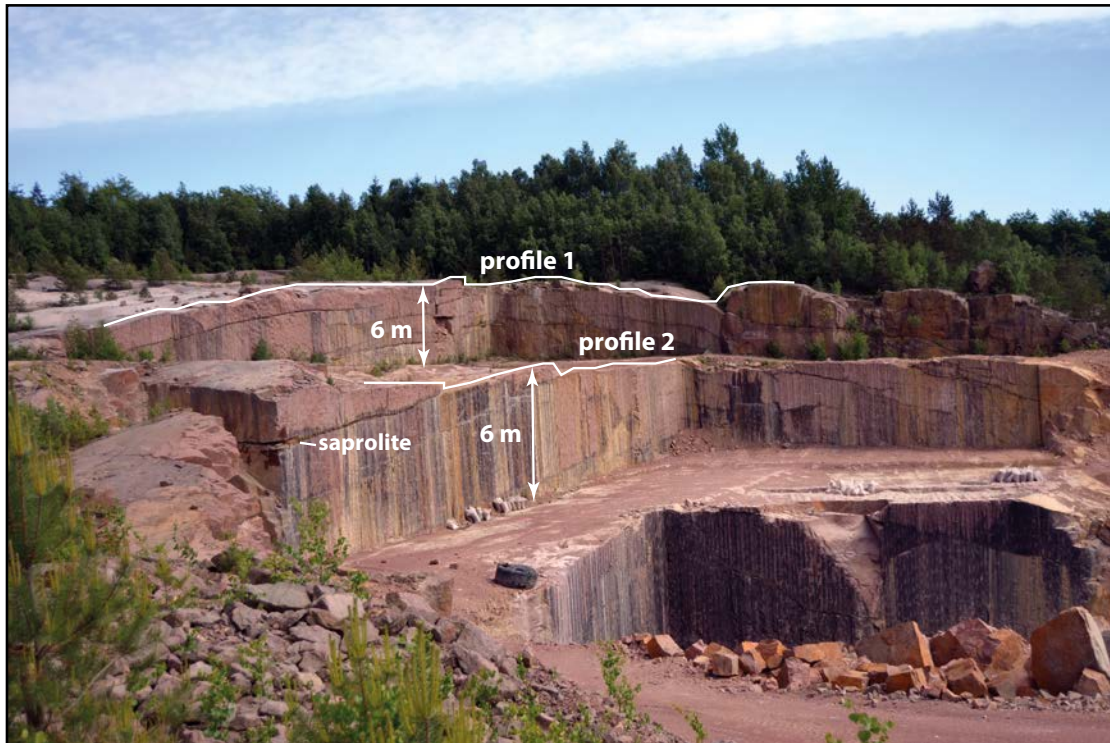
Figure 4-3. Locations of the two GPR profiles at Vånga quarry (cf. Figure 5-1). Well-developed sheeting joints lie subparallel to the ground surface, which is original. The quarry walls to the left in the picture face west, whereas those to the right face North. Both quarry faces are 6 m high. Note the presence of saprolite in a sheeting joint.
