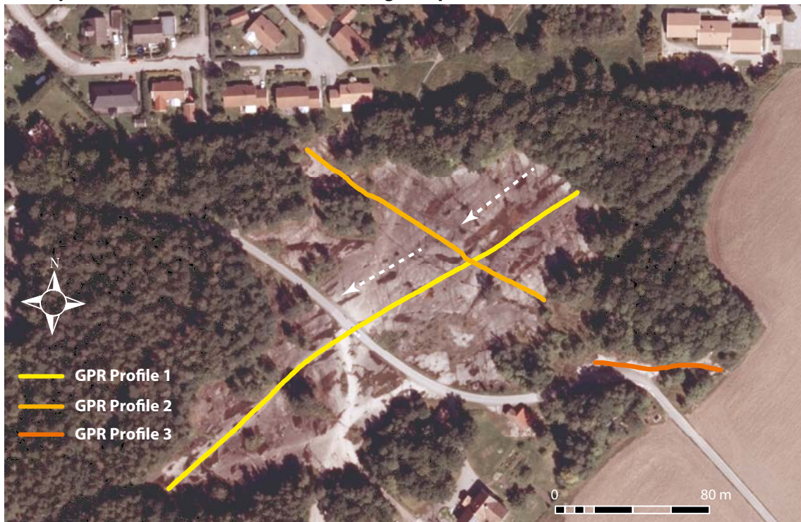
Figure 5-10. Orthorectified aerial photograph showing the locations of three GPR profiles at Sandhem, Trollhättan. Former ice flow direction, inferred from water-filled linear depressions on the outcrop surface, is shown by the white dotted arrows.
