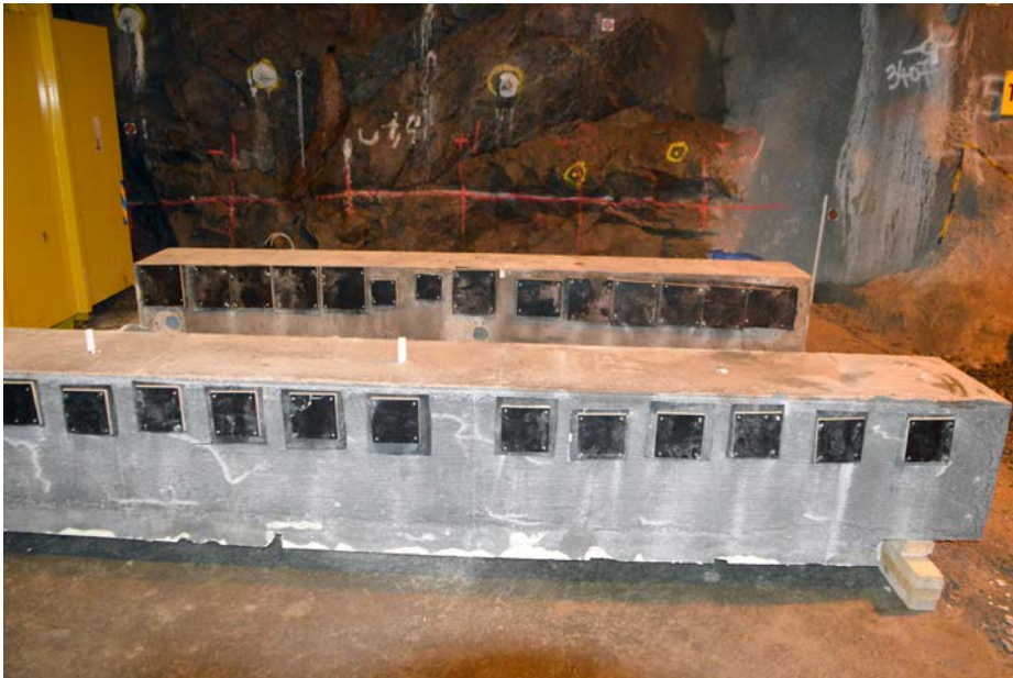
Figure 9-18. The concrete beams used in the grouting tests.
