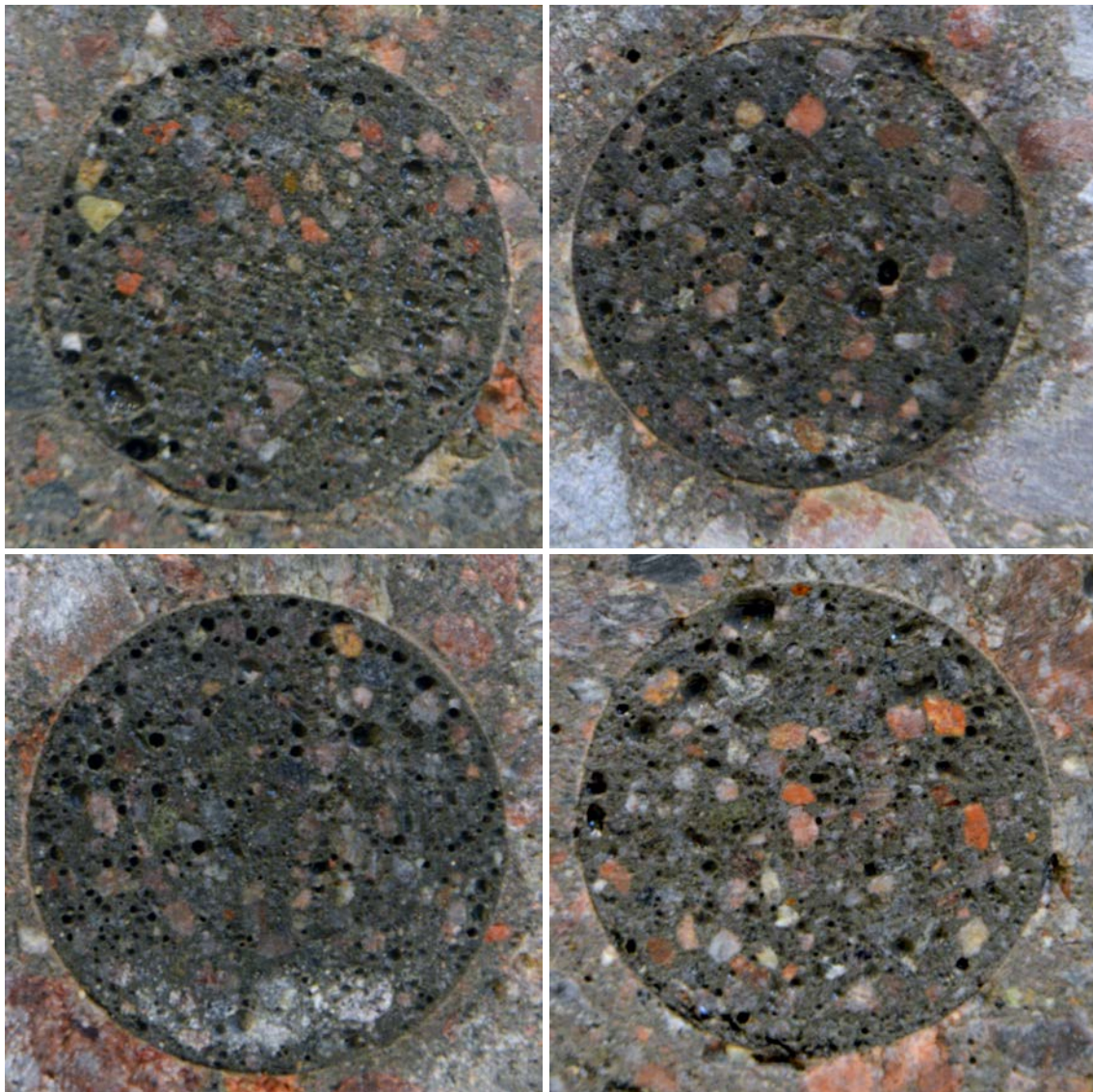
Figure 9-24. Cross sections of some of the cores extracted from the concrete beams used in the production test.
