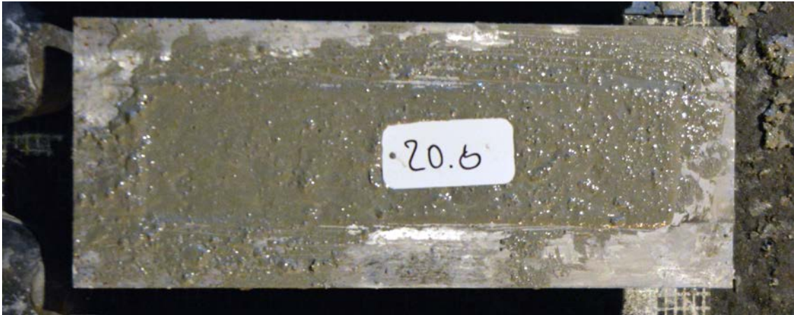
Figure 8-16. A concrete beam for shrinkage measurements made of concrete from transport truck #20.
