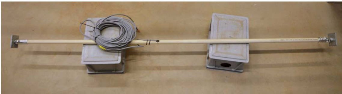
Figure 3-3. Manufactured strain transducer.
