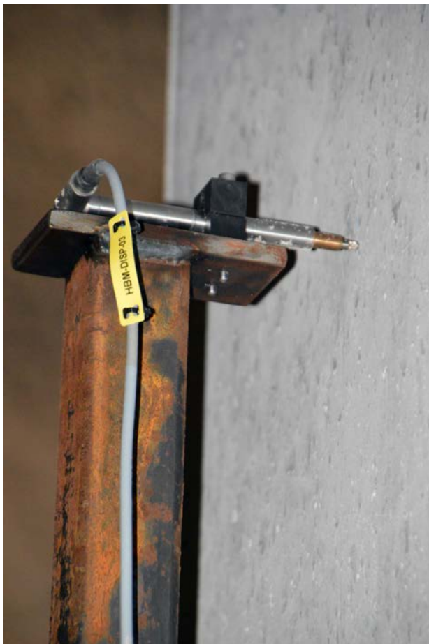
Figure 8-6. LVDT-sensor mounted against the top part of the wall.
