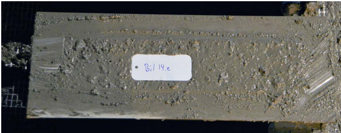
Figure 7-21. Concrete beam for shrinkage measurements made in connection with casting.
