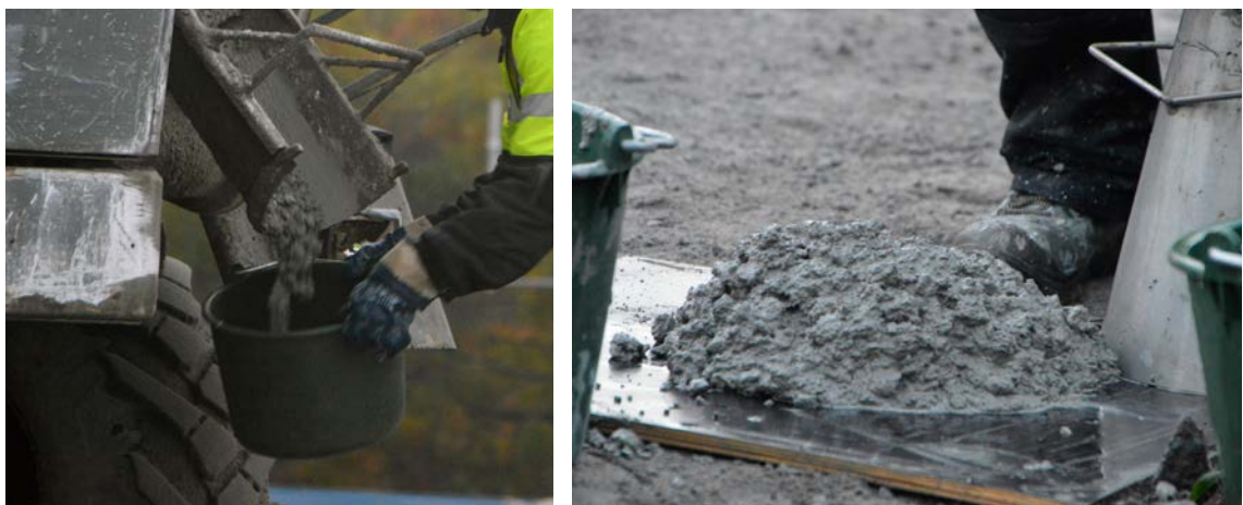
Figure 5-13. Concrete sampling and slump measurement.
