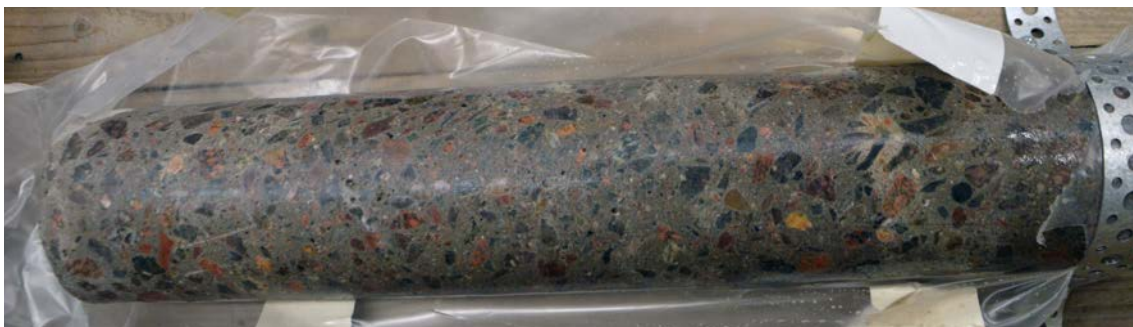
Figure 6-9. An overview picture showing one of the cores. The core is 500 mm long and 100 mm in diameter.
