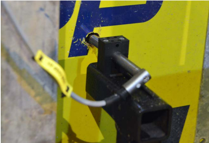
Figure 7-6. LVDT mounted through the formwork against the base slab.
