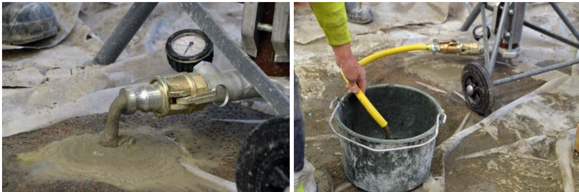
Figure 9-17. Pumping of Bemix A3 without and with a short hose.
