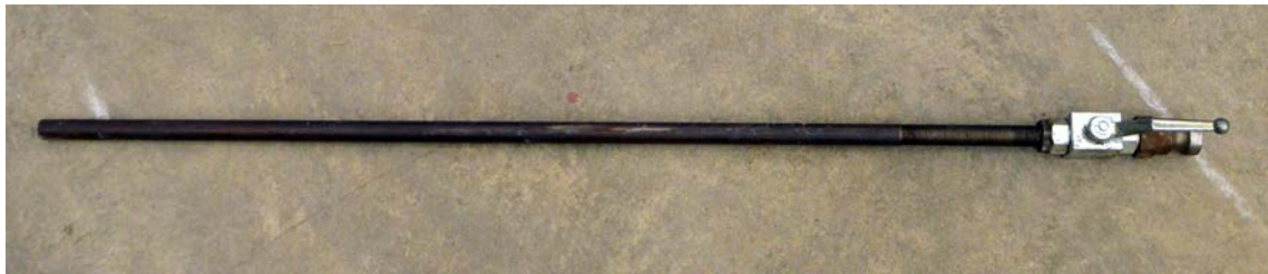
Figure 9-16. The steel pipe aimed for use during grouting.
