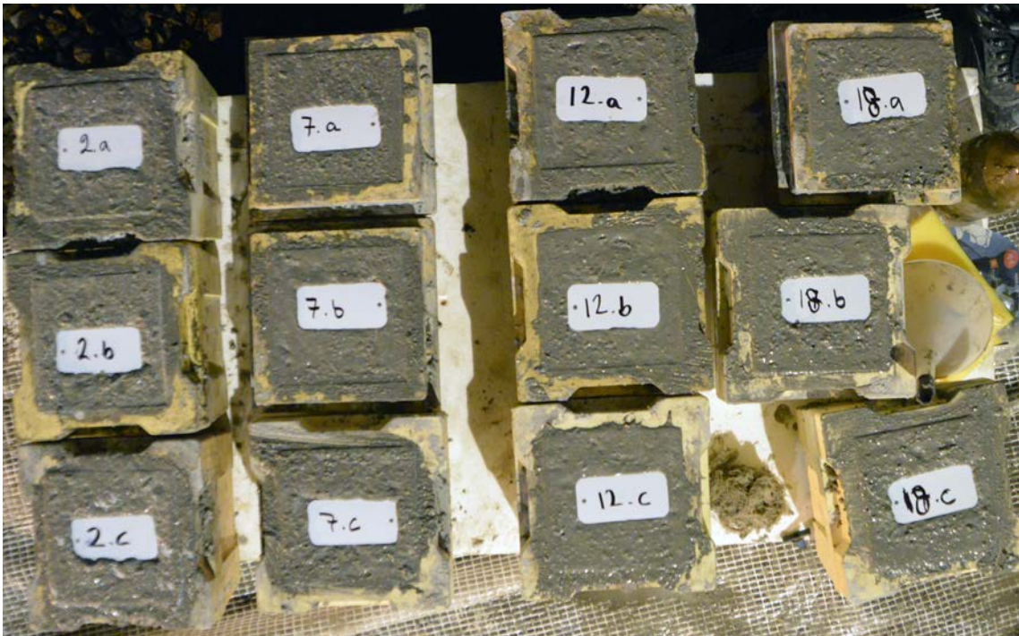
Figure 8-7. Specimens for control of compressive strength.
