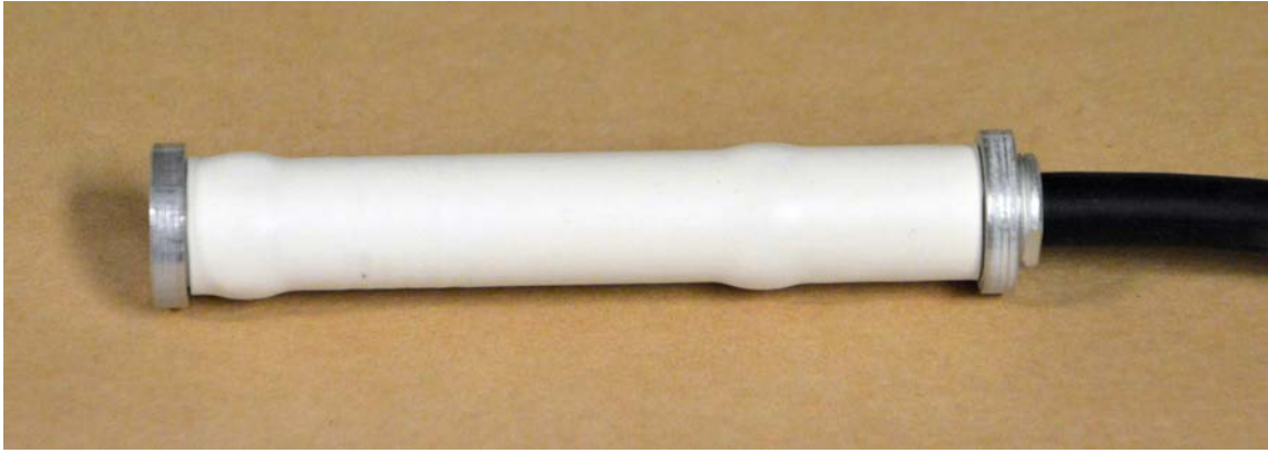
Figure 3-2. Strain gauge transducer.
