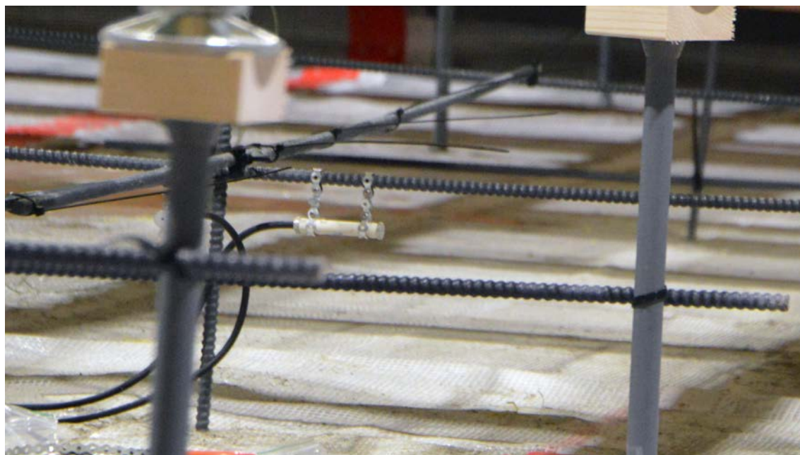
Figure 7-5. A short strain transducer mounted between 2 of the rods that were used to support the footbridge of the working platform.
