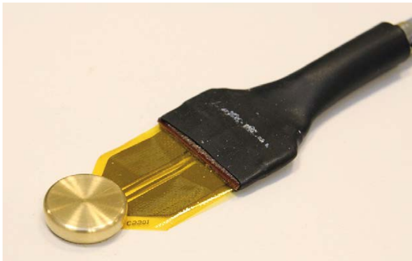
Figure 6-7. Picture of the sensor used for specific heat measurement.
