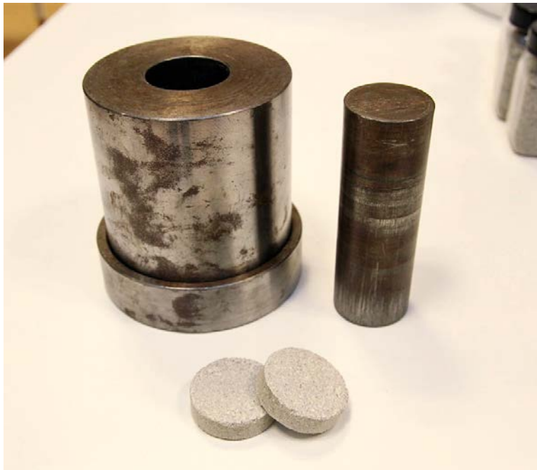
Figure 6-9. The mould and a bentonite sample after compaction.
