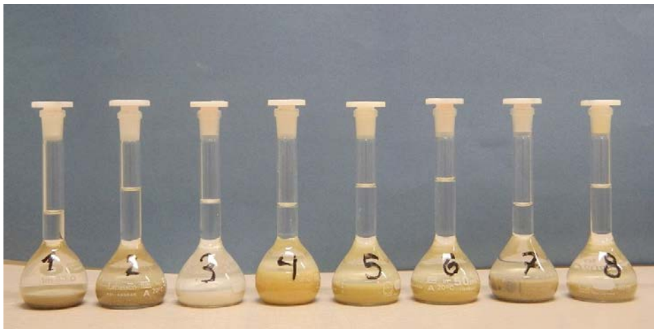
Figure 6-22. Volumetric flasks were the grain density is being determined.
