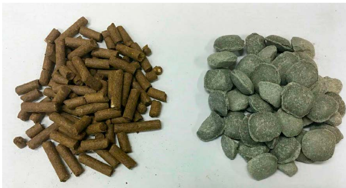
Figure 2-1. Extruded pellets made of Asha material to the left and roller compacted pellets from MX80 to the right.
