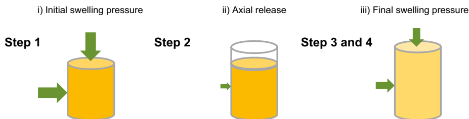
Figure 5-7. Schematic outline of four steps in the one-element analysis.
