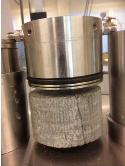
Figure A3-2. Photo of the specimen, suspended in the upper piston, before mounting into the test device.
