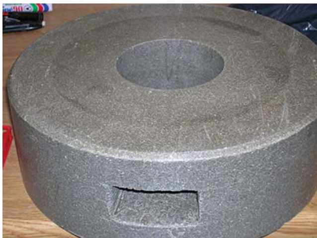
Figure A6-1. Photo of cylinder ring with cavity used for test SH1.
