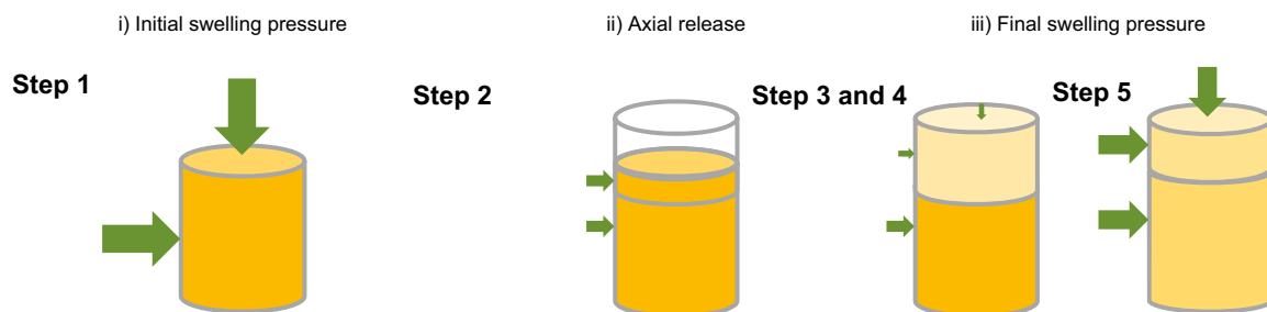
Figure 5-12. Schematic outline of five steps in the two-element analysis.
