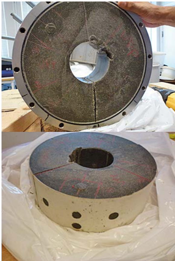
Figure A6-4. Photos of the bentonite ring after dismantling of SH1. The bentonite ring, still inside the steel device but without the inner steel ring, sawn radially and with the sampling marked on the upper surface (to the left) and the dismantled bentonite ring with the filter still left on the outer surface and the sampling marked on the bottom surface (to the right).
