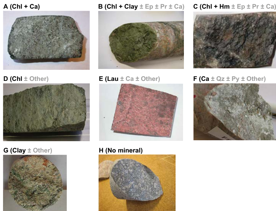
Figure 4-3. Typical fracture surfaces of Forsmark drill core samples. Photos reproduced from Byegård et al. (2008, Table 2-3). Mineral abbreviations are: chlorite (Chl), calcite (Ca), epidote (Ep), hematite (Hm), laumontite (Lau), prehnite (Pr), pyrite (Py), quartz (Qz).
