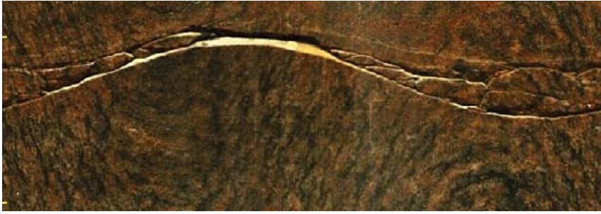
Figure 5-3. OPTV-image of the only crushed interval in KFM25 at 66.54 m.
