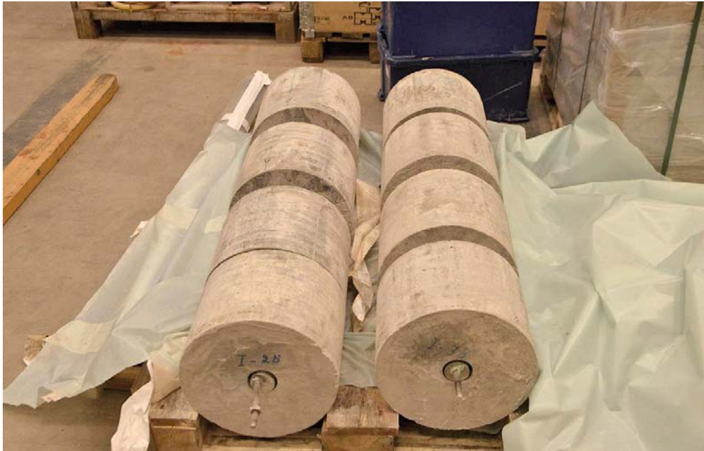
Figure 2-6. The concrete cylinders after sectioning.
