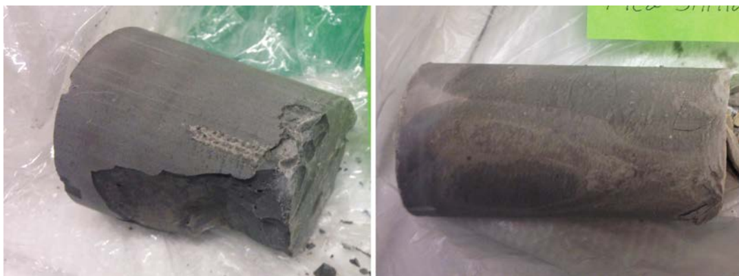
Figure A-1. The cement core without silica (left) and with silica (right).
