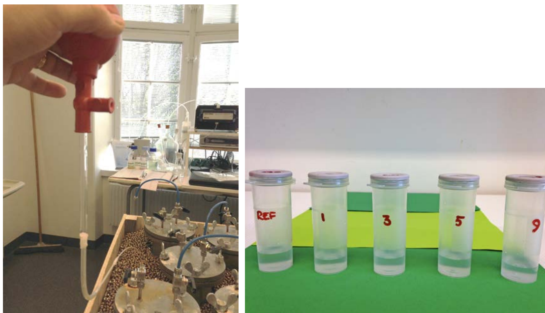
Figure 3-1. Sampling of the steel containers (left image) and water samples from the steel containers (right image).
