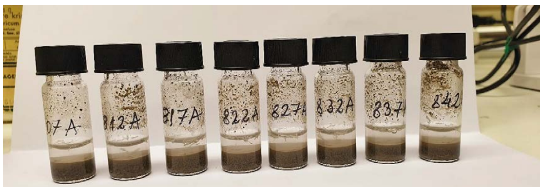
Figure 3-3. Samples in of deuterium-oxide before ultrasonification.
