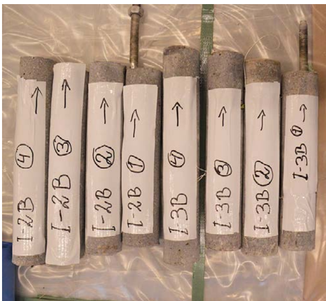
Figure 2-7. Drill cores from the different parts of the concrete cylinders containing different types of material specimens.
