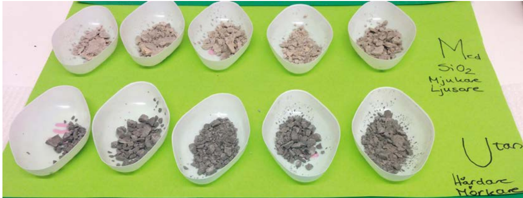
Figure A-2. Samples from the cement cores. The closest specimens are made from standard cement paste while the upper specimens are made from cement blended with \text{SiO}_2 .
