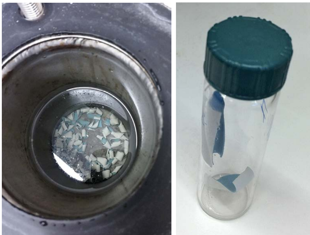
Figure 3-2. Top view of container # 3 and the rubber pieces taken for solid state NMR measurements.
