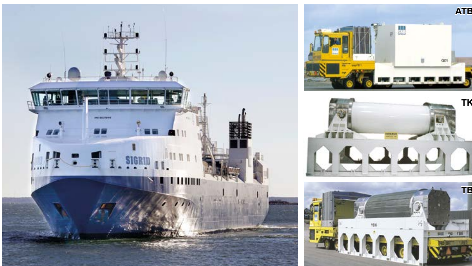
Figure 2-9. M/S Sigrid and the transport casks for short-lived radioactive waste (ATB), for core components (TK) and spent fuel assemblies (TB).
