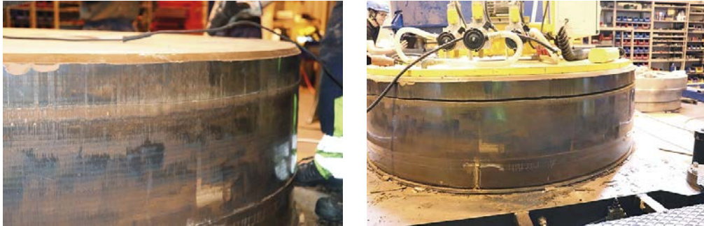
Figure 5-3. A block compacted with the bentonite India 2018.
