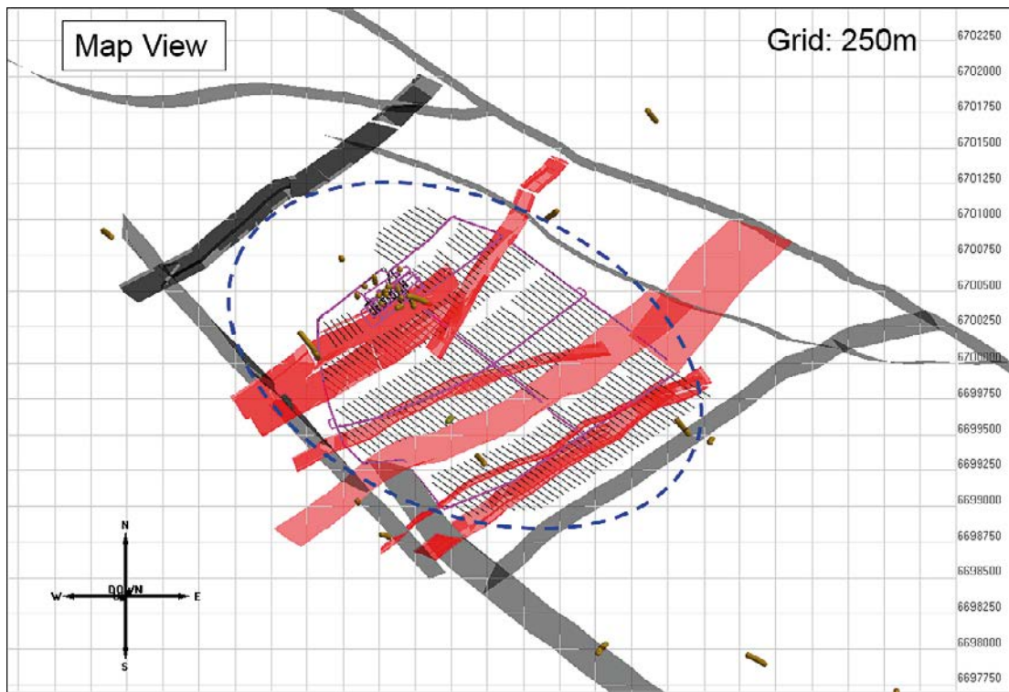
Figure 2-2. Simplified view of vertical (or near vertical) fractures over the proposed repository location. The ideal placement of sensors to avoid attenuation and increasing signal complexity is within the area outlined by the dashed blue line. Red fractures represent those which are most likely to impact microseismic monitoring. Boreholes available for sensor placement indicated in gold.
