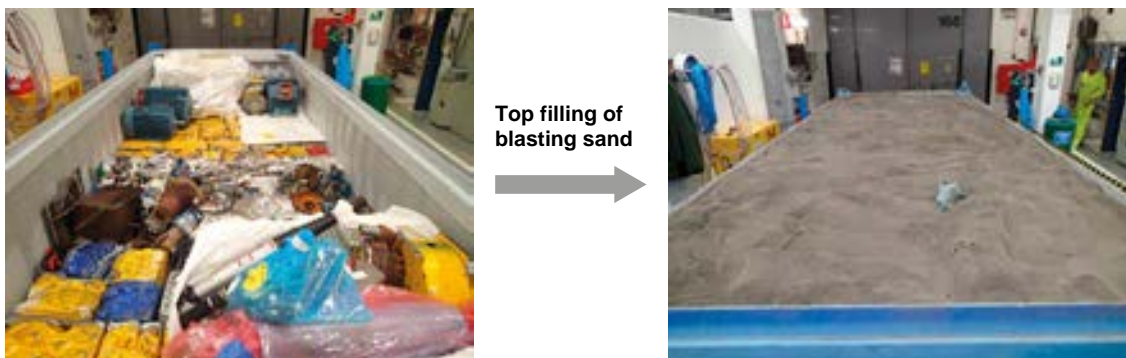
Figure 3-3. Left: metal fraction to a near-surface repository packed in a half-height ISO container; right: top filling of blasting sand to utilise the volume and minimise the void (fitting of lids is done before deposition).
