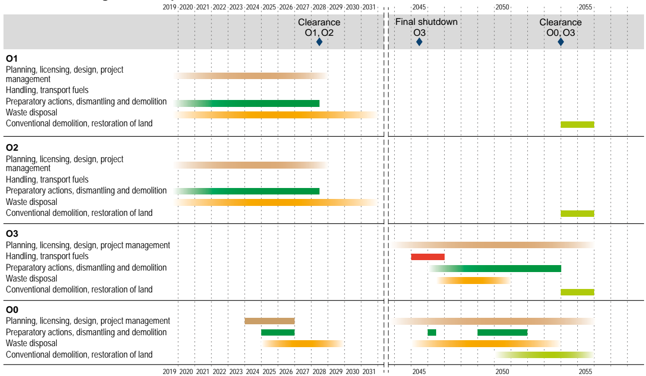
Figure 16-4. Schematic overview of OKG's timeplan for decommissioning (O0 are common facilities that are described separately).
