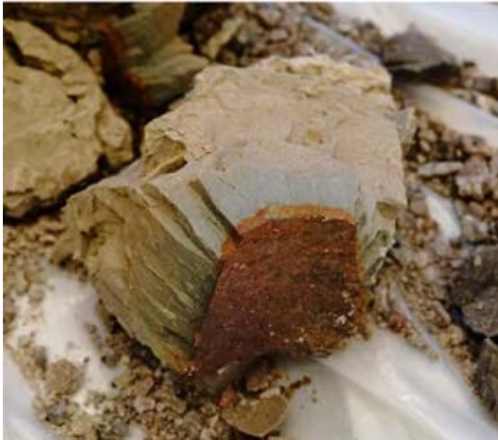
Figure II-13. Sample of Calcigel bentonite from ABM's test package 5, which was retrieved in 2017.
