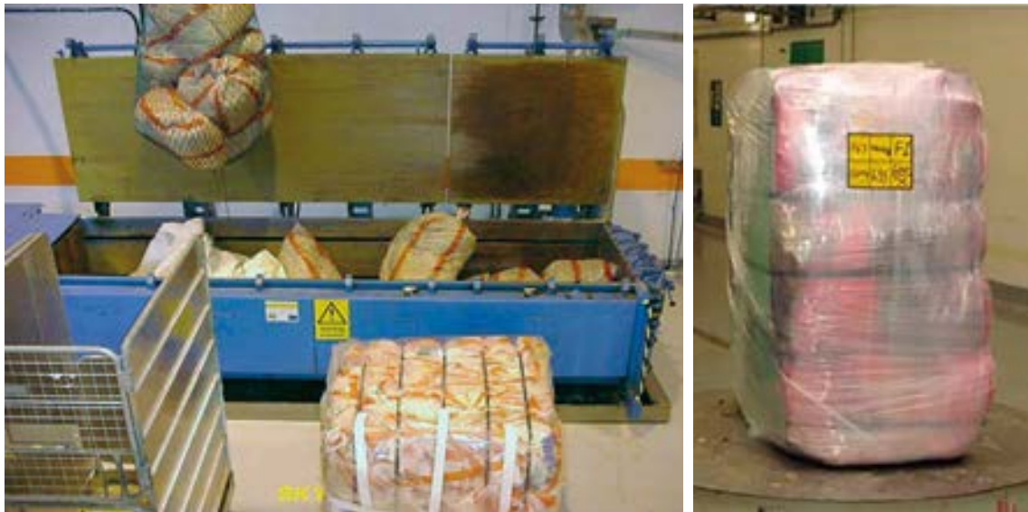
Figure 3-4. Left: bale press for compaction of soft waste; right: compacted waste bale.
