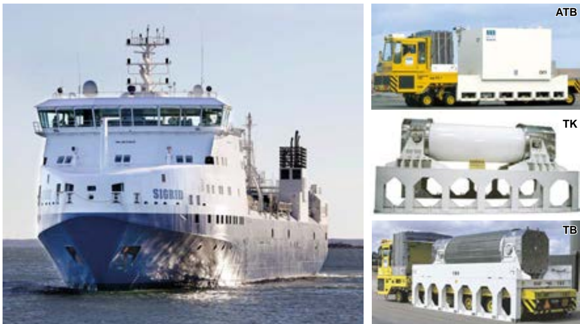
Figure 2-10. M/s Sigrid and current transport casks for short-lived radioactive waste (ATB), for core components (TK) and spent fuel assemblies (TB).
