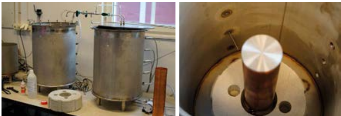
Figure 11-2. Left: Two stainless steel containers equipped with sensors for temperature and relative humidity and connections for online analysis of gas composition. Right: A central heated copper heater with exchangeable copper shields for easy installation and analysis.
