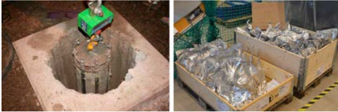
Figure 10-1. Retrieval of a package of 30 bentonite blocks (left-hand picture). Each block also contains four small material samples, which is why the blocks are sorted into four parts and vacuum-packaged before analysis (right-hand picture).
