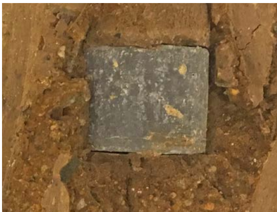
Figure 6-3. Image of a cylinder made of standard cement paste that has been in contact with Asha bentonite. Specimen FXM000778 (Fe).
