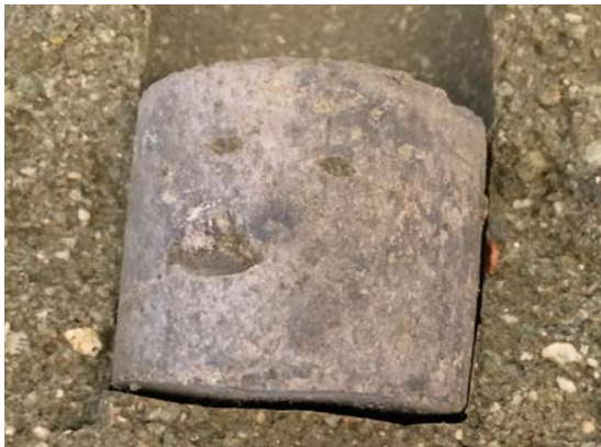
Figure 6-21. Image of a cylinder made of low-pH cement paste that has been in contact with Ibeco RWC bentonite. Specimen FXM000736 (Mo).
