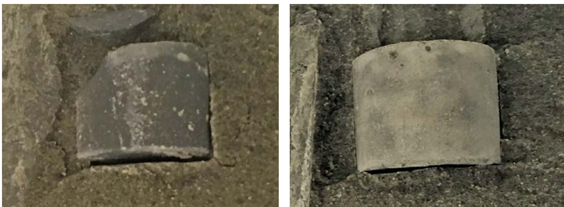
Figure 6-28. Images of cylinders made of low-pH cement paste that have been in contact with MX-80 bentonite. Specimen FXM000766 (left, Fe) and FXM000768 (right, Mo).
