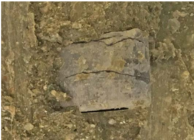
Figure 6-14. Image of a cylinder made of low-pH cement paste that has been in contact with Febex bentonite. Specimen FXM000708 (Mo).
