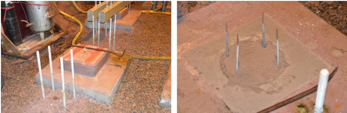
Figure 2-1. The beams have been removed and the lid is lifted. The tubes protruding from the sand provided water for saturation of the bentonite.
