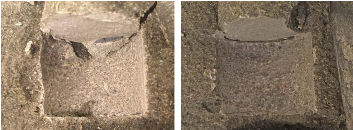
Figure 6-27. Images of the bentonite at the position where specimens of low-pH cement paste have been placed. Specimen FXM000766 (left, Fe) and FXM000768 (right, Mo).
