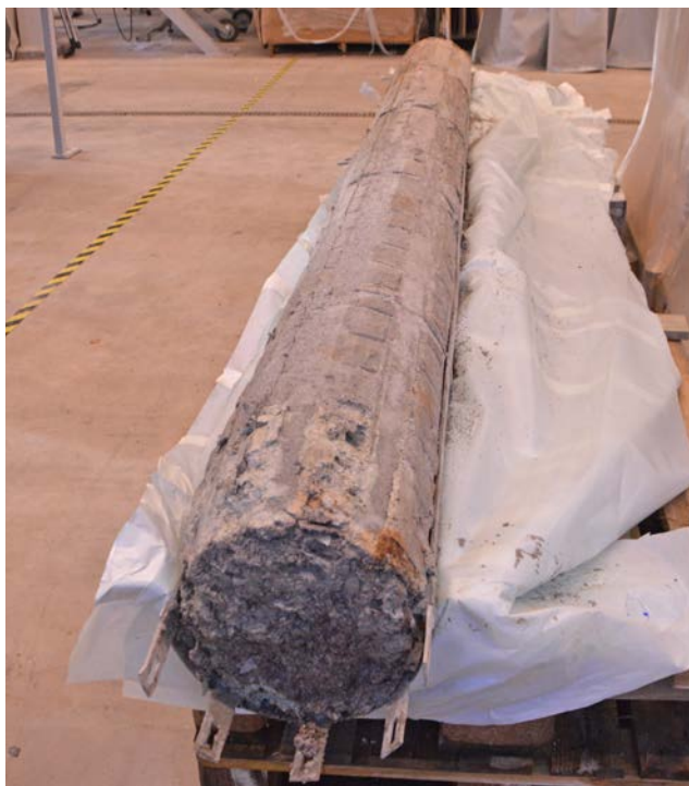
Figure 3-1. The plastic sheet has been removed from the package and the titanium cage cut in half.
