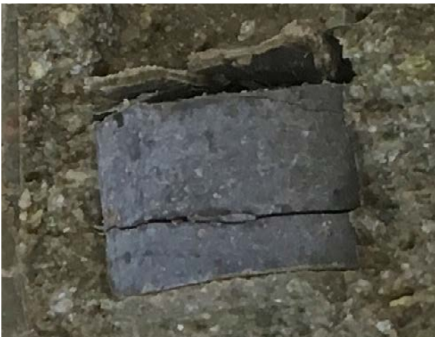
Figure 6-10. Image of a cylinder made of standard cement paste that has been in contact with Febex bentonite. Specimen FXM000697 (SrCl 2 ).
