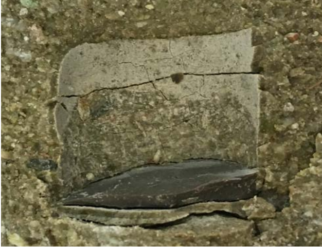
Figure 6-9. Image of the bentonite (Febex) at the position where a specimen of standard cement paste has been placed. Specimen FXM000697 (SrCl 2 ).
