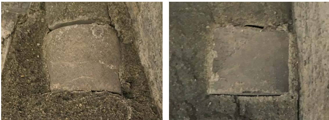
Figure 6-24. Images of cylinders made of standard cement paste that have been in contact with MX-80 bentonite. Specimen FXM000745 (left, Fe) and FXM000761 (right, \text{EuCl}_3 ).
