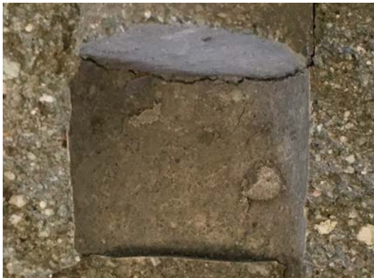
Figure 6-20. Image of the bentonite at the position where a specimen of low-pH cement paste has been placed. Specimen FXM000736 (Mo).
