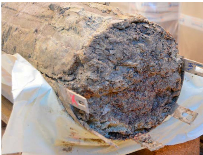
Figure 3-2. The top part of the package showing how the top blocks have coalesced into a structure with the resemblance of mud rather than clearly distinguishable separate blocks.
