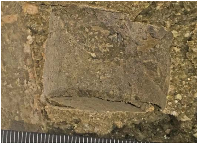
Figure 6-13. Image of the bentonite (Febex) at the position where a specimen of low-pH cement paste has been placed. Specimen FXM000708 (Mo).
