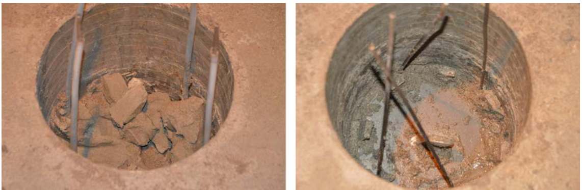
Figure 2-2. The bentonite on top of the experiment package is removed and the lid is exposed.
