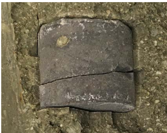
Figure 6-17. Image of a cylinder made of standard cement paste that has been in contact with Ibeco RWC bentonite. Specimen FXM000714 (Fe).
