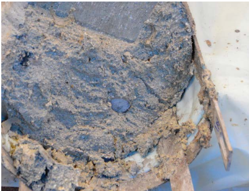
Figure 3-3. Test cut in the top dummy block showing the unexpected presence of a cement specimen in the middle of the image.
