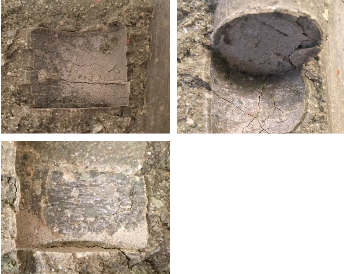
Figure 6-16. Images of Ibeco RWC bentonite at the position where specimens of standard cement paste have been placed. Specimen FXM000714 (top left, Fe), FXM000725 (top right SrCl 2 ) and FXM000732 (lower left, CsCl).
