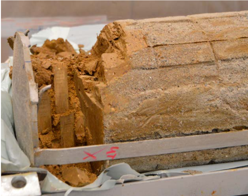
Figure 3-4. Removal of the 3 dummy blocks at the bottom of the package. Note how the bentonite swelling pressure has made the thick titanium bottom plate convex. Here the joints between the different blocks are clearly visible.
