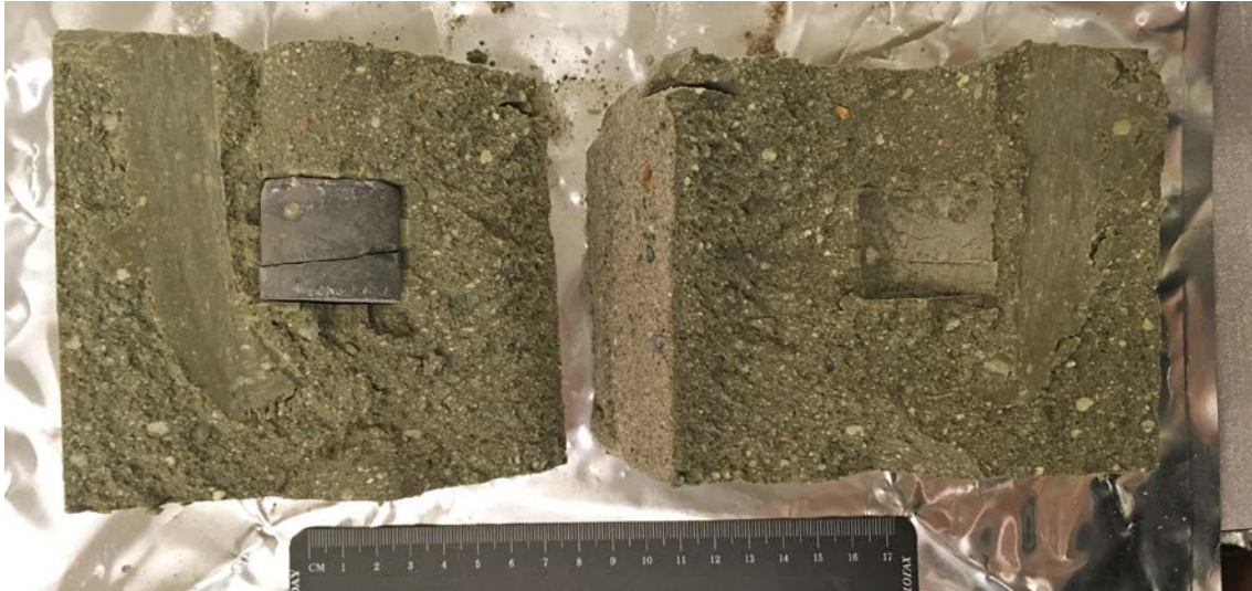
Figure 4-1. Chopping of the bentonite block exposed the cement/bentonite interface
