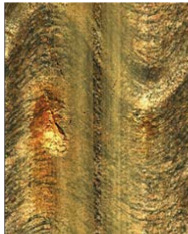
Figure 6-2. a) Excerpt from the log result of the acoustic televiewer. The small breakout at 399.4–399.5 m depth is clearly seen in both the “Amplitude” and “Caliper” columns. The left border of the images corresponds to the bearing of the borehole. The central points of the breaks are located opposite each other in a direction, at 90 and 270 degrees from the bearing direction. Below the breakout in the same direction some darker dots in the “Amplitude” log can also be noted, indicating small starting “Micro fallout”. b) The same location of KFM24 in the optical log (OPTV). The OPTV log (Lundgren 2017) gives the colours of the rock of the borehole wall. It can be noted that the rock seems reddish in the area of the breakout. This example also illustrates why acoustic televiewer is needed to clearly identify breakouts, and other small geometrical variations, in the borehole wall.
