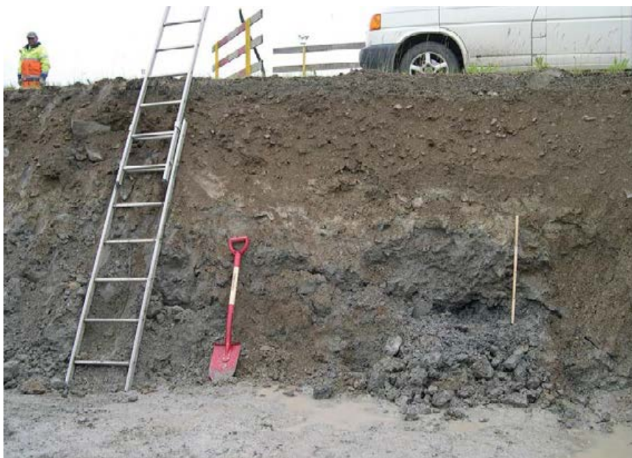
Figure 2-4. Photograph of artificial-fill profile in a trench (Figure 5-25 in Hedenström and Sohlenius 2008).
