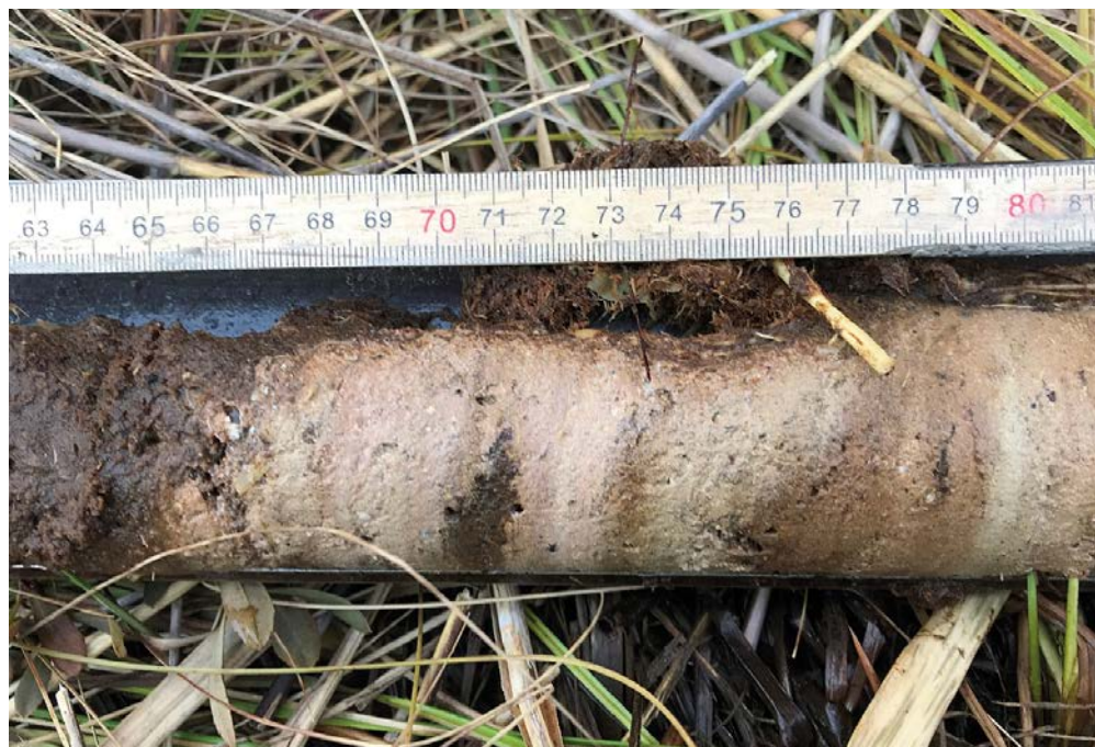
Figure 4-7. Calcareous gyttja sampled in the peat covered wetlands surrounding Lake Gunnarsboträsket. The gyttja contain a high frequency of shells (PFM008042). The same type of gyttja was found at the floor of the lake and have also been recorded in many other lakes in the area and a calcium carbonate content as high as 63 % has been recorded (Hedenström 2004).
