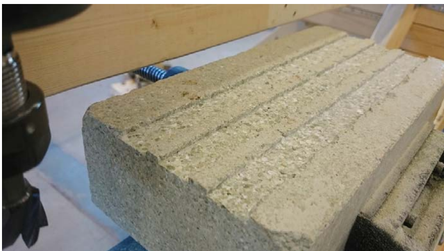
Figure 4-2. Milled track in bentonite with the linear motor.
