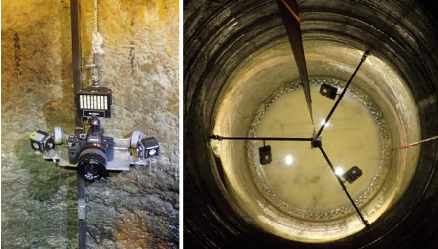
Figure 3-10. Tests of setups and rigs for photography of deposition holes. To the left: Adjustable camera cradle with attached lightning. To the right: Rig with attached lightning used for photography with a spherical iSTAR camera from NCTech.
