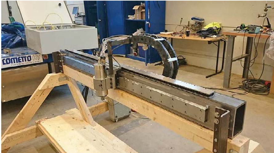
Figure 4-1. Test rig for the linear motor and the motor spindle.
