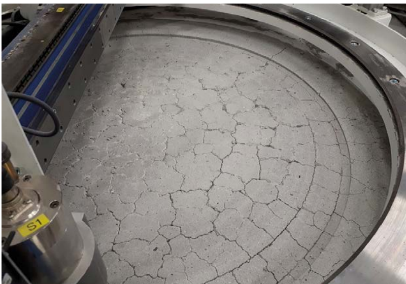
Figure 4-5. Milling the surface levelled on which the canister stands.
