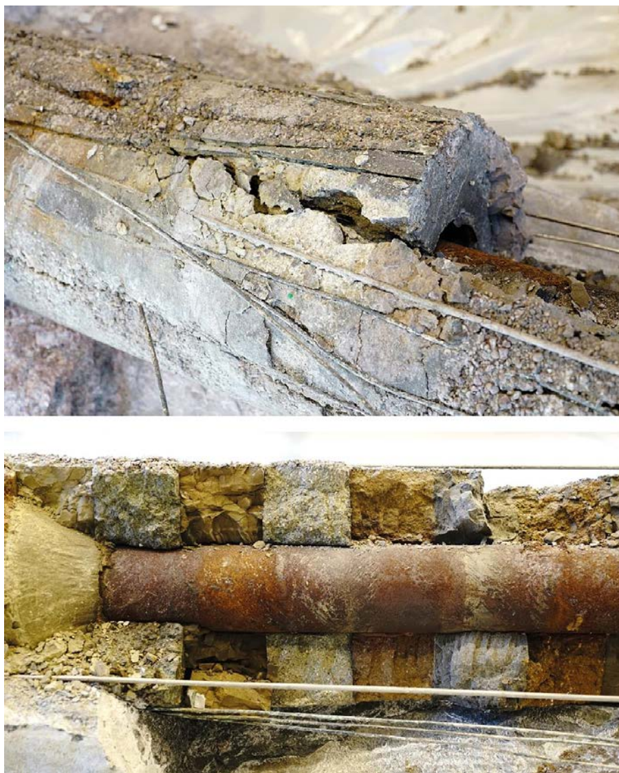
Figure 3-30. Highly fractured bentonite blocks from the very high temperature experiment ABM5 excavated in 2017.
