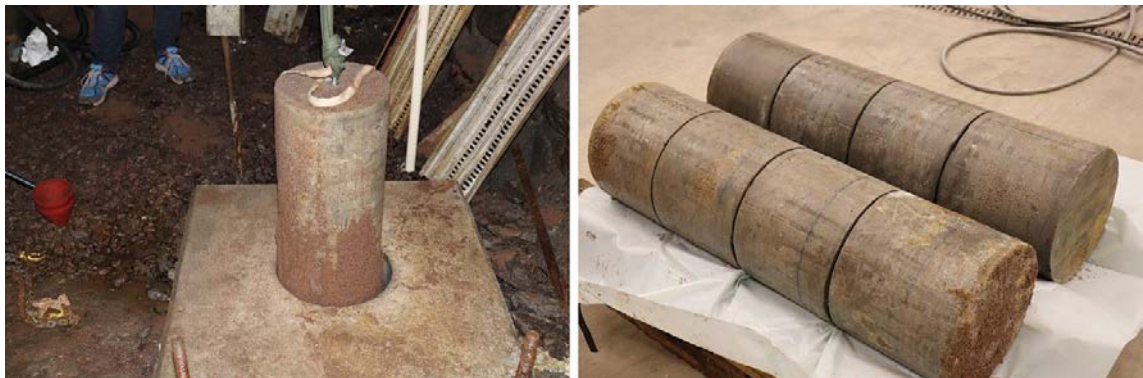
Figure 3-28. Retrieval and segmenting of the concrete cylinders.
