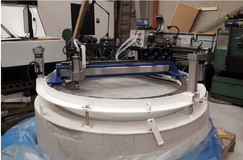
Figure 4-3. The prototype fully assembled and ready for milling test.
