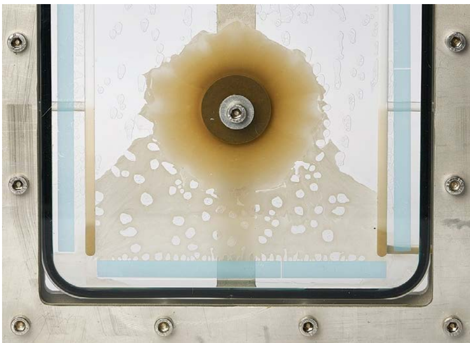
Figure 5-2. Experimental cell for measuring of chemical erosion of swelling clays. In this case the clay used is dialysed Nanocore at very low ionic strength in a 0.2 mm vertical fracture. The vertical placement show the impact from gravity on the sedimentation.
