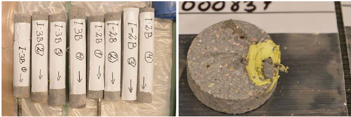
Figure 3-29. Cores from the segments of the concrete cylinders and a segment of the core containing a piece of organic material.
