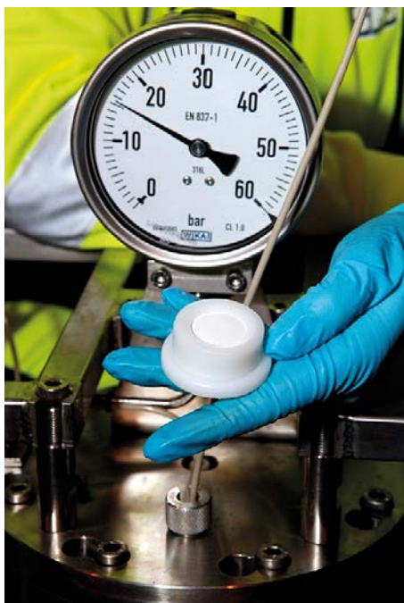
Figure 2-3. The simple and robust DGT device is deployed for a known time in deep groundwater and provides the time weighted average concentration for the REEs.
