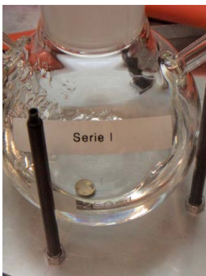
Figure 2-1. Leaching of unirradiated AIC alloy.
