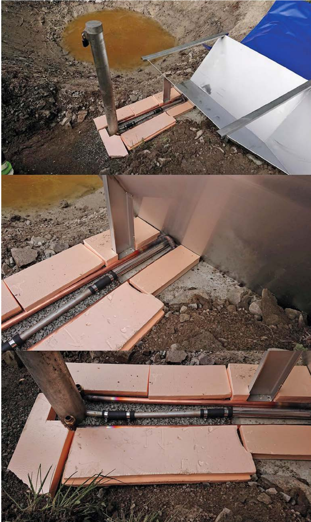
Figure 2-4. The pipe connecting the flume to the observation well, and close ups of the insulation and copper pipe for heating, looped around the connection pipe.
