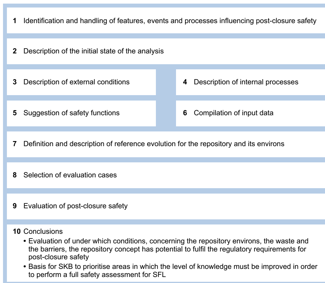
Figure S-2. Overview of the methodology applied for the evaluation of post-closure safety for the proposed repository concept for SFL.
