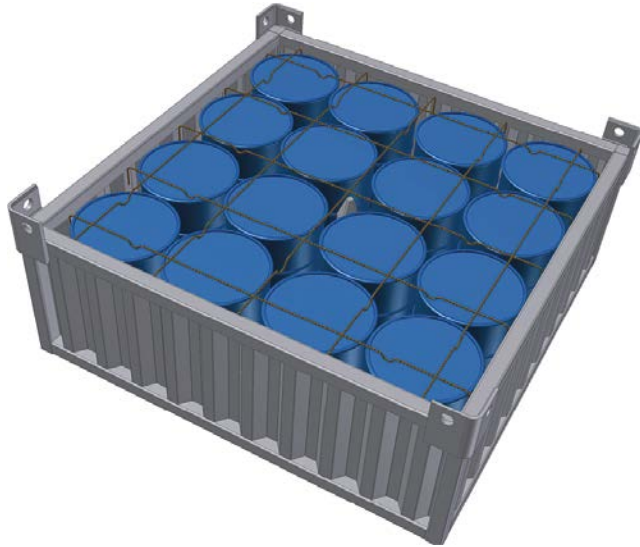
Figure 3-5. 3D-view of a waste packaging loaded with four trays with four drums each. Reinforcement bars that will stabilise the future grout on top of the drums are also shown.
