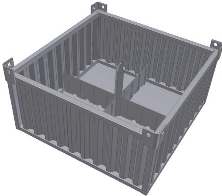
Figure 3-2. 3D-view of a waste packaging for standard moulds when empty. The stiffening plates for the bottom plate and guides for the moulds are visible.
