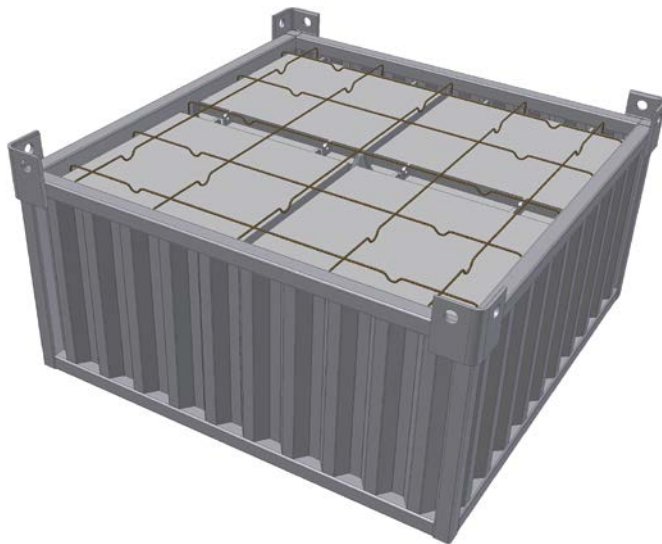
Figure 3-3. 3D-view of a waste packaging loaded with standard moulds. Reinforcement bars that will stabilise the future grout on top of the moulds are also shown.
