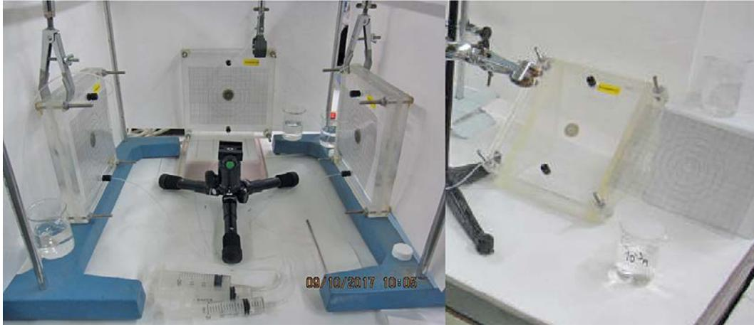
**Figure 3-6.** Photographs of sedimentation tests carried out at: (left) 90° slope and (right) 45° slope.
