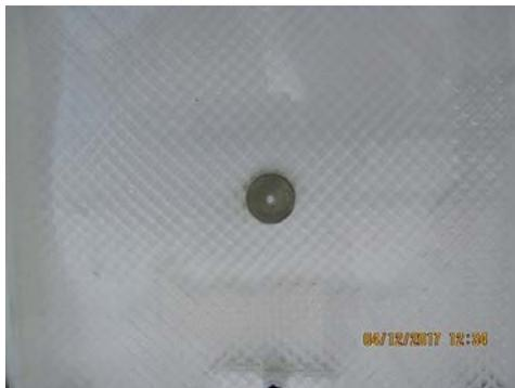
**Figure 3-2.** Photography of a rough fracture, including a methacrylate plate with well-defined rough pattern (clay pellet diameter is 19 mm).
