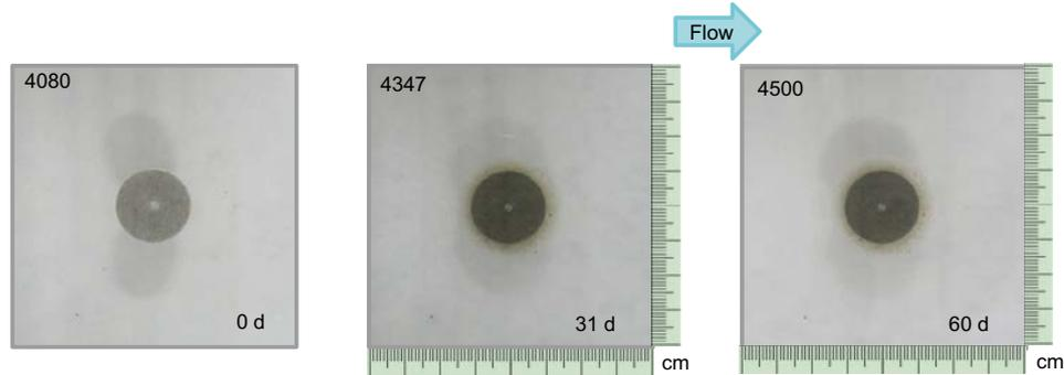
Test 13A: RawMX-80 1.4 g·cm<sup>-3</sup> - Slope 0° - Aperture 0.2 mm - NaCl 10<sup>-3</sup> M
