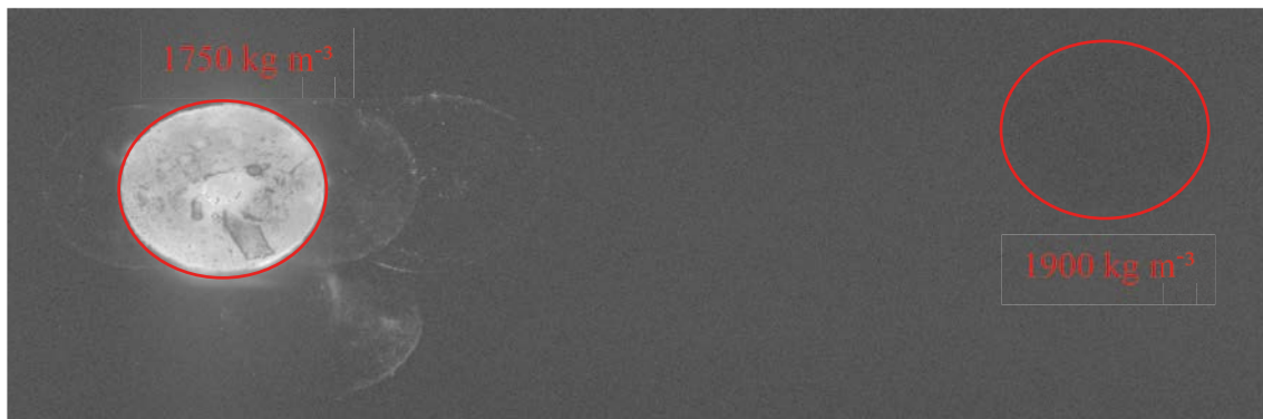
Figure 3-3. Phosphor plate exposed to the copper discs used in the pressure cells. A lighter colour indicates a greater exposure to radiation from S-35.
