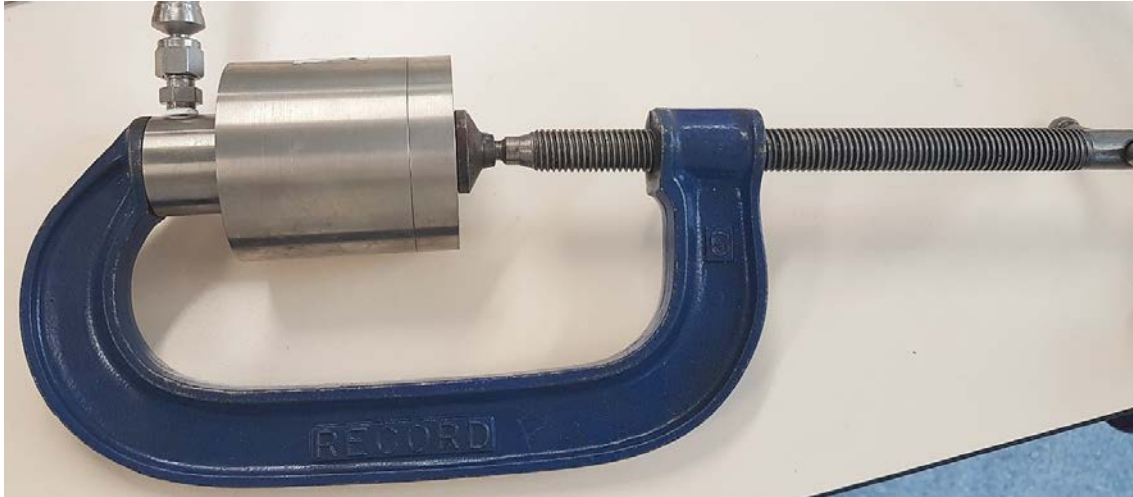
Figure 2-1. Use of a G-clamp to compact the bentonite inside of the pressure cells. The tightening of the screw pushes the piston into the pressure cell reducing the volume to that required for the experiment.
