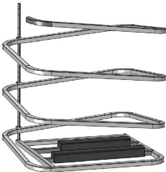
Figure 1-1. Schematic picture of SFL repository design with the BHA vault (front) and the BHK vault (back).
