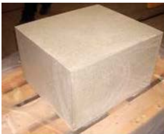
Figure 2-1. Left: Photo of a bentonite block that was used for the sealing section. Right: Schematic drawing of the block stack for the bentonite seal.
