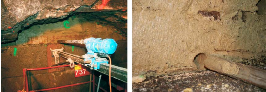
Figure 4-20. Left: The central parts of the backfill were sampled using a core drill. Right: The outermost parts, close to the rock wall were sampled with a special made “half pipe”.
