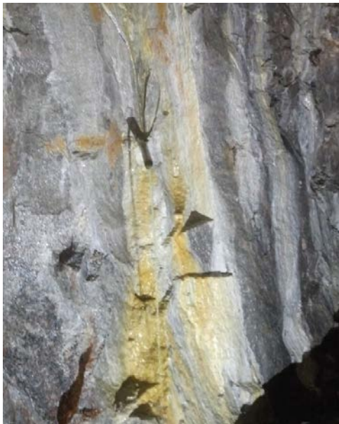
Figure 2-10. Photo showing the rock fracture where water was collected. A steel tube was glued to the rock surface and the leakage water measured.
