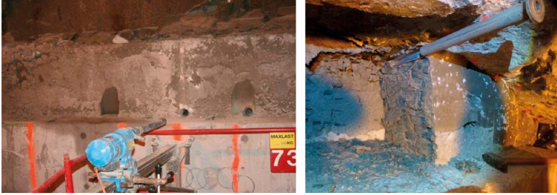
Figure 4-6. Left: The central parts of the bentonite seal were sampled using a core drill. Right: The outermost parts, close to the rock wall were sampled with a special made “half pipe”.
