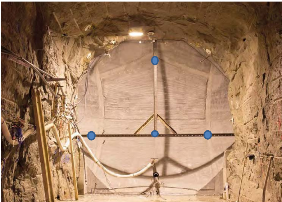
Figure 3-11. Photo showing the approximate position of the four displacement sensors mounted on the dome plug.
