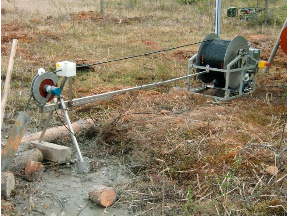
Figure 4-2. Set-up, cable drum with electrical motor for lowering the probe and a measuring wheel for positioning the probe (left).
