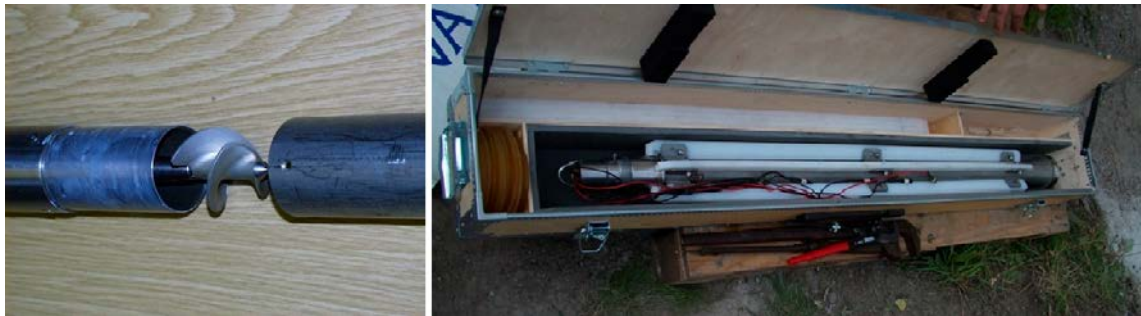
Figure 4-1. The spinner used for logging of the flow (left) and probe with plastic guides (right). A rubber disk at the end of the probe can be changed for different diameters of the borehole (left in the box).
