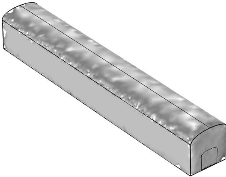
Figure 6-35. Iso-surface of zero portlandite volume fraction in the 3D vault-scale domain after 8 500 years.
